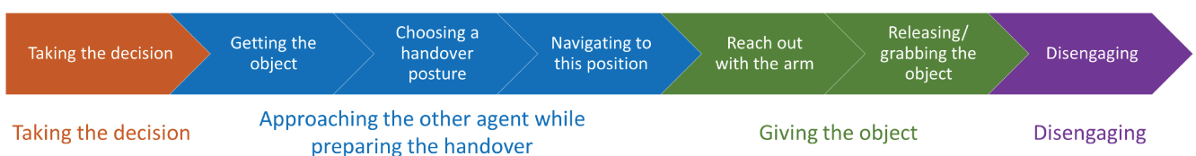
FIGURE 2.1: During a handover, the agents 1 go through four phases, with, in each one, a number of actions to perform. This time-line concern both agents.
