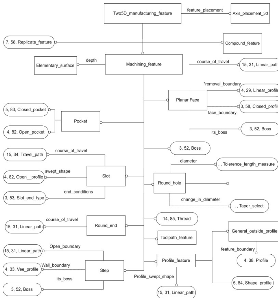
Figure 21 : Ensemble des manufacturing feature 2.5D du standard STEP-NC (Dipper et al., 2011)
