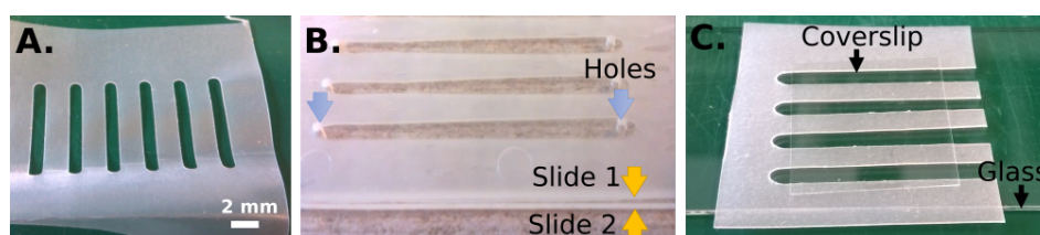
Figure 4.27 – Low-cost fabrication of polystyrene and glass devices. (A) Channels were cut in a parafilm sheet with a plotter cutter. (B) Two of these sheets were embedded between two polystyrene slides aligning the ends of the channels with the drilled holes on slide 1. Then the device was placed on a hot plate at 50°C for 45 s to glue the assembly. (C) A glass slide and a coverslip could be used instead of polystyrene slides. But no holes were drilled. The width of the channels were unevenly deformed upon heating but the height ( \approx 200 \mu\text{m} ) remained constant.
