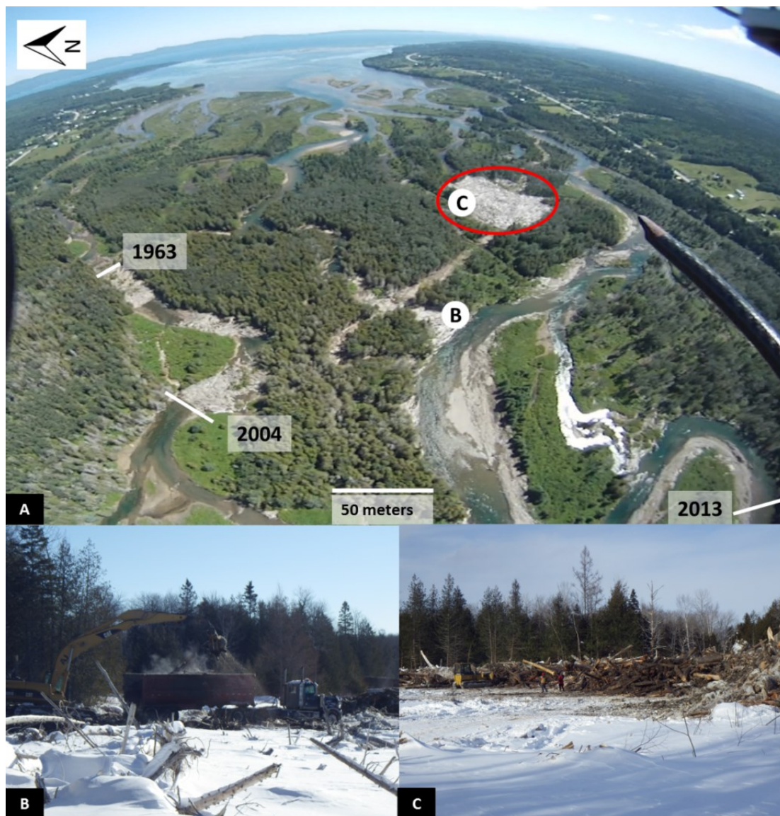
Figure 40. (A) Aerial photography (drone) of the Saint-Jean delta in July 2015, after dismantling of the main large raft in the south channel. (B) Photography during the dismantling in February 2015 and (C) Area of deposited LW from the raft in February 2015. (B) and (C) represent the position where the pictures were taken in (A). *The red circle represents the deposition area of the removed wood of the raft in winter 2015 and line represent limits of the raft in 1963, 2004 and 2013.
