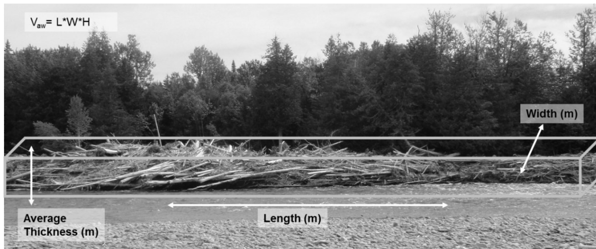
Figure 17. Theoretical examples of the method used to measure the ‘air-wood’ volume of large wood (LW) accumulations. The width ( w ), the average thickness ( h ) and the length ( L ) of a simple rectangular are measured to the nearest centimetre using a rigid and flexible graduated ruler.
