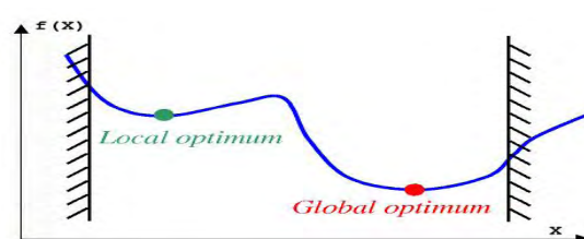
Figure III.8 — Solution optimale locale vs solution optimale globale
