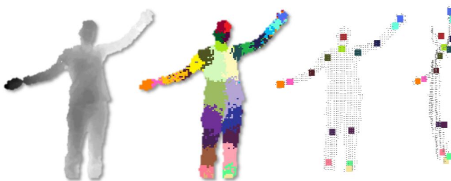
Figure 2.8 – Depth image, corresponding inferred most likely body part labels and joints proposals. Extracted from [SFC + 11].
