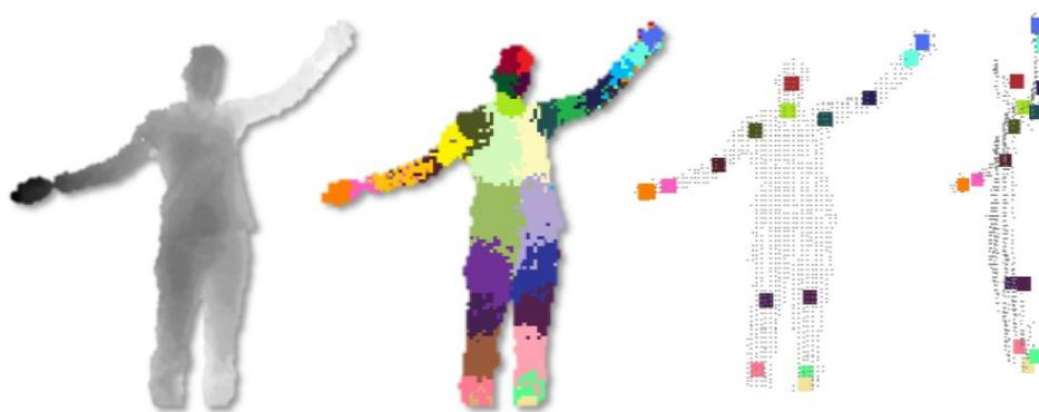
Figure 2.8 – Depth image, corresponding inferred most likely body part labels and joints proposals. Extracted from [SFC<sup>+</sup>11].
