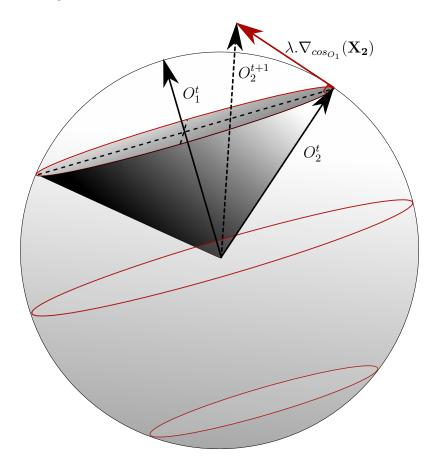
Figure 3.3 – Representation of the effect of an update step on the norm of the projections for a pair of outputs  $(\mathbf{O_1^t}, \mathbf{O_2^t})$  at the epoch t in 3D. The centre of the sphere corresponds to the origin of the output space. The grey cone represents the equipotential surface for the function  $cos_{O_1}$ . For simplification,  $\mathbf{O_1^t}$  and  $\mathbf{O_2^t}$  were given the same norm.
