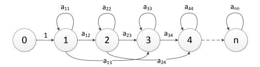
Figure 2.10 – Example of a left-to-right HMM, with two forward connections.
