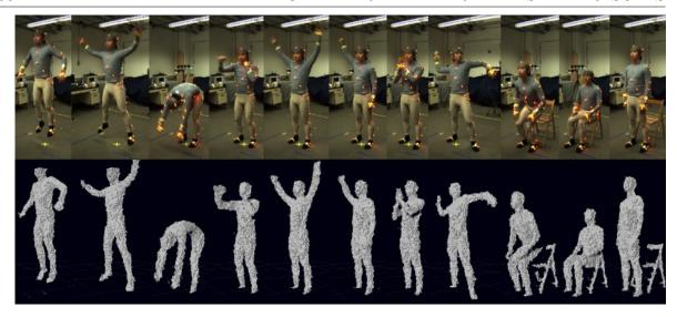
Figure 4.1 – Snapshots from all the actions available in the Berkeley MHAD are displayed together with the corresponding point clouds obtained from the Kinect depth data. Actions (from left to right): jumping, jumping jacks, bending, punching, waving two hands, waving one hand, clapping, throwing, sit down/stand up, sit down, stand up. Extracted from [OCK+13].
