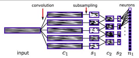
Figure 2.14 – Representation of the architecture and activation maps of a Convolutional Neural Network. Extracted from [DBLG14]. Convolutional layers  $c_i$  are followed by sub-sampling layers  $s_i$ , which allows a progressive dimensionality reduction and feature computation for the last output layer operating the classification.
