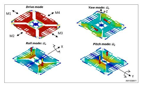
Figure 2.5 – Single driving structure of 3-axis digital gyroscopes. Extracted from [STM].
