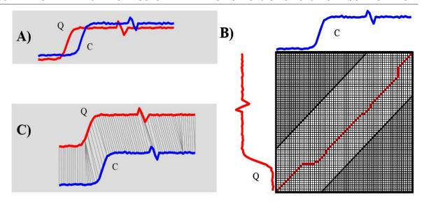
Figure 2.11 – Extracted from [RK04]. Example of DTW computation between two similar, out-of-phase signals Q and C, represented in A. B corresponds to the warping matrix, with the minimum-weight warping path between the two signals. C is the representation of the resulting alignment.
