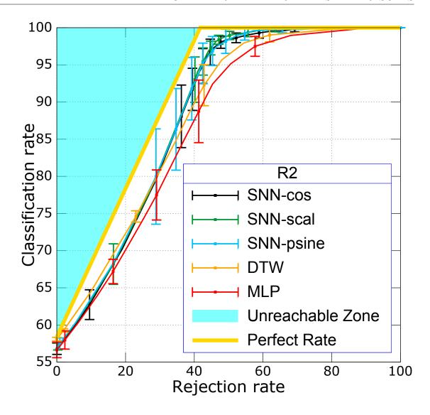
Figure 4.10 – SNN-scal, SNN-psine, DTW and MLP comparison on **R2**.
