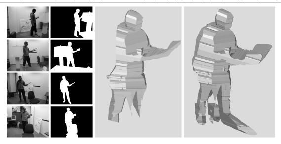
Figure 2.6 – Representation of the visual hull, result of 3D space carving. Extracted from [GSFP06].
