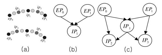
Figure 2.9 – Example of a recursive construction of a primitive model. Gesture primitives, formed by two end-points (EP) which are local extrema for the acceleration signal, are recursively decomposed in inter-primitive points (IP), located at equal distance from their parents). Extracted from [CCB<sup>+</sup>06].
