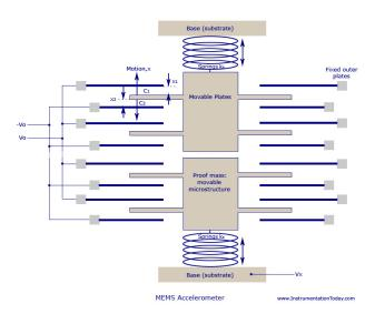
Figure 2.2 – Schematics for a one-dimensional MEMS accelerometer. Extracted from [ins].
