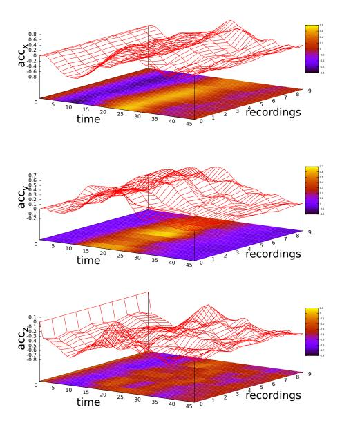
Figure C.2 – Accelerometer signals for 10 recordings of the "Flick East" gesture for one user after preprocess.
