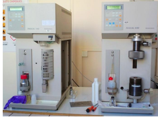
Figure 2.17: Mercury porosimetry equipment of “Pascal 140” and “Pascal 440”.
