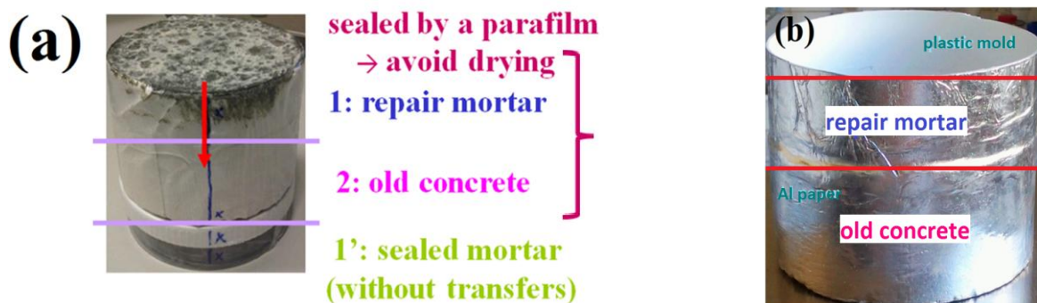
Figure 2.2: Schema of repair systems for (a) techniques in which metallic compounds are forbidden; (b) other traditional techniques.
