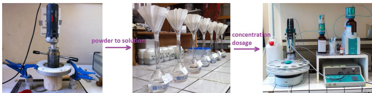
Figure 2.21: Dosage of chloride ions concentration
