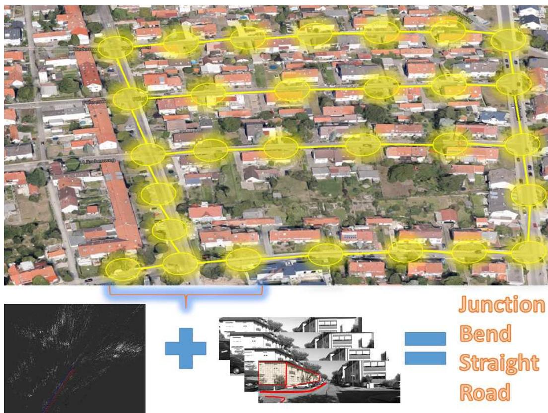
**Figure 1.7:** Global Mapping strategy is illustrated. Our map contains three different (at the same time mutually connected) steps: local metric reconstruction, topological map building and semantic path classification. **Top:** Topo-metric structure is shown under the graph. **Bottom:** Path classification step is illustrated.
