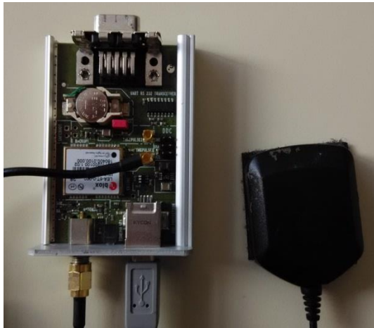
Figure 39 GNSS receiver and antenna used for the data collection
