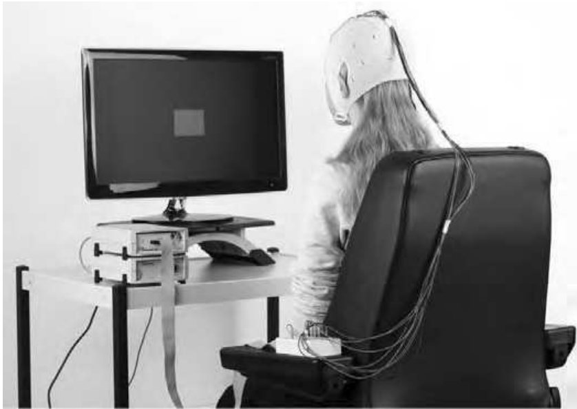
Figure 4. EEG is recorded from the scalp, commonly using between 16 and 256 electrodes. From Herrmann et al., 2015.
