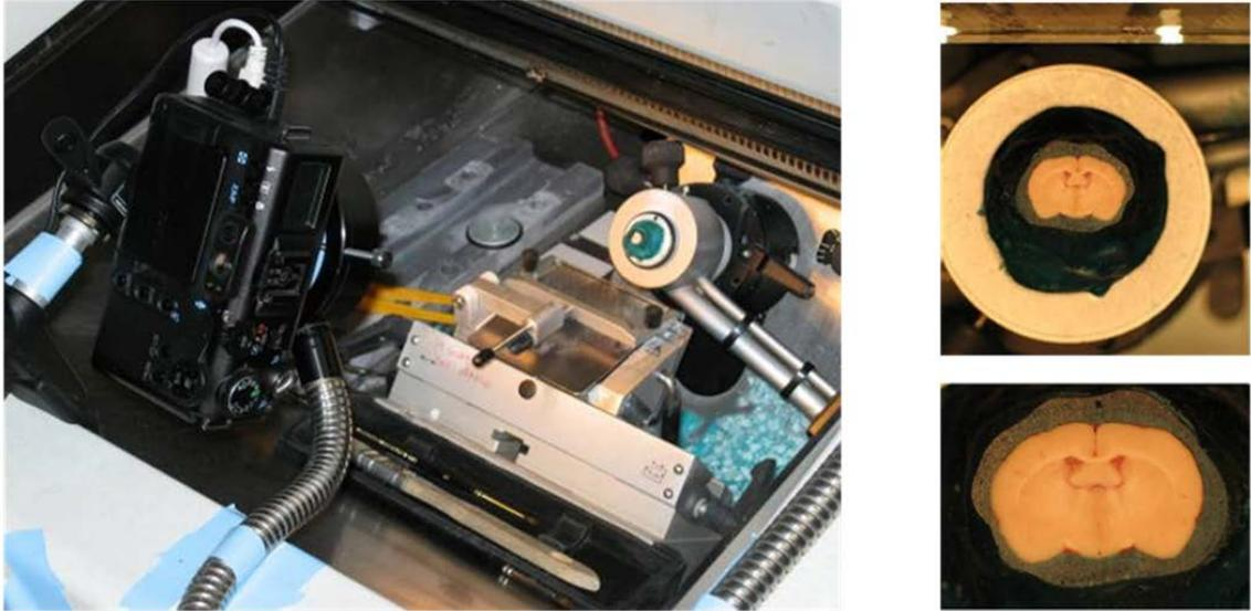
Figure 2.2: Block-face photography. Left: A camera device is fixed on top of a cryostat during brain sectioning. Right: Block-face photographs of a tissue section before it is removed from the tissue block.
