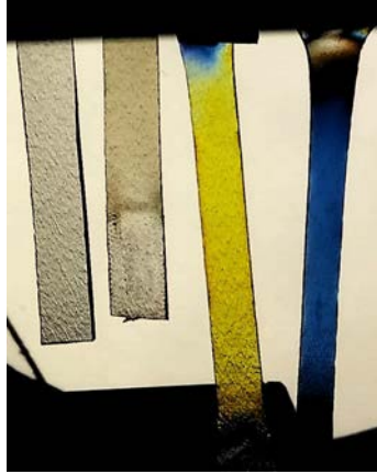
Figure 3.22: Four different samples initially with the same 20 mm length. From left to right: Reference sample in the initial shape, sample stretched at 200% at 20 °C, sample stretched at 200% at 50 °C and sample stretched at 200% at 70 °C. The samples are only clamped by their upper end despite what can be seen from the picture.
