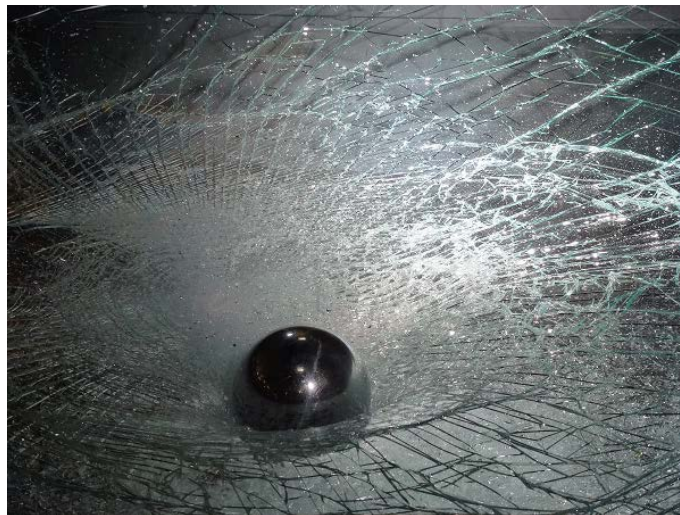
Figure 1.2: A 4 kg ball test used in European Standard EN 356. The ball is dropped three times on the glass which has to sustain the impacts [3].
