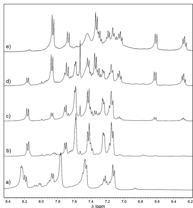
Figure 2. Portion of 1 H NMR spectrum in (CD 3 ) 2 CO of a solution of E-2 (a); E-2 and P(OMe) 3 immediately after addition of P(OMe) 3 (b), after 4 h at rt (c), and after 24 h at rt (d); and 1 H NMR spectrum of E-6b (e).
