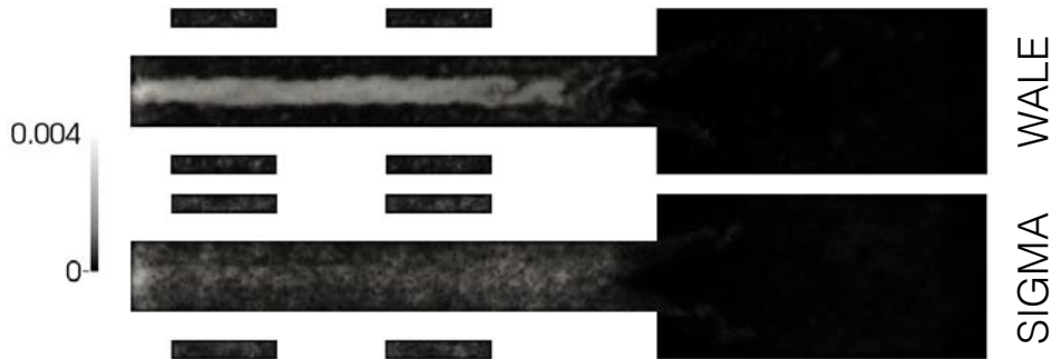
Figure 9.5: Turbulent viscosity (in \text{kg s}^{-1} \text{m}^{-1} ). Comparison between the WALE (top) and SIGMA (bottom) SGS models.
