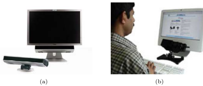
Figure 3.2: Two eye-tracking apparatus used in our experiments. (a) SMI © iView X TM RED, (b) Eye Link 1000 Remote/Head Free
