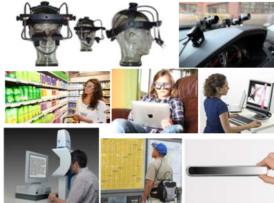
Figure 3.1: Commercial eye-trackers, a bench of solutions: head mounted devices, embedded in car or glasses, professional and clinical solutions or non-intrusive on a regular PC.
