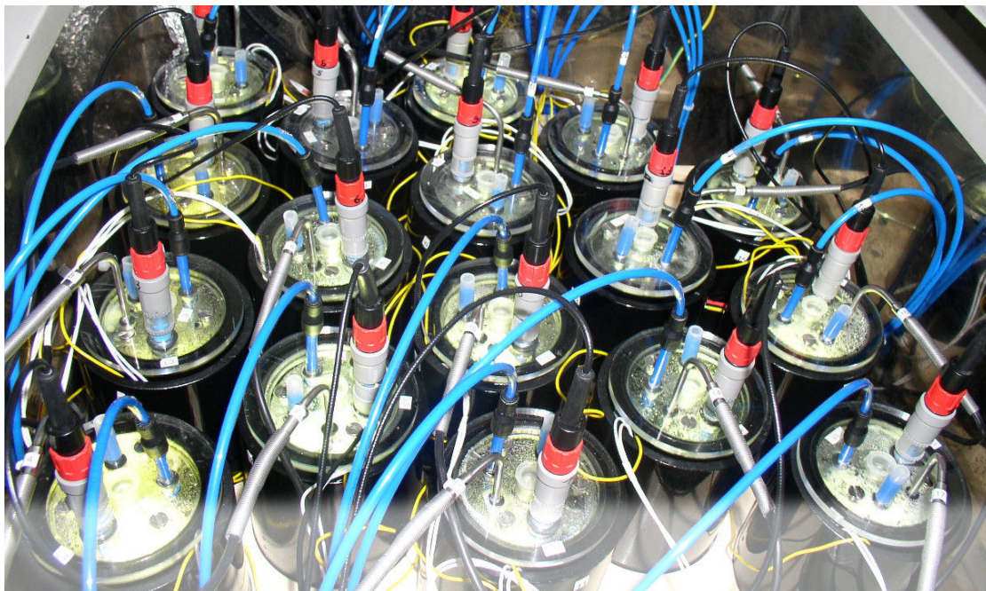
Figure 2.2: TIP device - Cultures of Tisochrysis lutea in the multifactorial TIP device designed at IFREMER Nantes.
