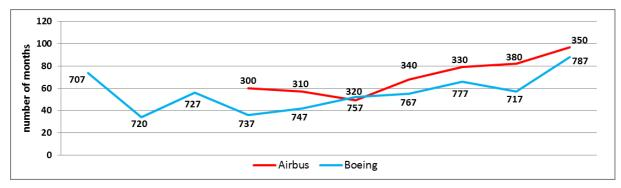
Figure 3.1: Length of the development period for new aircraft models of Airbus and Boeing
