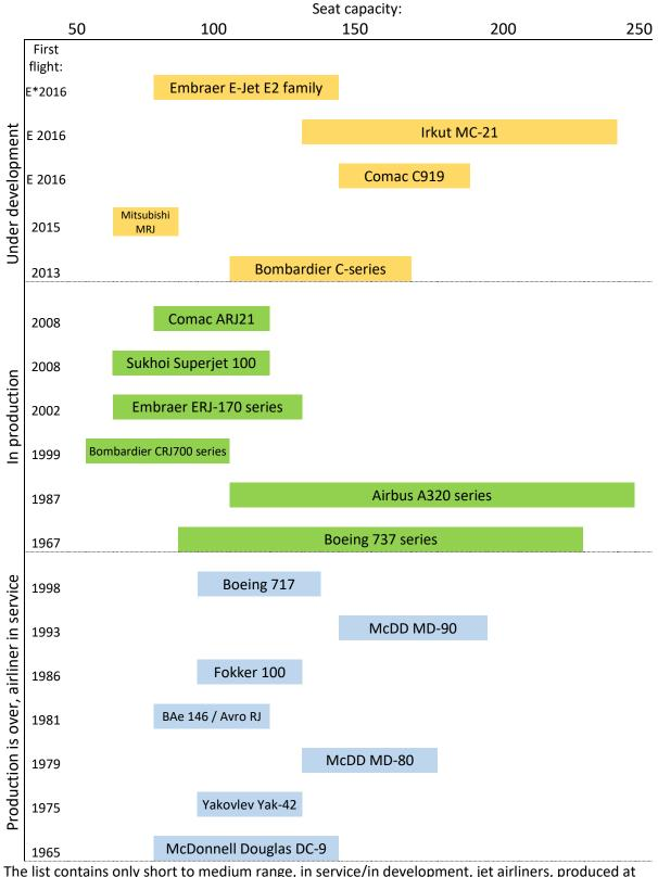
Figure 2.13: In service or in development short to medium rage jet aircrafts in the world
