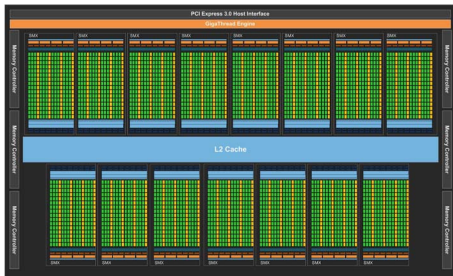
Figure 1.2: Block diagram of the Kepler K40m GPU.
