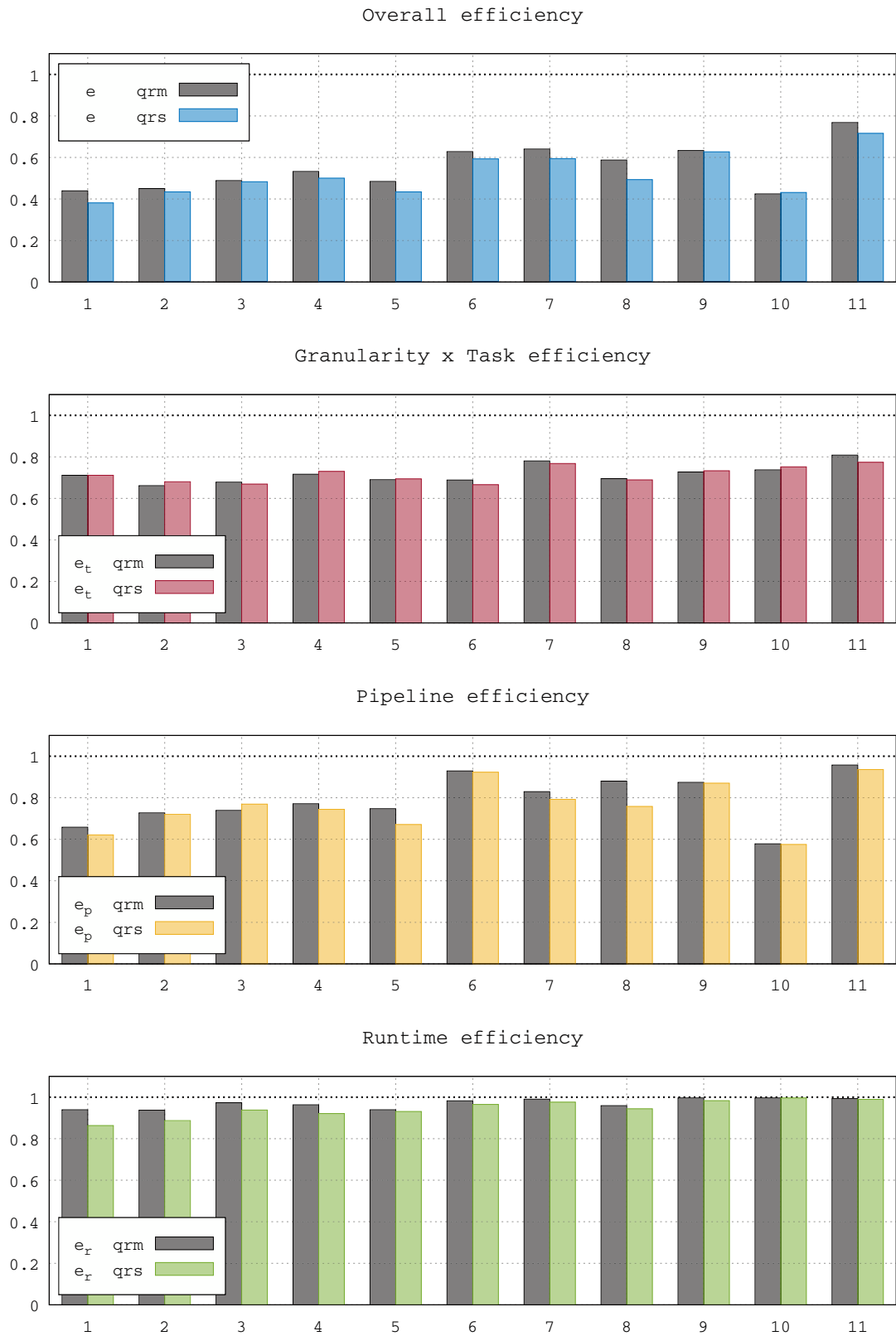
Figure 3.6: Efficiency measures for qr_mumps ( qrm ) and qr_mumps_starpu ( qrs ).
