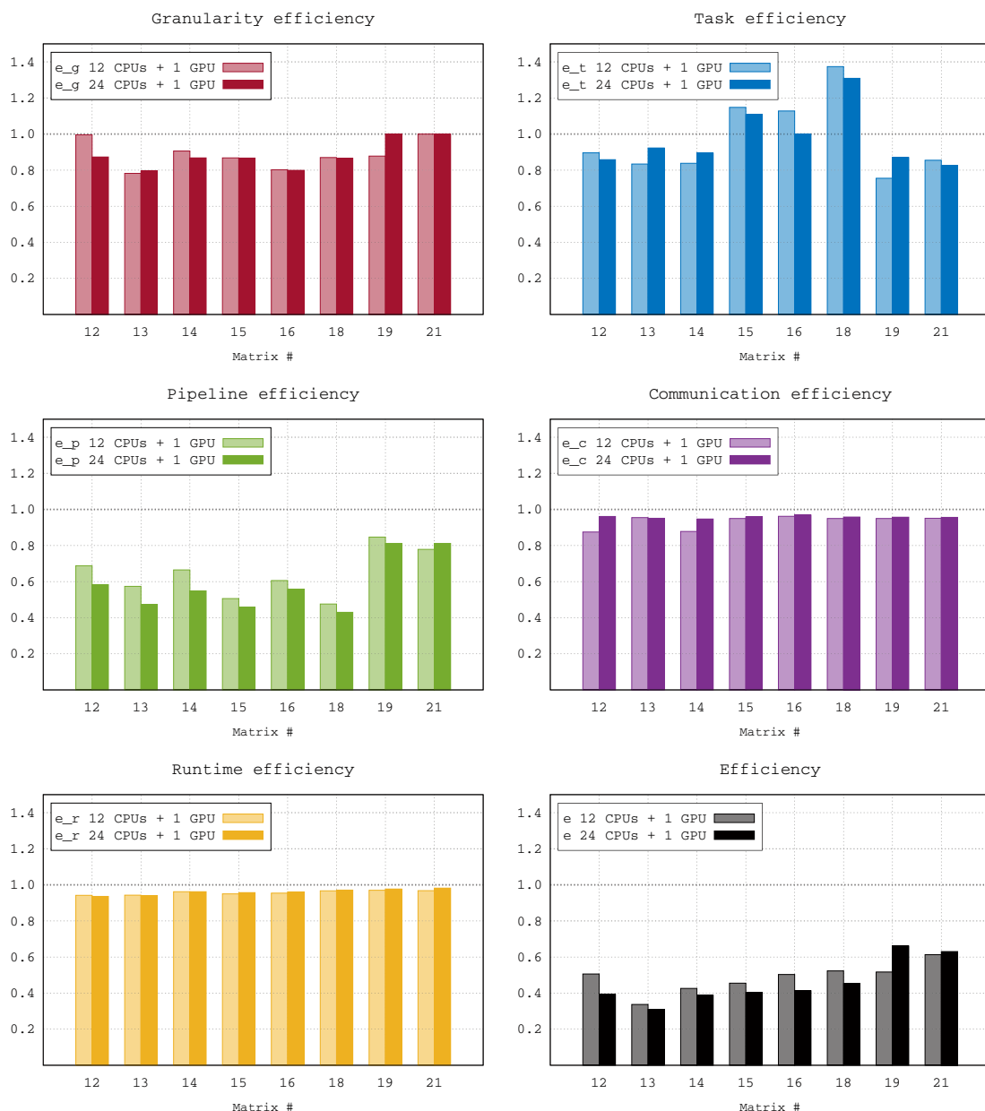
Figure 6.8: Efficiency measures for the STF heterogeneous algorithm on Sirocco with both configurations 12 CPUs ( 1 \times E5-2680 ) + 1 GPU ( 1 \times K40M ) and 24 CPUs ( 2 \times E5-2680 ) + 1 GPU ( 1 \times K40M ). Note that due to technical issues in StarPU, we are currently unable to obtain the efficiency measures for matrix # 17.
