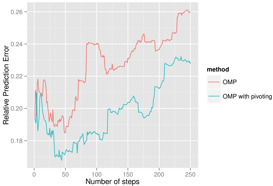
FIGURE 3.5. Comparison of the relative prediction error of OMP and and OMP with pivoting on text data with binary encoding.
