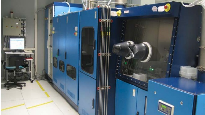
The MOCVD reactor at CNR-IMM, Agrate Brianza, Italy
