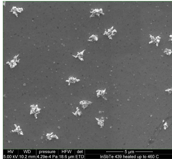
Figure 57: \text{In}_3\text{Sb}_{2.5}\text{Te}_{1.2} (sample 439) heated to 460°C and return to the room temperature (RT) - Heterogeneous surface
