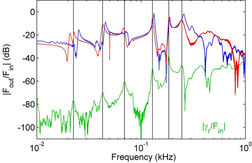
Figure 3.19: Modulus of the transfer function between the input force  $F_{in}$  and the output force  $F_{out}$  measured for 20 N (blue) and for 40 N (red) static compression. The green curve represents the transfer function between the radial acceleration  $\gamma_r$  of a supporting cylinder and the axial input force  $F_{in}$ . The black vertical lines indicate the resonant frequencies found experimentally at about 22.5, 42.8, 69, 128.6, 184.8 and 246.4 Hz.
