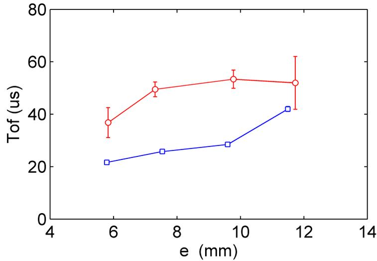
Figure 6.8: Time of flight (Tof) of the maximum of the envelope of transmitted pulses as a function of the sample thickness  $e$  (number of layers). Red circles are experimental results in the dry case and blue squares are experimental results in the wet case. Here, the input signal has a high amplitude.
