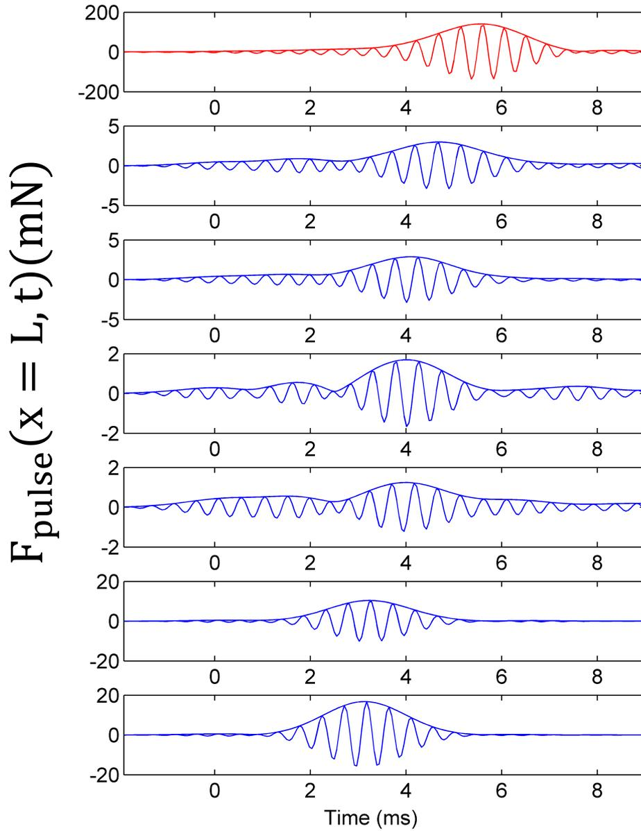
Figure 5.3: (a) Output deconvolved wavepacket  $F_{pulse}(x = L, t)$  in the dry media. In (b), (c), (d), (e), (f) and (g): output signals for wet media for viscosity of  $\mu = 0.1, 0.2, 0.5, 1, 5$  and  $10$  Pas; Here the static force is  $F_0 = 5$  N. The wavepackets are centered at  $f_c = 2.2$  kHz.
