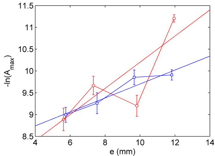
Figure 6.7: Maximum of the envelope of the transmitted pulses  $A_{max}$  as a function of the sample thickness  $e$  (number of layers). Red circles are experimental results in the dry case and blue squares are experimental results in the wet case. Here, the input signal has a low amplitude. The red and blue straight lines are best fits in the wet and dry cases, respectively.
