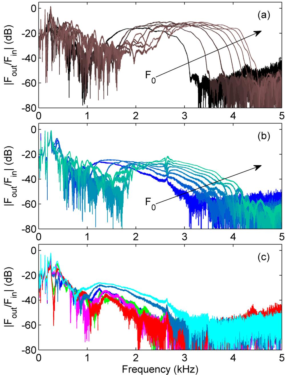
Figure 5.2: Magnitude  $|H|$  of the transfer function  $H = F_{out}/F_{in}$  versus frequency. (a) In the dry case for different static force  $F_0$ . (b) In the wet case as a function of  $F_0$  for viscosity  $\mu = 10$  Pas. (c) In the wet case at  $F_0 = 5$  N, but for viscosity of 0.1, 0.2, 0.5, 1, 5 and 10 Pas, shown respectively in green, blue, magenta, red, light blue and cyan curves.
