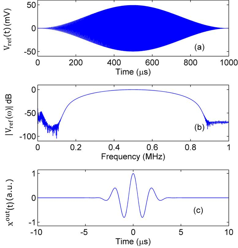
Figure 6.10: (a) Temporal representation of a signal generated by the arbitrary wave generator  $V_{ref}$  (Agilent 33500B). (b) Modulus of the Fourier transform of (a). (c) Cross-correlation  $x^{out}(t)$  between the reference signal  $V_{ref}(-t)$  and the signal transmitted through the sample  $V_{acq}(t)$ .
