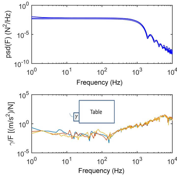
Figure 3.15: (a) Power spectral density of the force measured with an impact hammer while kicking the table on which stands the setup. (b) Acceleration  $\gamma$  measured by an accelerometer glued on a side of the table. (b) The different colors show different experimental conditions: in blue the hammer kicks the table as is, in red a 40 kg mass is set on top of the table and in yellow the table is firmly constrained against a wall. The inset shows a sketch of the experiment (b).
