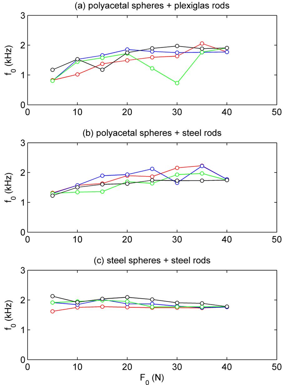
Figure 3.14: Low cutoff frequency  $f_0$  estimated at -20 dB below the average value of the propagative band (see Fig. 3.13). (a) Polyacetal spheres with plexiglas supports, (b) polyacetal spheres with steel supports and (c) steel spheres with steel supports. The red curves correspond to the first increase of the static force, from 5 N to 40 N, the blue curves to the first decrease, from 40 N to 5 N, the green curves to the second increase and the black curves to the second decrease.
