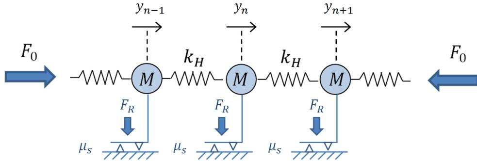
Figure 3.6: An alignment of particles with mass  $M$  and radius  $R_0$  interacting via an elastic potential with stiffness  $k_H$ . The particles are pressed against the ground with a force  $F_R$ , for instance the weight of each particle, and interact with the ground via a Coulomb's coefficient of friction  $\mu_s$ .
