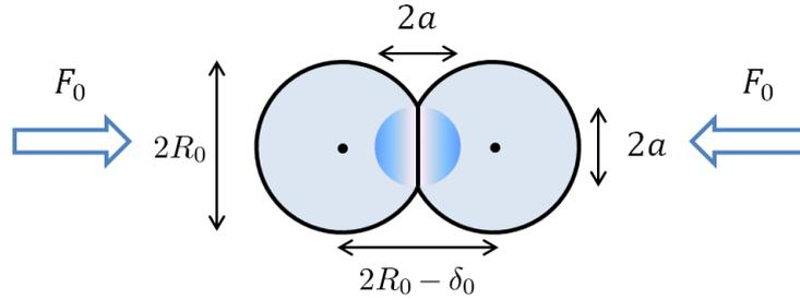
Figure 2.3: Two spheres with radius  $R_0$  compressed with a static force  $F_0$ .
