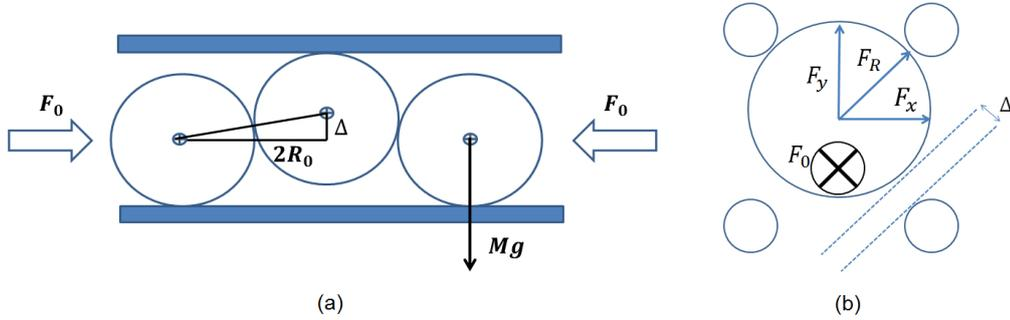
Figure 4.2: (a) Spheres with radius  $R_0$ , weight  $Mg$  and clearance  $\Delta$  under compression  $F_0$ . (b) Axial view, where  $F_y$  is the projection of  $F_0$  and  $F_r$  is the radial force.
