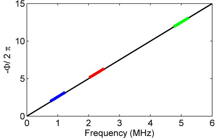
Figure 3.4: Phase delay  $\Phi$  of the transfer function as a function of frequency for longitudinal waves centered at 1 MHz (blue), 2.25 MHz (red) and 5 MHz (green). The black curve is a guide line showing the linear regression  $\Phi = \omega e / c_L$ .
