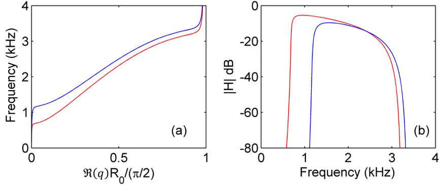
Figure 4.4: (a) Theoretical dispersion relation, where  $\Re(q)$  is the real part of the wave number and  $R_0$  is the sphere radius, (b) modulus of the transfer function. Here the results are estimated for polyacetal spheres under a 20 N static compression. The spheres are supported by four 1 m long rods with Young's Modulus of  $E_s \simeq 0.1$  GPa (red curves) and with  $E_s \simeq 200$  GPa (blue curves).
