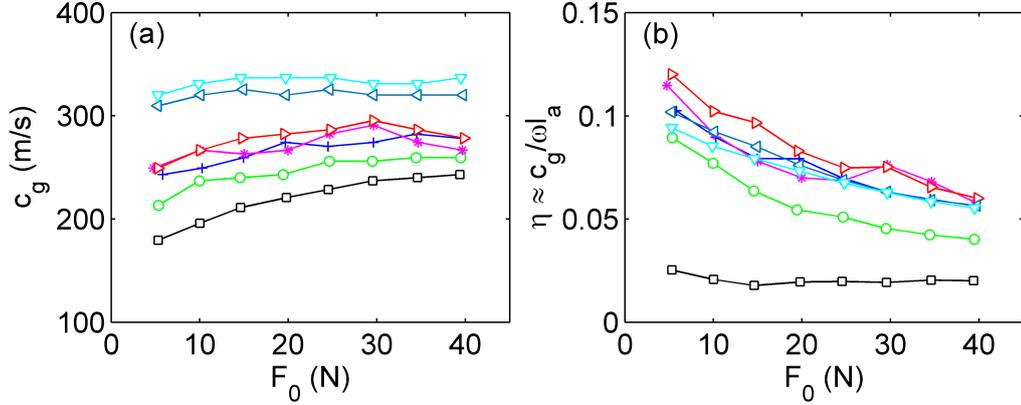
Figure 5.5: (a) Group velocity  $c_g$  and (b) loss factor  $\eta = c_g/\omega l_a$  at central frequency  $f_c$ . The dry case is shown in black squares, the wet cases with viscosity of 0.1, 0.2, 0.5, 1, 5 and 10 Pa.s are traced respectively in green  $\circ$ , blue  $+$ , magenta  $*$ , red  $\triangleright$ , light blue  $\triangleleft$  and cyan  $\nabla$ .
