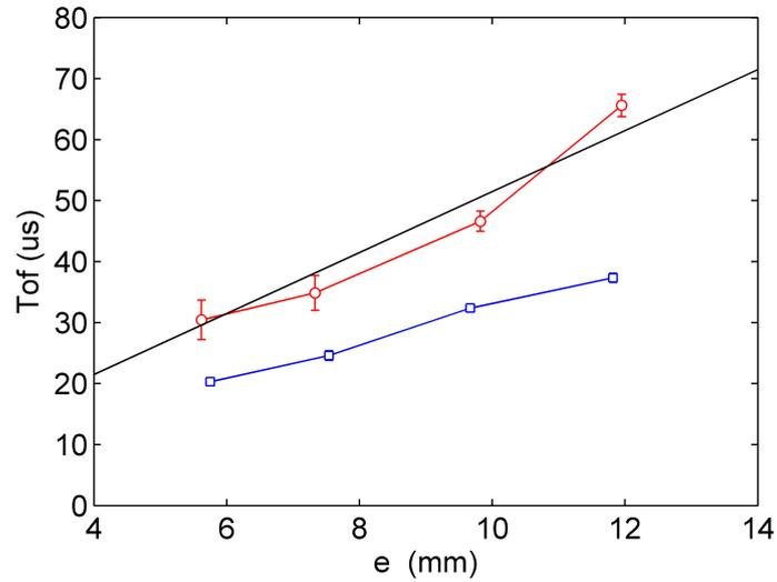
Figure 6.6: Time of flight (Tof) of the maximum of the envelope of transmitted pulses as a function of the sample thickness  $e$  (number of layers). Red circles are experimental results in the dry case and blue squares are experimental results in the wet case. The black line indicates the wave speed given by the EMT theory, see Eq. 6.1. Here, the input signal has a low amplitude.
