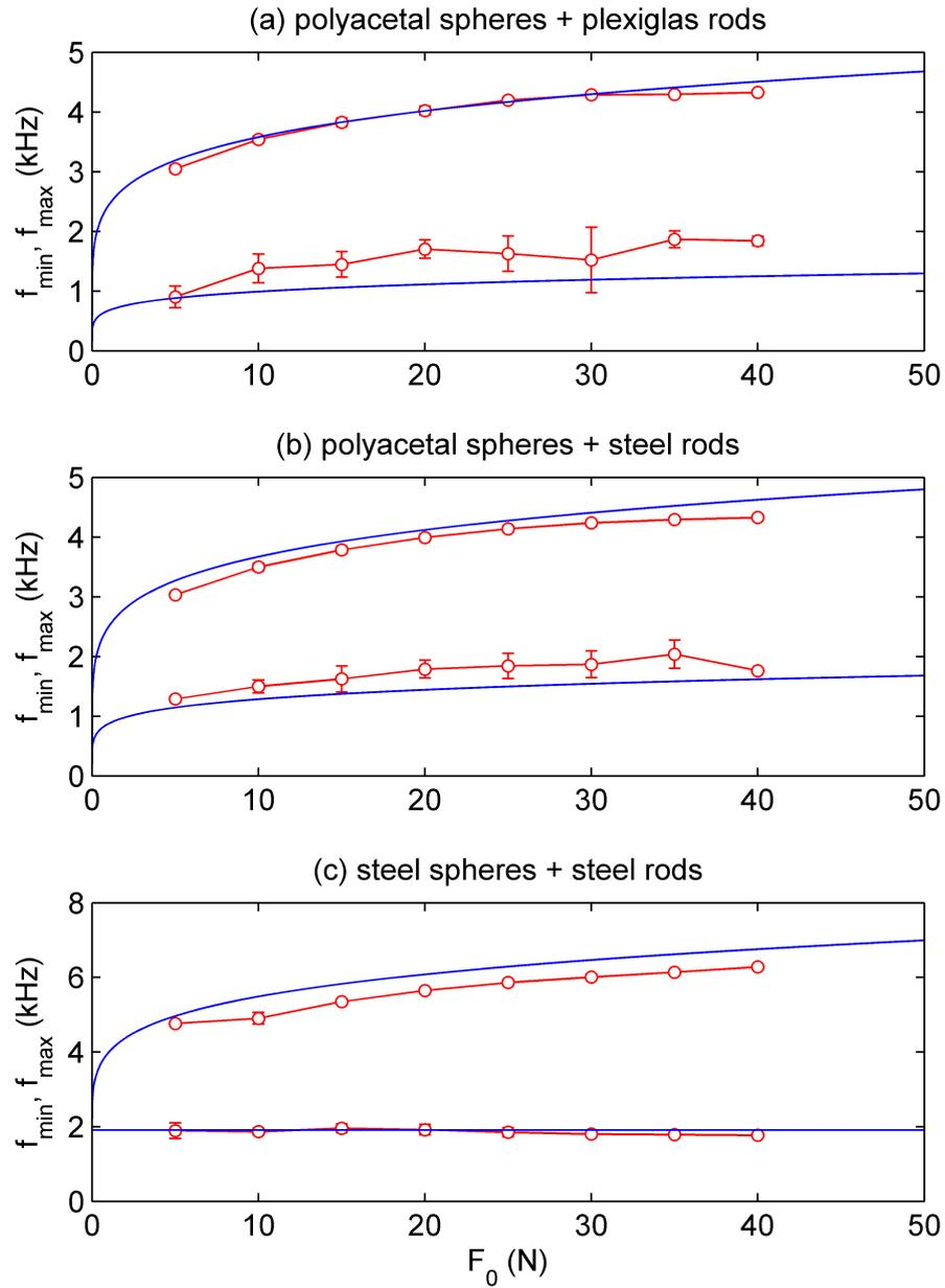
Figure 4.3: Lower and upper cutoff frequencies,  $f_{min}$  and  $f_{max}$ , as a function of the static force in the axial direction. (a) Configuration with polyacetal spheres and plexiglas supports, (b) polyacetal spheres with steel supports and (c) steel spheres with steel supports. Blue lines represent Eq. 4.6 and Eq. 4.7 and red dots are the experimental data extracted from Fig. 3.13 and shown in Fig. 3.14.
