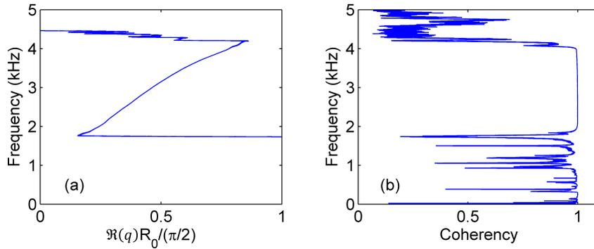
Figure 4.5: (a) Measured dispersion relation for polyacetal spheres with steel support and  $F_0 = 20$  N, in response to chirp excitation.  $\Re(q)$  is the real part of the wave number and  $R_0$  is the radius of the spheres. (b) Coherency between the output and input signals.
