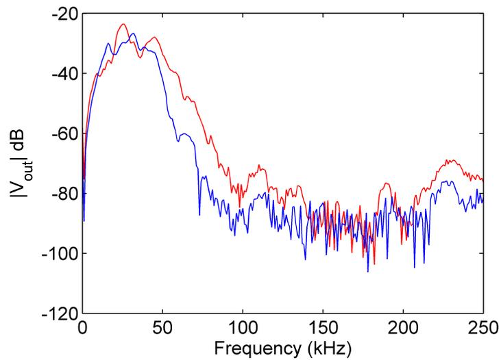
Figure 6.5: Example of Fourier transform of signals propagating through three (red curve) and five (blue curve) layers of polyacetal spheres.
