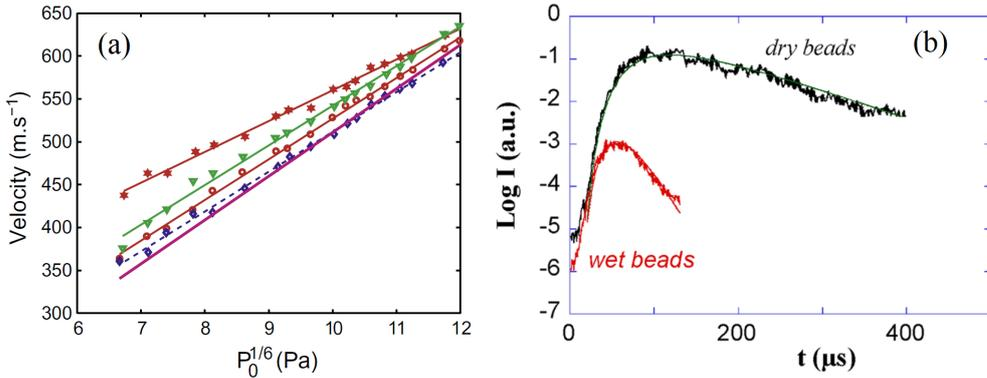
Figure 2.18: (a) Wave speed as a function of confinement pressure: in purple is the Hertz-Mindlin model, in red  $\circ$  a dry configuration, in blue  $\diamond$  with water, in green  $\nabla$  with an oil with viscosity 50 mPas and in red  $\star$  with a fluid with viscosity 10 Pas [107]. (b) Averaged intensity  $I$  in dry and wet granular packings: the solid lines stands for fitted models [108].
