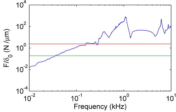
Figure 3.18: Effective stiffness  $k_E$  of the end extremity, as the ratio between the force  $F$  measured by the impact hammer and the displacement  $\delta_0$  measured from the accelerometer. The red line (resp. the green line) indicates the typical stiffness  $k_H$  between two steel spheres (resp. between two polyacetal spheres).
