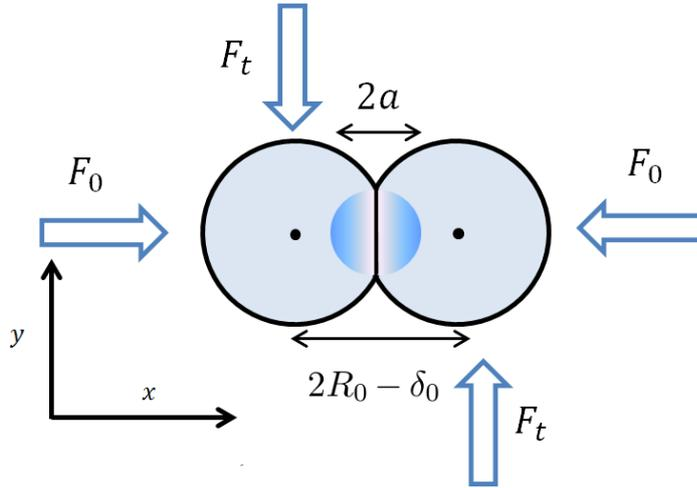
Figure 2.5: Two spheres with radius  $R_0$  pushed against each other with a static force  $F_0$ ; an additional tangential force  $F_t$  is applied causing micro displacement or shearing in  $y$ -axis.
