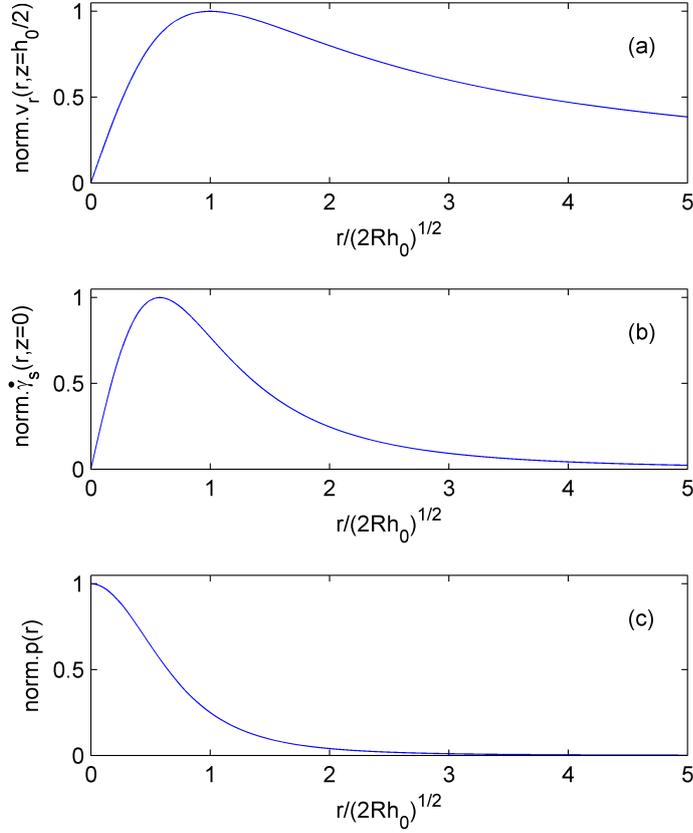
Figure 2.9: (a) Normalized radial velocity, (b) normalized shear rate and (c) normalized hydrodynamic pressure distribution as a function of the normalized radial coordinate  $r/\sqrt{2Rh_0}$ . Here,  $h_0$  is the minimal distance between the sphere and the plane and  $R$  is the radius of the sphere.
