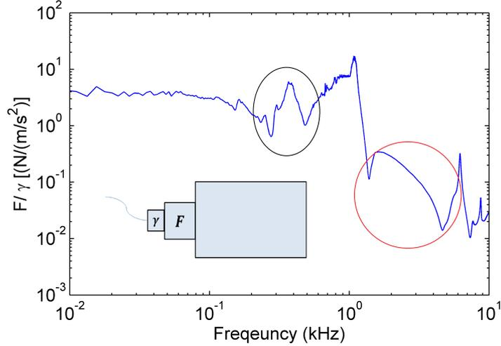
Figure 3.16: Modulus of the transfer function between the acceleration  $\gamma$  captured by an accelerometer glued on the static force sensor and the force  $F$  recorded by an impact hammer. One can observe resonances near 280 Hz and 470 Hz and anti-resonance near 380 Hz (see inside the black circle). Inside the red circle, resonances are observed in the 1-5 kHz frequency region. In inset, a sketch showing the experimental configuration.
