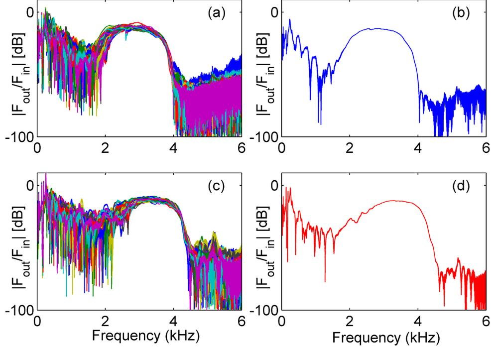
Figure 4.11: (a,c) 40 realizations of the transfer function  $H(\omega) = F_{out}/F_{in}$  between the signals measured at the beginning  $F_{in}$  and at the end  $F_{out}$  of the alignment, as a function of frequency; (a) is at 20 N static compression and (c) at 40 N. (b,d) Average magnitude  $|H|$  over the 40 realizations at 20 N and 40 N, respectively.
