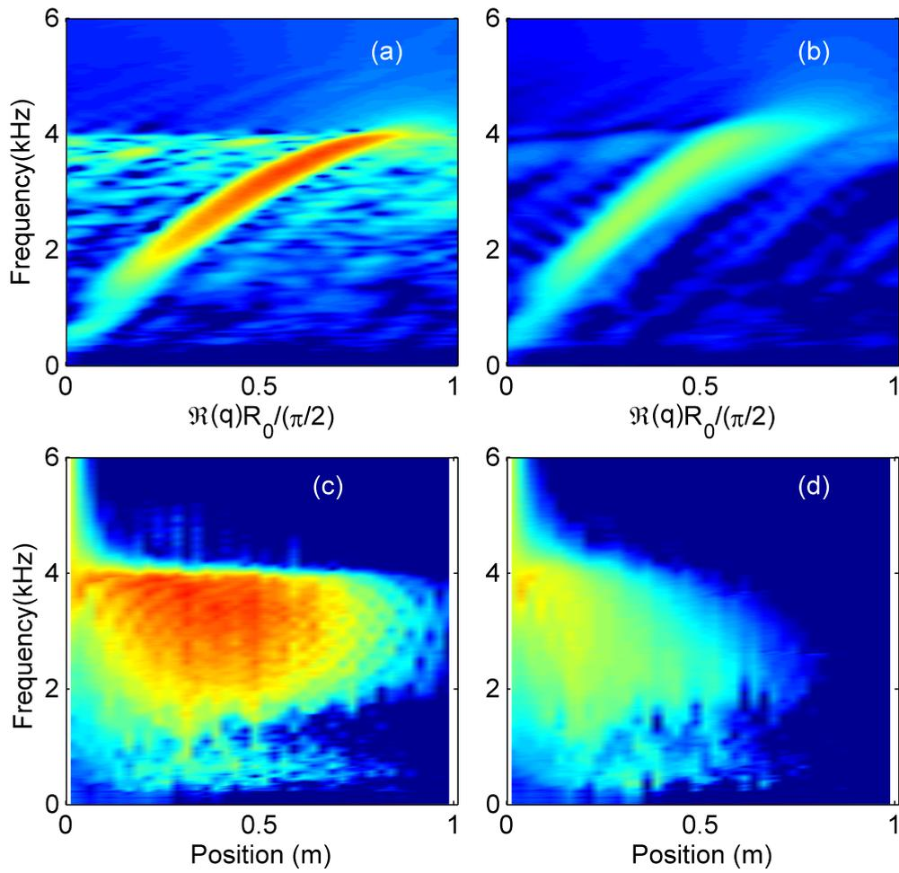
Figure 5.9: (a,b) Dispersion relation unraveled by the use of the embedded sensor in the dry and the wet cases, respectively. Here, the fluid viscosity is  $\mu = 1$  Pa.s. (c,d) Modulus of the transfer function measured by the embedded sensor in the dry and the wet cases, respectively. Here, the static compression is 20 N and  $\Re(q)$  is the real part of the wave number and  $R_0$  is the radius of the spheres.
