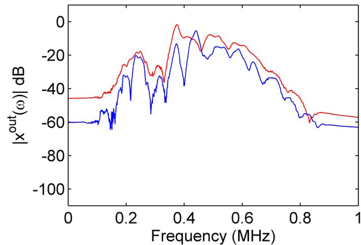
Figure 6.12: Fourier transform of the signals propagating through two  $x_2^{\text{out}}$  and three  $x_3^{\text{out}}$  layers of dry granular media, in red and in blue respectively.
