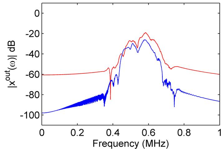
Figure 6.16: Fourier transform of the signals propagating through two  $x_2^{\text{out}}$  and three  $x_3^{\text{out}}$  layers of wet granular media, in red and blue respectively. The signals are here filtered with a gaussian filter centered at 0.5 Mhz and with a bandwidth equal to 0.15.
