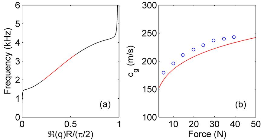
Figure 4.8: (a) Theoretical dispersion relation for polyacetal spheres with steel support under  $F_0 = 20$  N static force. From (a), one estimate the theoretical group velocity as the average slope over the frequency range indicated in red. (b) Experimental (blue dots) group velocity,  $c_g$ , at central frequency  $f_c = (f_{max}(F_0) + f_{min}(F_0))/2$ .
