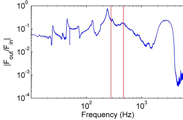
Figure 3.17: Modulus of the transfer function between the signal measured at the beginning  $F_{in}$  and at the end  $F_{out}$  of the chain as a function of frequency, under 20 N static compression. Here, the configuration is an alignment of polyacetal spheres on steel rods. Red lines indicate the values of the resonant frequencies measured in Fig. 3.16
