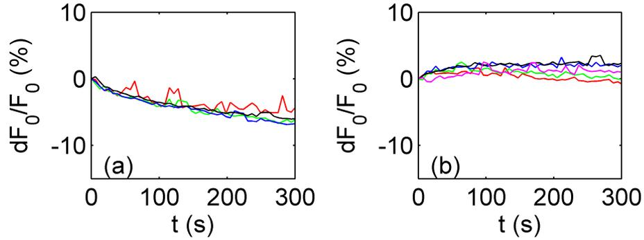
Figure 3.9: Relative decay of the static force  $F_0$  measured as a function of time  $t$ . (a) Protocol 1A: temporal evolution of the static force from set points 10 N, 20 N, 30 N and 40 N in red, green, blue and dark respectively. (b) Protocol 1B: temporal evolution of the static force at 20 N after having waited 1 min, 2 min, 3 min 4 min and 5 min in red, green, blue, dark and magenta respectively at the static force of 40 N. Here, the system is not excited by a dynamic signal.
