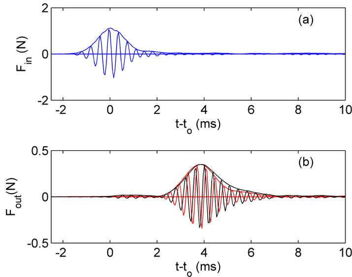
Figure 4.7: (a) Input signal measured at the beginning of the chain  $F_{in}(t) = F_{pulse}(x = 0, t)$ . (b) Output signal measured as the response of gaussian pulse excitation  $F_{out}^g(t)$  (black curve) and as the convolution of the input (a) with the experimental transfer function measured from the response of broadband chirp excitation  $F_{out}(t) = F_{pulse}(x = L, t)$  (red curve, see the details of the method in Sec. 4.1.4).
