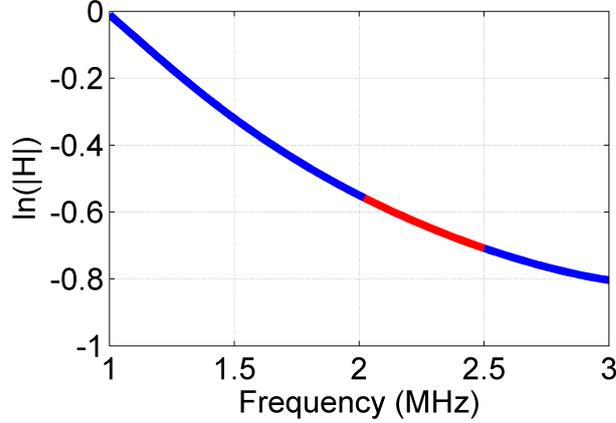
Figure 3.5: Natural logarithm of the modulus of the transfer function versus frequency. The loss angle estimated from Eq. 3.8 near the central frequency (here around 2.25 MHz) of the transducer is shown in red.
