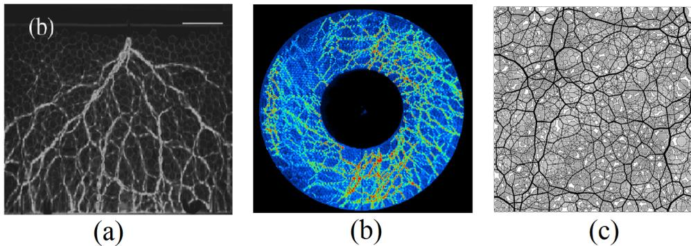
Figure 2.13: Photoelastic pictures of the heterogeneous force chains which support most of the load in compressed granular media. (a) The media is either submitted to a point force [89] or (b) under shear stress [87]. (c) Numerical simulations showing the network of normal forces in polydisperse granular media [88].
