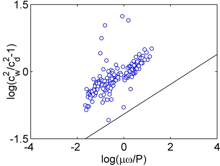
Figure 5.7: Ratio between the group velocity in the wet case  $c_w$  and the dry case  $c_d$  traced as a function of the viscosity  $\mu$ , angular frequency  $\omega$  and confinement pressure  $P = F_0/\pi R_0^2$ . The experimental data are traced for all static forces  $F_0$ , viscosity  $\mu$  and central frequencies  $f_c$ ,  $f_{c1}$  and  $f_{c2}$ . The black line is a guide line indicating a power law with an exponent  $1/3$ .
