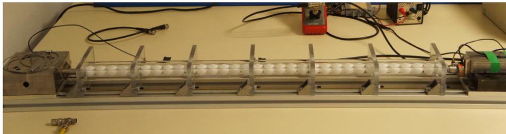
Figure 3.1: Experimental setup, here consisting of 32 identical polyacetal spheres aligned on four plexiglas rods.
