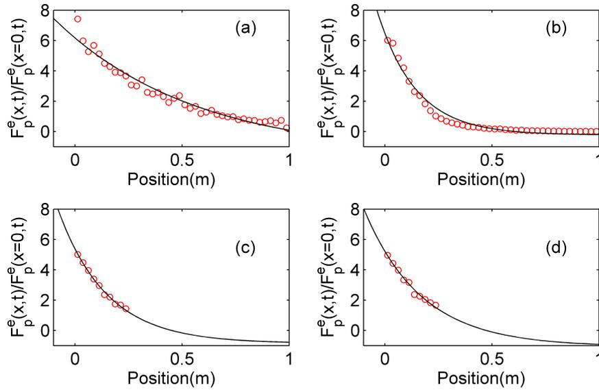
Figure 5.11: Evolution of the attenuation  $\max[F_p^e(x, t)] / \max[F_p^e(x = 0, t)]$  as a function of the position  $x = 2nR$  inside the chain; experimental results are shown in red dots and the black line stands for the Eq. 5.21. (a) Dry chain of spheres and in (b,c,d) wet chains of spheres with interstitial fluid with viscosity of 1 Pas, 5 Pas and 10 Pas, respectively. Here, the alignments are both under a 20 N compression.
