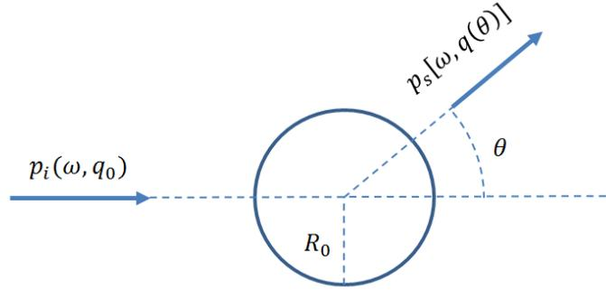
Figure 6.2: A plane wave scattered by a sphere.
