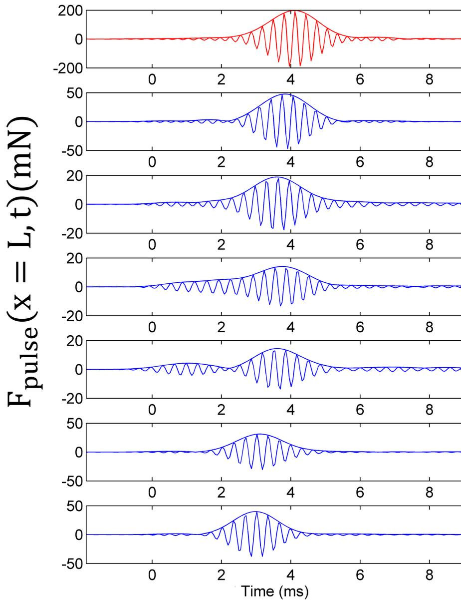
Figure 5.4: (a) Output deconvolved wavepacket  $F_{pulse}(x=L, t)$  in the dry media. In (b), (c), (d), (e), (f) and (g): output signals for wet media for viscosity of  $\mu = 0.1, 0.2, 0.5, 1, 5$  and  $10$  Pas; Here the static force is  $F_0 = 40$  N. The wavepackets are centered at  $f_c = 3.2$  kHz.
