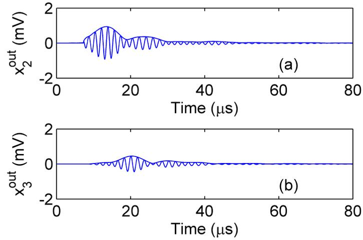
Figure 6.15: (a,b) Signals propagating through two  $x_2^{\text{out}}$  and three  $x_3^{\text{out}}$  layers of wet granular media, respectively. The signals are here filtered with a gaussian filter centered at 0.5 Mhz and with bandwidth equal to 0.15.
