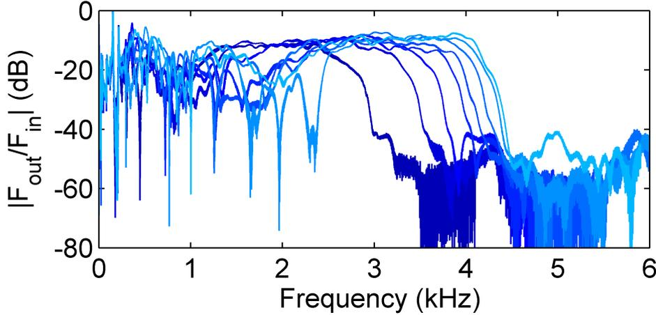
Figure 3.12: Modulus of the transfer function between the force measured at the beginning  $F_{in}$  and at the end  $F_{out}$  of the chain as a function of frequency. Different colors correspond to different applied static forces  $F_0$ . Here, the spheres are in polyacetal and the rods are in plexiglas.
