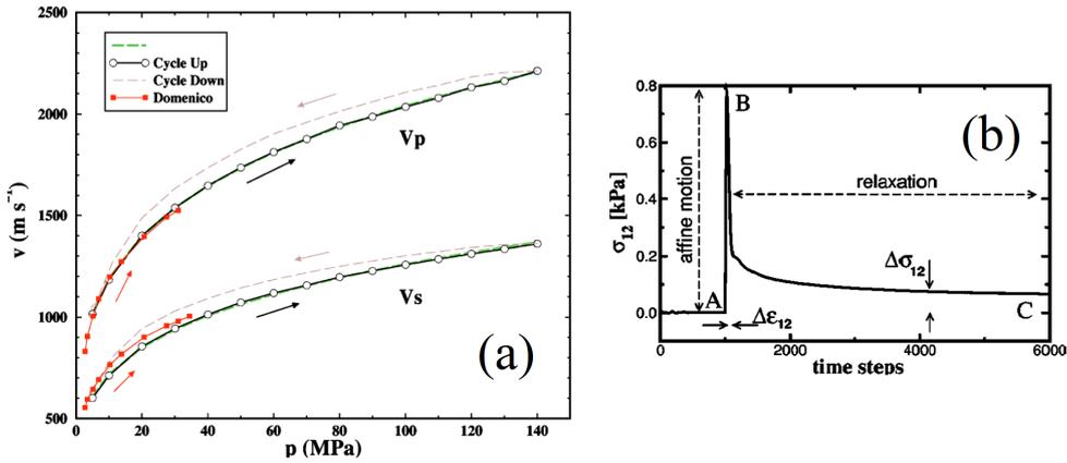
Figure 2.17: (a) Evolution of the longitudinal wave speed  $V_p$  speed as a function of the confinement pressure  $P$ . (b) The relaxation of the shear stress  $\sigma_{12}$ : the path from points A to B indicates an affine motion while the relaxation takes place B to C.
