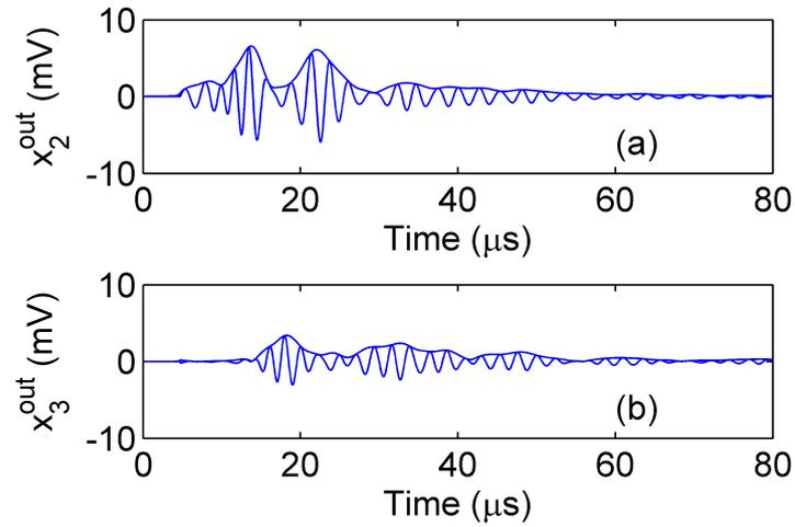
Figure 6.11: (a,b) Signals propagating through two  $x_2^{\text{out}}$  and three  $x_3^{\text{out}}$  layers of dry granular media, respectively.
