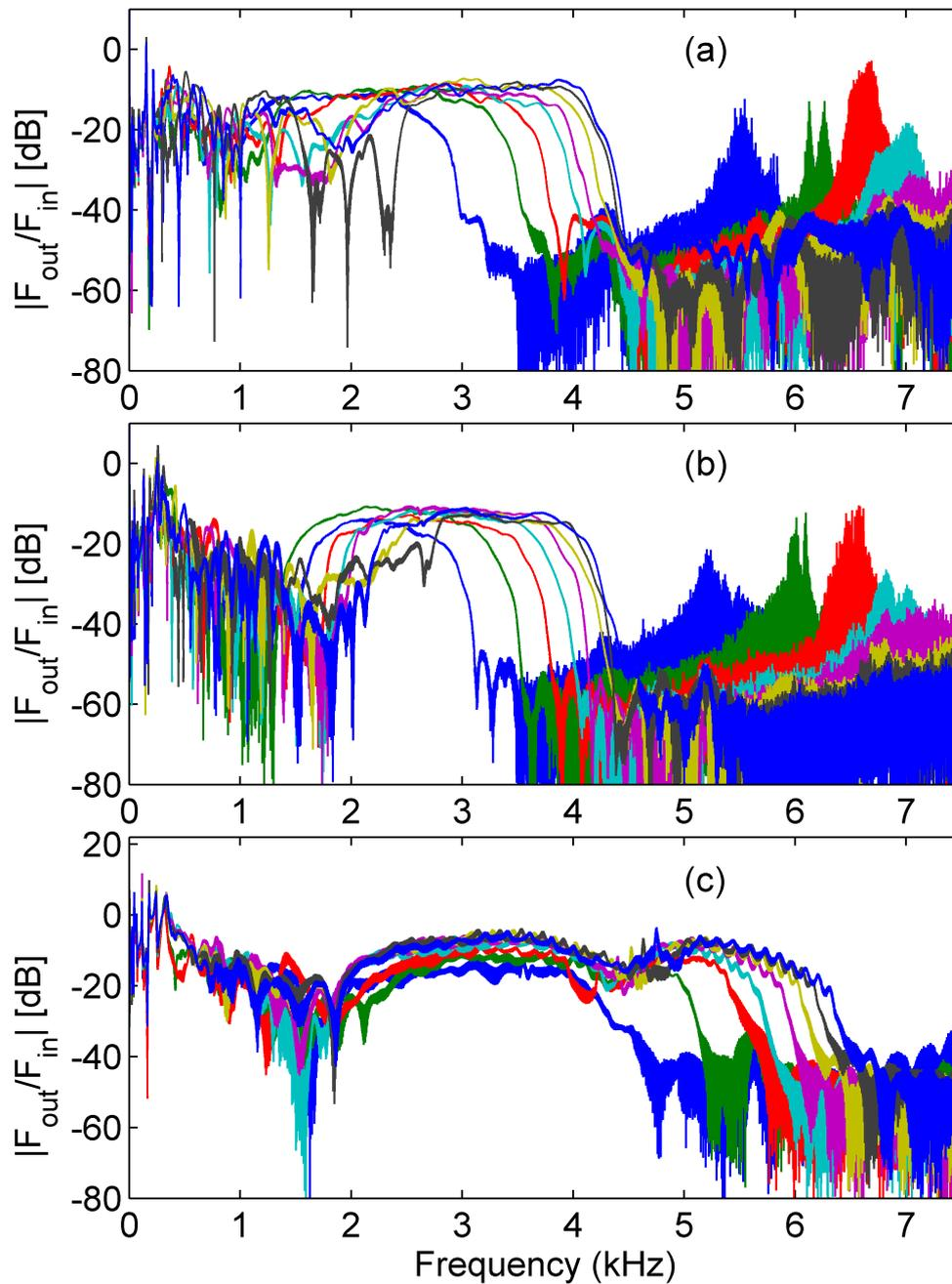
Figure 3.13: Modulus of the transfer function, for dry chain between the output signal  $F_{out}$  and input signal  $F_{in}$  as a function of frequency; different colors show different static force applied  $F_0$  ranging from 5 N to 40 N every 5 N. (a) The results for configuration with polyacetal spheres and plexiglas supports, (b) polyacetal spheres and steel supports and (c) steel spheres and steel supports.
