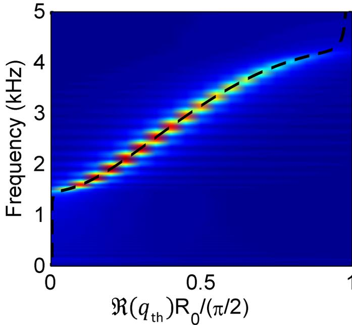
Figure 4.10: Dispersion relation  $K_{th}$ , the dashed line is Eq. 4.11. Here the simulations and the analytic estimation are performed for polyacetal spheres with steel rods under  $F_0 = 20$  N static compression.
