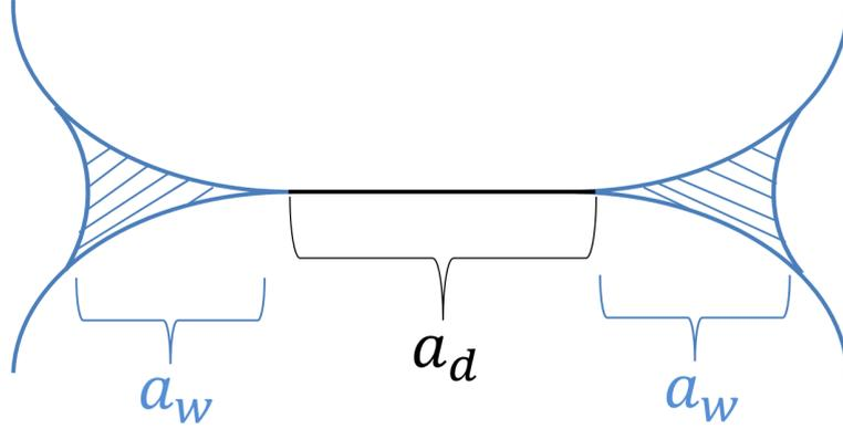
Figure 5.6: Sketch of the contact region between two compressed wet spheres. Here,  $a_d$  is the extent of the dry contact while  $a_w$  indicates the extent of the hydrodynamic field in the fluid. Such a framework is compatible with the one given by Marshall [63].
