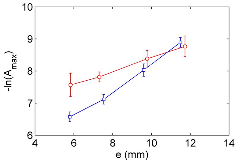
Figure 6.9: Maximum of the envelope of transmitted pulses  $A_{max}$  as a function of the sample thickness  $e$  (number of layers). The red circles are experimental results in the dry case and the blue squares are experimental results in the wet case. Here, the input signal has a high amplitude.
