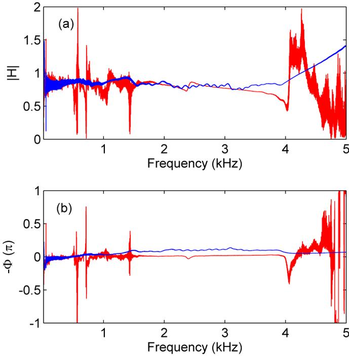
Figure 3.8: Transfer function  $H(\omega) = F_{emb}/F_{ref}$  between the signals acquired by the embedded sensor and the reference dynamic force sensor  $F_{ref}$ , where  $F_{ref} = F_{in}$  is the dynamic force sensor in front of the piezoelectric actuator (the blue curve) and  $F_{ref} = F_{out}$  is the dynamic force sensor on the output side (the red curve). Results are shown in modulus (a) and in phase (b) as a function of frequency.
