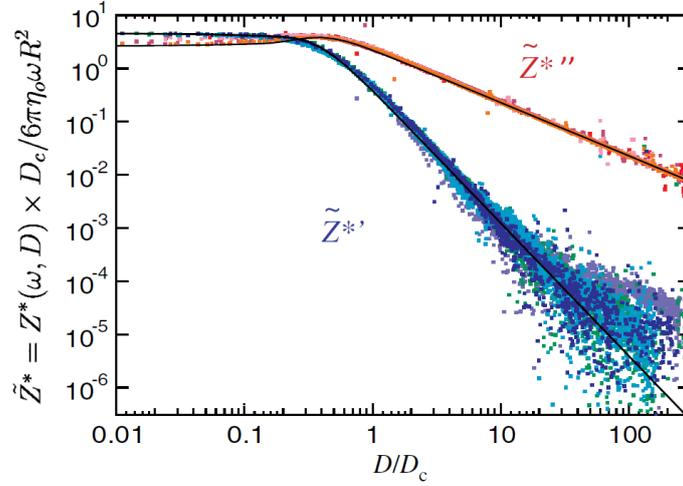
Figure 2.11: Normalized mechanical impedance  $Z$  ( $\kappa_\omega$  in our notations) as a function of the normalized separation distance  $D$ . The elastic part is shown in blue and the viscous part is shown in red [81].  $D_c$  is the critical distance,  $\omega$  is the angular frequency,  $R$  is the radius of sphere and  $\eta$  is the viscosity.
