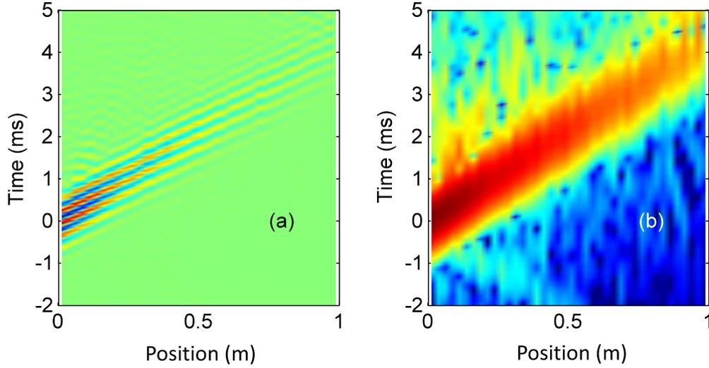
Figure 4.13: (a) Output signal  $F_{pulse}(x, t)$  deconvolved from the transfer function measured at each position inside the alignment and as a function of time. (b) Envelope of the pulse  $F_{pulse}^{env}(x, t)$  as a function of time and position. Both results obtained by the method given by Eq. 4.31 and Eq. 4.32 while considering an input wavepacket centered at 3.25 kHz and bandwidth 0.3, at  $F_0 = 40$  N static force.
