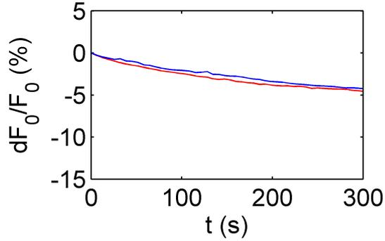
Figure 3.11: Relative decay of the static force as a function of time  $t$  with experimental protocol C, for a 20 N static force and during 5 min. In red, the response without solicitation (protocol 1C), in blue the response with solicitation (protocol 2C).
