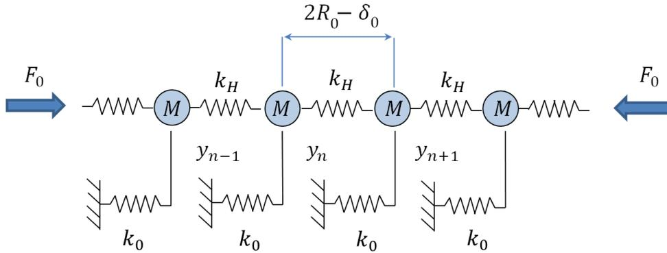
Figure 4.1: One-dimensional chain of spheres with mass  $M$  under static compression  $F_0$  interacting via a Hertzian contact stiffness  $k_H$ , with an additional stiffness  $k_0$  which quantifies the interaction of the spheres with the support.
