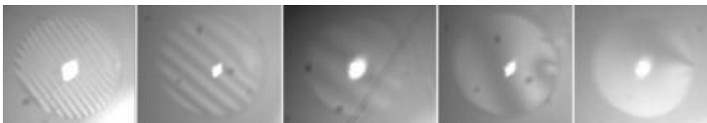
Figure 7.14.: Interference pattern between the crystal face and the fiber end observed with the camera. From left to right the fiber alignment is better and better until the two faces are parallel (right).
