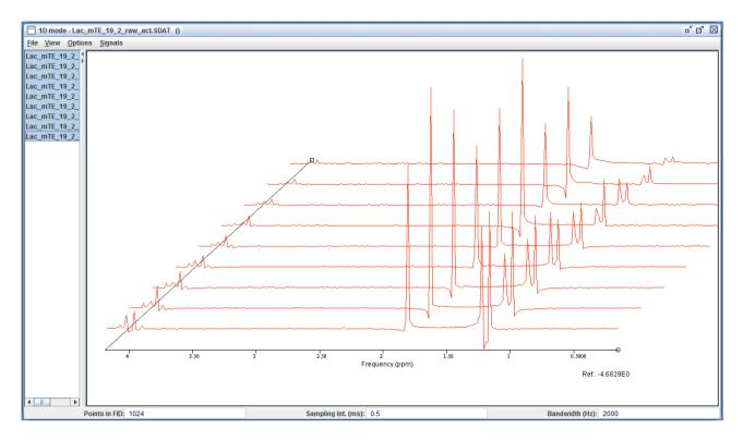
Figure 32: Acetate and Lactate spectrum with multi-echo sequence acquired with TE multiples of 288 ms. TE(ms) = 29, 288, 576, 864, 1152, 1440, 1728, 2304, 2880. TR = 6000 ms. NSA = phase cycles = 16.
