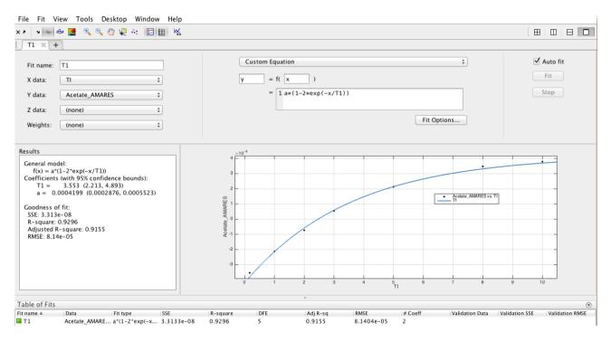
Figure 21: Example of Acetate T1 estimation with cftool using f1 function for fitting. Area under the peaks have been estimated by AMARES. As shown the signal don't saturates.
