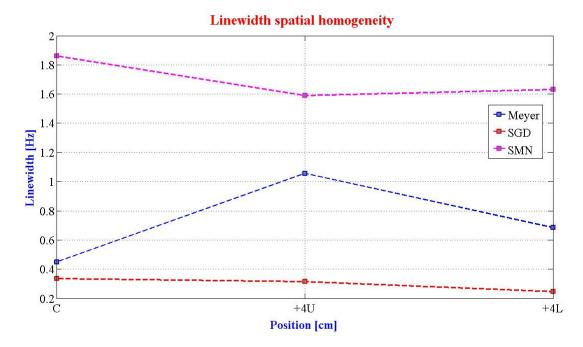
Figure 16: Linewidth spatial homogeneity. "C" means central position, "+4U" means a displacement of 4 cm upper, while "+4L" means lateral. For Meyer data it must be taken in account that data come from a 3T MR scanner.
