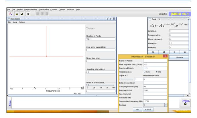
Figure 58: example of water spectra simulation using QUEST. Scanner 3T, bandwidth 2000 Hz, sampling 0.5 ms. Alpha and Beta parameters are for a Voight curve.
