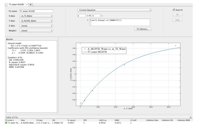
Figure 19: example of water data fitting with MATLAB-cftool using f1 function for fitting. Data obtained by HLSVD algorithm.
