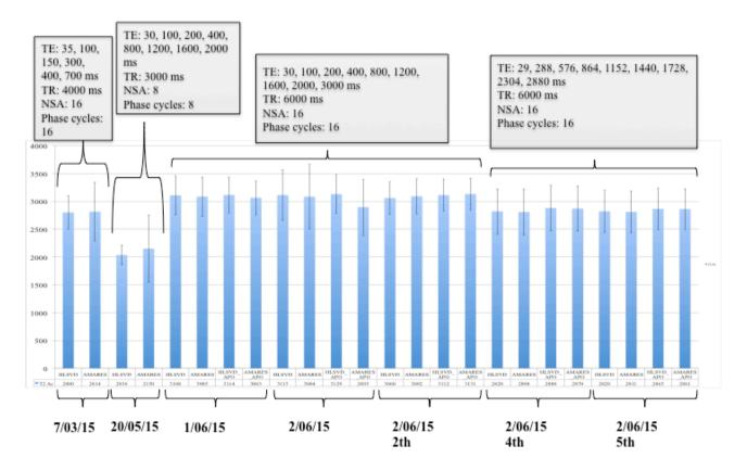
Figure 30: Acetate T2. Error bars have been estimated automatically by the fitting procedure with MATLAB-cftool.
