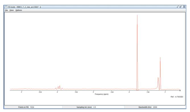
Figure 38: Spectrum of Siemens phantom. Metabolites peaks are visible. TR = 4000 ms, TE = 35 ms.
