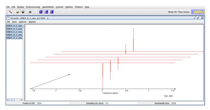
Figure 17: Example Water spectrum with multi-inversion time displayed in jMRUI. TI(ms): 30, 250, 700, 2500, 5400. TE = 35 ms. TR = 6000 ms. NSA = 16, Phase cycles = 16. Inv. Bandwidth = 1500 Hz.
