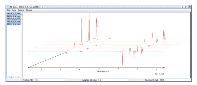
Figure 18: Example of metabolities spectrum with multi-inversion time displayed in jMRUI. The residual water peak is visible at about 4.7 ppm. Metabolites peaks: acetate at about 1.9 ppm, lactate doublet at about 1.3 ppm and lactate quadruplet at about 4.1 ppm. TI(ms): 30, 250, 700, 2500, 5400. TE = 35 ms. TR = 6000 ms. NSA = 16, Phase cycles = 16. Inv. Bandwidth = 1500 Hz.
