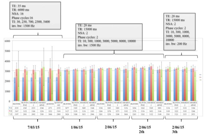
Figure 20: Water T1 estimation at different time with different sequence parameters, algorithms (HLSVD, AMARES and QUEST). Apodization has been tested for all the algorithms. Error bars have been estimated automatically by the fitting procedure with MATLAB-cftool.
