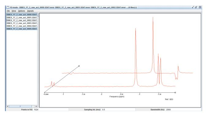
Figure 31: Lactate and Acetate peaks. Distorsions in Lactate peaks are clearly visible in the backward spectrum (TE 700 ms), while in the front spectrum (TE = 35 ms) there are no distorsions.
