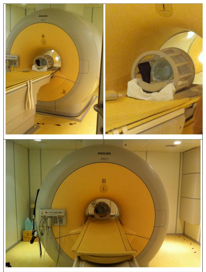
Figure 2: Siemens phantom inserted into the Philips Achieva 1.5 T MR scanner at the Santa Maria Nuova hospital.
