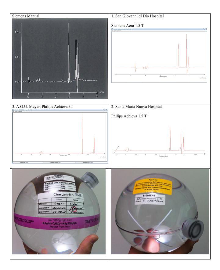
Figure 1: Siemens phantom. Top left: spectrum from Siemens Manual [Ref. 89]; top right: 1. spectrum acquisition at San Giovanni di Dio Hospital with Siemens Aera MR scanner at 1.5 T; middle right: 2. spectrum acquisition at Santa Maria Nuova with Philips Achieva MR scanner at 1.5 T. Left middle panel: spectrum acquisition at Meyer Philips Achieva 3 T; Bottom left: Metabolites concentration certified from Siemens; Bottom right: ID number.
