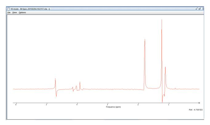
Figure 35: Metabolites spectrum from Siemens phantom acquired at SGD. Data: "Spettro\_04feb2015\_fantoccio\_Siemens"
