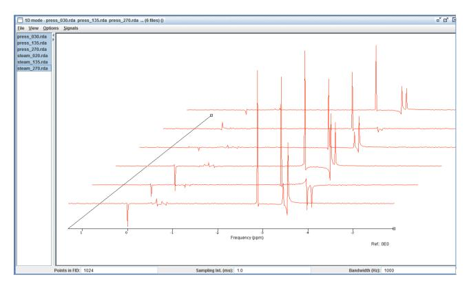
Figure 36: PRESS and STEAM spectra performed on Siemens phantom in date 5 september 2014. Data from "SVS\_QA\_fantoccio\_siemens\_5set14"
