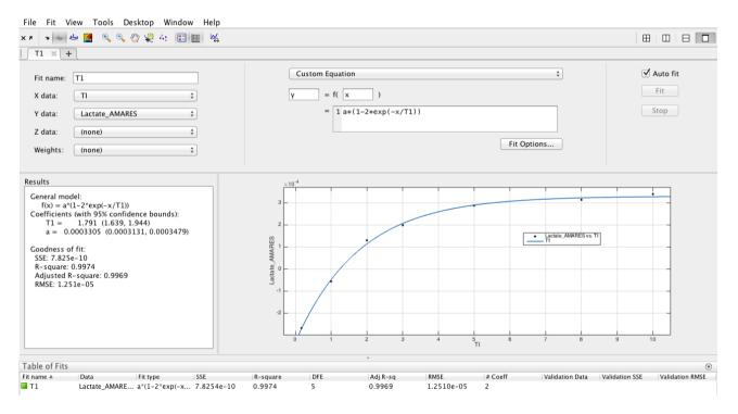
Figure 23: Example of Lactate T1 estimation with cftool using f1 function for fitting. Area under the peaks have been estimated by AMARES. As shown the signal saturates at about 8 s.
