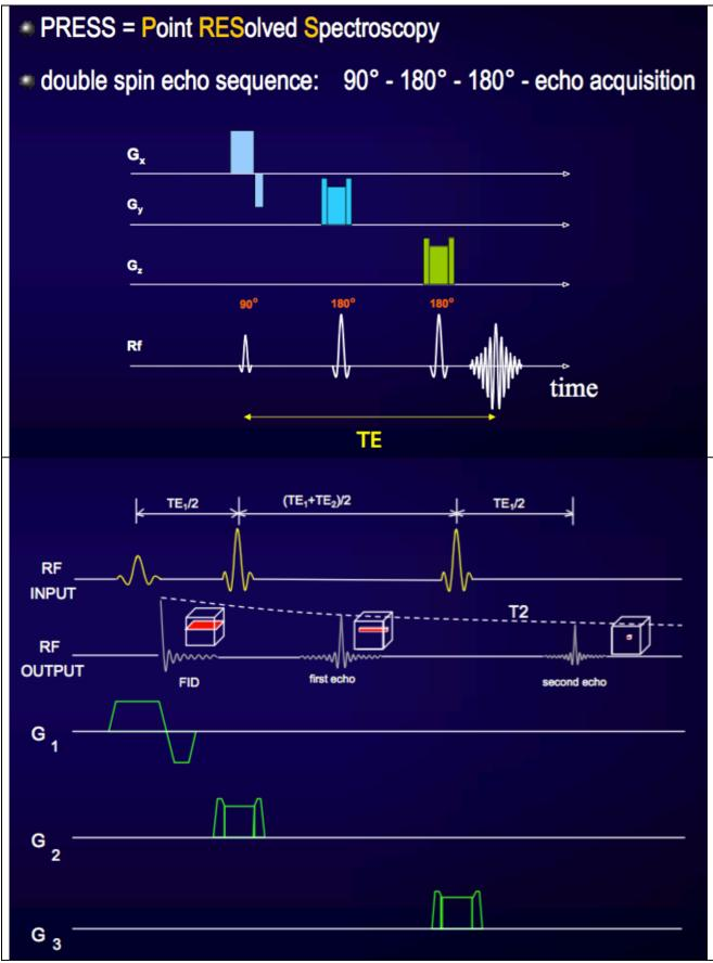
Figure 3: PRESS – Point RESolved Spectroscopy sequence scheme.
