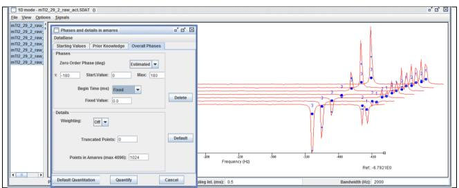
Figure 26: Example os AMARES parameters setting for Acetate and Lactate T1 estimation. Sequence 2/06/15 3th. Inv. Bw = 300 Hz, center at 400 Hz. Lactate doublet: peaks 1, 2; Lactate quadrouplet: peaks 4, 5, the other two have a too low SNR to be estimated; Acetate: peak 3.
