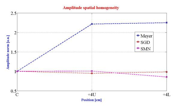
Figure 15: Amplitude spatial homogeneity. "C" means central position, "+4U" means a displacement of 4 cm upper, while "+4L" means lateral. Data are normalized to "Central position".
