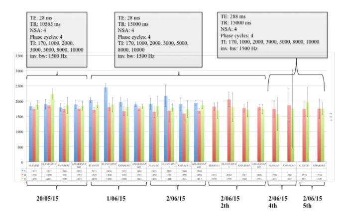
Figure 25: Lactate T1 doublet and quadrouplet estimation at different time with different sequence parameters, algorithms (HLSVD, AMARES). Apodization has been tested for all the algorithms. Error bars have been estimated automatically by the fitting procedure with MATLAB-cftool.
