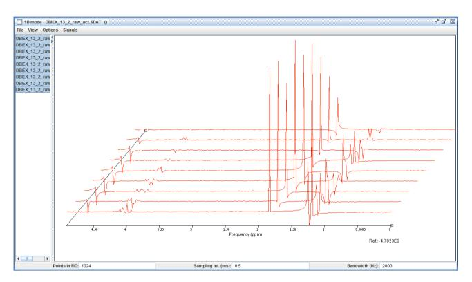
Figure 29: Example of Acetate and Lactate spectrum with multi-echo sequence. These TE echo times are not correct for estimation of Lactate peaks area as clearly shown. TE(ms): 30, 100, 200, 400, 800, 1200, 1600, 2000, 3000. TR = 6000 ms. NSA = phase cycles = 16.
