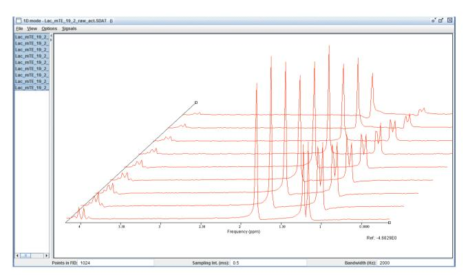
Figure 33: Acetate and Lactate spectrum with multi-echo sequence acquired with TE multiples of 288 ms. Spectrum have been apodized with a Lorentzian of 5 Hz. TE multiples of 288 ms.
