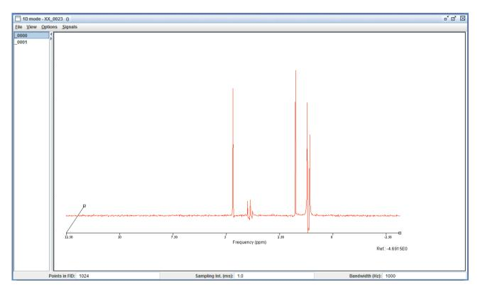
Figure 37: Siemens phantom spectrum with water suppression, acquired at SMN with PRESS sequence. TE 30 ms. Data: "Phantom\_siemens\_19marzo15"
