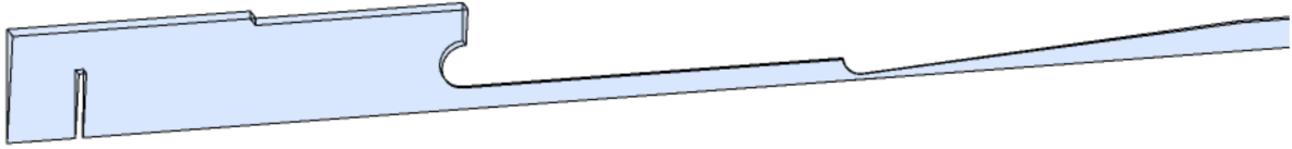
Figure 1.25: Sketch of the 3D-URANS computational domain segment [Mühlbauer 2009].
