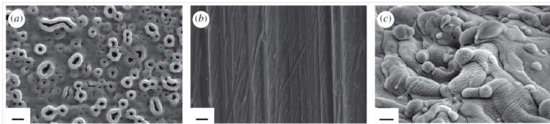
Figure I- 13 : SEM images of modified titanium surfaces (a) anodic oxidized surface (TiUnite, Nobel Biocare) showing volcanoes porous structure (b) machined surface (Fixture Original, Branemark Integration) showing ridges and valleys along the turning direction (c) laser-modified surface showing a combined surface roughness in both the micro- and nanoscale. (Scale bars, 5 \mu\text{m} ). From (Palmquist et al., 2010).
