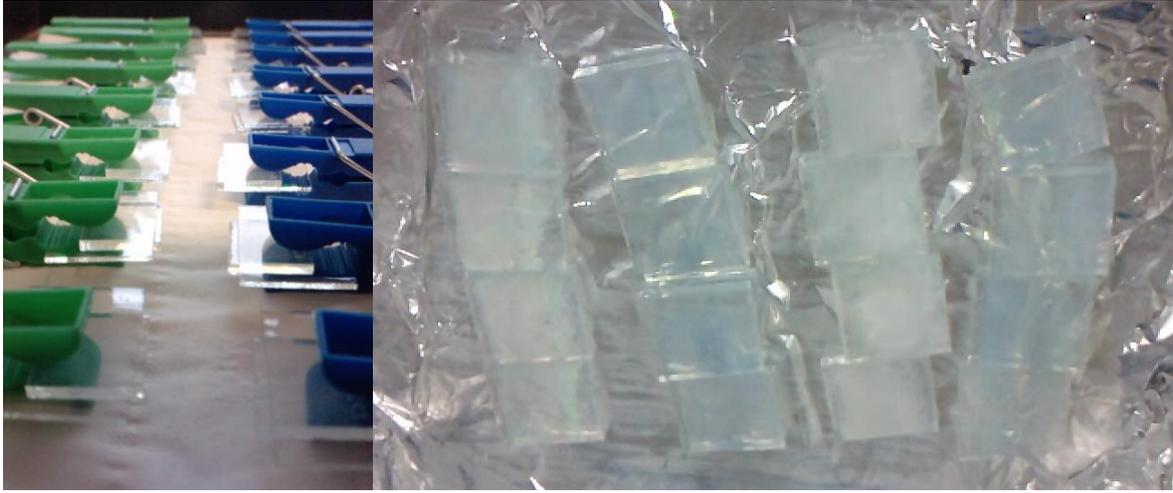
**Figure 116 (left) Infiltrated opals clamped with a glass slide and left to dry overnight. (Right) Infiltrated substrates before PS bead removal**
