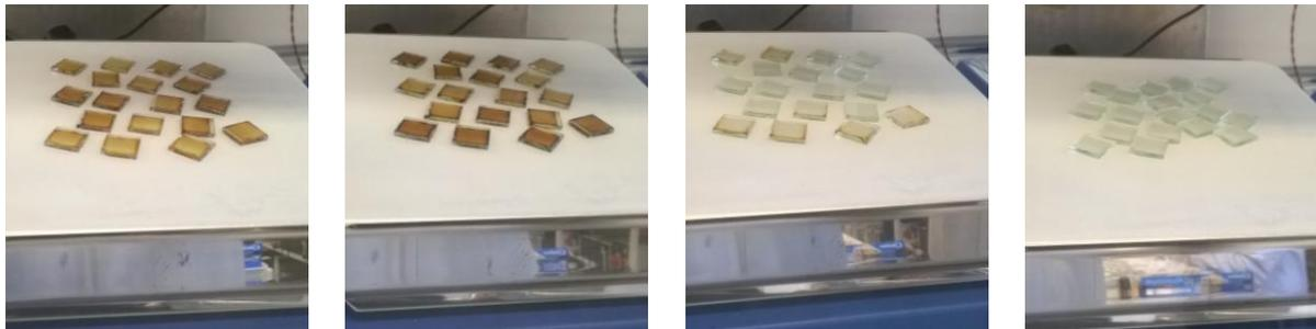
**Figure 114.** Changes in substrate appearance at (from left to right) 250 °C, 350 °C, 450 °C and 500 °C
