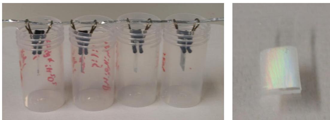
**Figure 110. (Left) Photograph to demonstrate how the glass slides were vertically supported. (Right) Photograph of a substrate coated with 595 nm PS beads after the vertical deposition process.**
