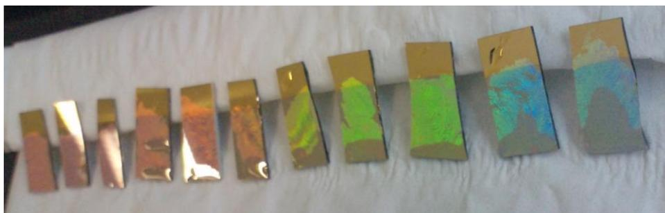
**Figure 112. Pictures of transferred monolayers consisting of 430 nm PS beads on substrates.**
