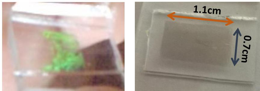
Figure 123. Photographs of gold nanopillar arrays after transferring onto PDMS
