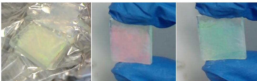
**Figure 115** Photos of opal templates deposited on TiO<sub>2</sub> coated (screen printed) FTO via the stacking of four monolayers of 595 nm PS beads (viewed from various angles).
