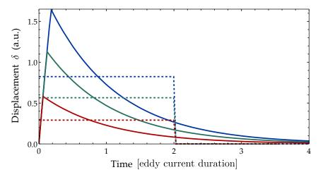
Figure 3.9: Excitation ramp. Solid lines show the time evolution of the displacement  $\delta$  induced by the magnetic bias, the rise and fall duration of which is set by eddy currents. Increasing the control duration (from black to blue) actually increase the amplitude reached by the displacement  $\delta$ . We approximate those kicks by step functions of constant duration  $\tau$  and increasing amplitude, shown in dashed lines.
