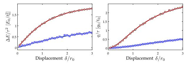
Figure 3.12: Energy increase  $\Delta E$  (left) and momentum q (right) gained by the cloud after duration  $\tau$  in a potential displaced by  $\delta$  along the  $\mathbf{x}$  direction (blue) or  $\mathbf{z}$  direction (red). Axes are scaled in dimensionless units. Data points are coming from numerical simulations with  $10^5$  particles, solid lines are given by eq (3.38) and eq (3.31) respectively, without free parameter.
