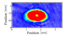
Figure 2.12: *In situ* picture of a  $^{40}$ K cloud in a plugged quadrupole trap. Notice the depletion of atoms in the center of the distribution. The RF evaporation has been pushed to  $T_{\rm cut} = 100 \, \mu \text{K}$ , further than in a normal operating sequence, to reduce the size of the beam and help with the plug alignment.
