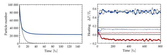
Figure 4.6: **Left**: Remaining atom number as a function of time, after a unit kick with  $\tilde{h}=1$ . Losses are defined by the passage through a death-circle in momentum space (4.46). The steady value is close to 22 500 particles and decreases by less than 2% between  $t=100\,t_0$  and  $t=1000\,t_0$ . The initial decay, fit by an exponential (black line) corresponds to a rate of  $\sim 0.2$  per time unit, within the order of magnitude expected by the Klein-Majorana loss rate (4.19).
