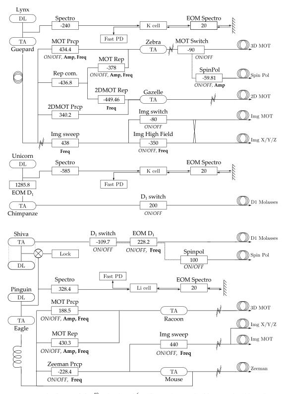
Figure 2.3: Logical scheme of the  $^{40}$ K (top) and  $^{6}$ Li (bottom) optical tables. Analog (digital) controls over the system are written in bold (italic) font. Optical sources are pictured with rounded box and AOM - EOM are represented with rectangular boxes and the corresponding frequency modulation is indicated in MHz. When relevant, the  $0^{th}$  order of an AOM is picture in dashed line. See annex A.5 for technical details. Zig-zag lines represent mechanical shutters.
