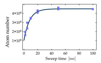
Figure 5.6: Rabi frequency measurement for  $V_{pp}=0.2$ . We fit  $N(t)=N_0\left(1-\exp(-2\pi\Omega_R^2\frac{t\,[\mathrm{ms}]}{100\,[\mathrm{kHz}]}\right)$  and estimate  $\Omega_R=0.55\,\mathrm{kHz}\pm0.04$ .
