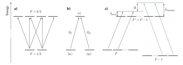
Figure 2.7: The energy levels and transitions resulting in the light shifts presented in Fig. 2.6. The standard bright Sisyphus effect is described with structure (a) while the simple  $\Lambda$  system (b) gives rise to a gray molasses. For  $^{40}K$  and  $^6Li$ , both intra- and inter-hyperfine transitions must be taken into account (c). The Raman detuning  $\Delta$  plays an important role in the cooling efficiency, as shown in figure 2.8.
