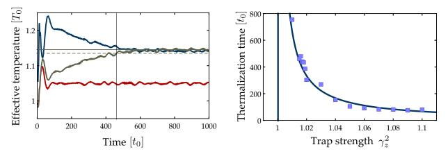
Figure 3.20: **Left**: the thermalization time is estimated as the duration after which the unexcited direction **y** reaches its final value  $T_y = T_x$ . **Right**: Thermalization time as a function of the anisotropy factor  $\gamma_z^2$ . The solid line given by the best hyperbolic fit  $t = \frac{6.67}{\gamma_z^2 - 1} t_0$ .
