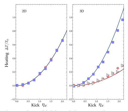
Figure 3.18: Heating as a function of the kick strength after an excitation along  $\mathbf{x}$  in an isotropic 2D trap (left) and 3D trap (right). Temperatures are given along  $\mathbf{x}$  (blue squares),  $\mathbf{y}$  (gray triangles) and  $\mathbf{z}$  (red circles). Points are obtain by numerical simulation over 10 000 particles. Solid lines are given by equations (3.50) and (3.62a-3.62b) with  $\Delta E = q^2/2m$  without any free parameter.
