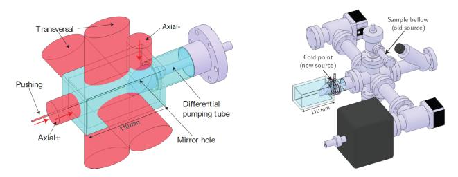
Figure 2.5: Schematics of the 2D-MOT
