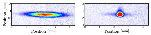
Figure 2.13:  $^{40}$ K in the optical dipole traps. (**Left**):  $7 \times 10^6$  atoms at 2  $\mu$ K after 5 ms time-of-flight from the single arm ODT. (**Right**):  $4 \times 10^6$  atoms at 1.2  $\mu$ K after 5 ms time-of-flight the crossed ODT.
