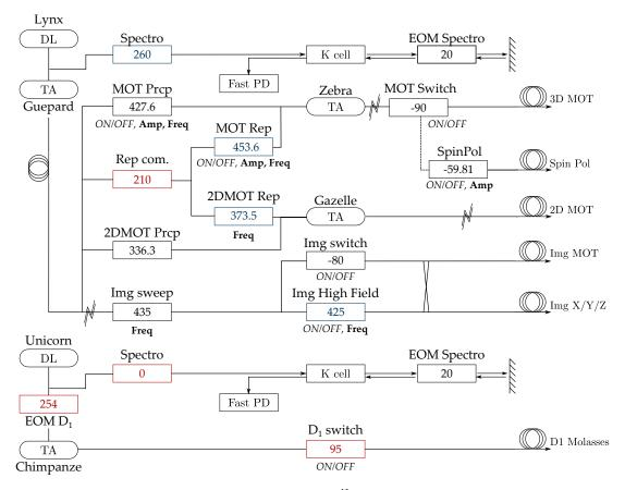
Figure 2.4: Adaptation of the potassium optical table  $^{41}$ K. For most AOM, it is sufficient to change the driving frequency. For some AOM (in blue), the order must be changed with respect to  $^{40}$ K setup. Some AOM (in red) must be removed or changed for a model with resonant frequency close to 100 MHz (rempumper commun and  $D_1$  setup).
