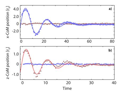
Figure 3.5: Center-of-mass oscillations of the Lithium cloud after a kick along  $\mathbf{z}$  (a) and  $\mathbf{x}$  (b). Blue squares (resp. red circles) are experimental data along  $\mathbf{x}$  (resp.  $\mathbf{z}$ ). Solid lines are exponentially damped sinusoidal oscillations. Damping results solely from dephasing of single particle trajectories. Here,  $r_0 = k_B T/\mu_B b \sim 0.6$  mm and  $t_0 = \sqrt{mk_B T}/\mu_B b \sim 1$  ms.
