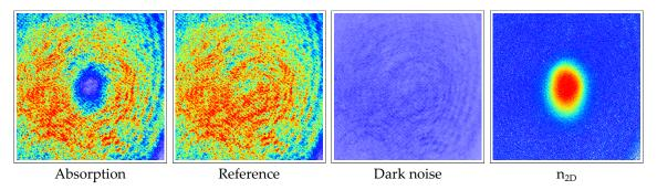
Figure 2.14: Raw and treated data from absorption imaging after 5 ms TOF. On the picture,  $\sim 10^7$   $^{40}$ K atoms after the optical molasses.
