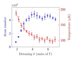
FIG. 9. (Color online) Number of atoms captured in the  $^6$ Li  $D_1$  molasses (circles) and their temperature (triangles) after a 3-ms capture phase at a high intensity,  $I_{\rm cool}=14.6I_{\rm sat}$ , as functions of the global detuning  $\delta=\delta_{\rm cool}=\delta_{\rm rep}$ . The number of atoms in the compressed MOT is  $8\times10^8$ .
