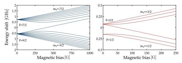
Figure A.2: Zeeman shift of the  $S_{1/2}$  manifold of  $^{40}$ K (left) and  $^{6}$ Li (right) as a function of the magnetic field, as estimated by the Breit Rabi formula (A.15)
