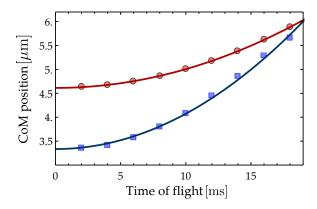
Figure 5.9: Calibration of the imaging magnification along  $\mathbf{x}$  (blue) and  $\mathbf{y}$  (red). We record the raw position (position in pixel  $\times$  size of a pixel) as a function of time and fit a parabola  $x(t) = x_0 + a_0t^2/2$ . The magnification is estimated as  $m = a_0/g$ . Here, we obtain m = 1.59 for the imaging system along  $\mathbf{x}$  and m = 0.6 for the imaging system along  $\mathbf{y}$ .
