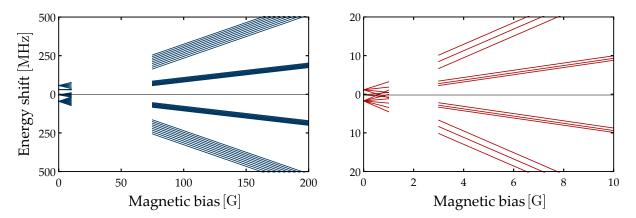
Figure A.1: Asymptotic regimes for the Zeeman shift of the  $P_{3/2}$  states of  $^{40}$ K (left) and  $^{6}$ Li (right) as a function of the magnetic field. The low field regime is given by equation (A.9), where the coupling to the magnetic field is treated perturbatively. The high field regime is given by equation (A.11b), where the hyperfine structure is estimated as a perturbation.
