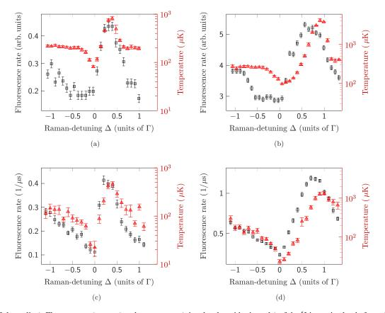
FIG. 2. (Color online) Fluorescence (squares) and temperature (triangles; logarithmic scale) of the  $^6$ Li atomic cloud after a  $100-\mu s$  pulse of  $D_1$  light with variable Raman detuning  $\Delta$ . Experiment: (a) low intensity; (b) high intensity. Simulation: (c) low intensity; (d) high intensity. Experimental and simulation results (a, c) for  $I_{cool} = 2.7I_{sat}$ ,  $I_{rep} = 0.13I_{sat}$  and (b, d) for  $I_{cool} = 9I_{sat}$ ,  $I_{rep} = 0.46I_{sat}$  per beam.
