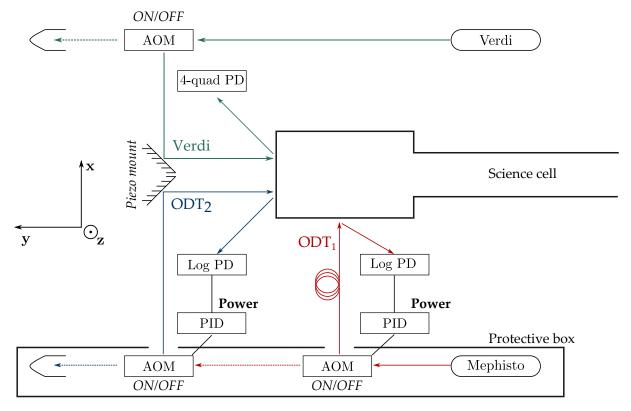
Figure 2.11: High power lasers close to the science cell. The setup is described in the main text and performances are detailed in table 2.9. We introduce directions  $\mathbf{x}$  (along ODT<sub>1</sub> beam),  $\mathbf{y}$  (along transport) and  $\mathbf{z}$  (opposed to gravity).
