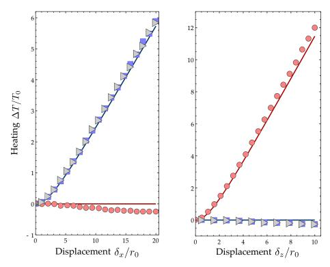
Figure 3.14: Heating after adiabatic displacement along x (left) and z (right). Results from numerical simulations over  $10^4$  particles. Solid lines are given by (3.44-3.43) and the energy redistribution (3.27), without any free parameter.
