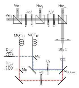
FIG. 7. (Color online) Optical scheme of the  $D_1$  molasses. The 3D MOT light and the  $D_1$  cooling light are superposed using a D-shaped mirror ( $M_{\rm D}$ ). Afterwards a dichroic mirror ( $M_{\rm dichroic}$ ) combines the lithium and potassium light, which is subsequently expanded and distributed to the three perpendicular axes of the 3D MOT.
