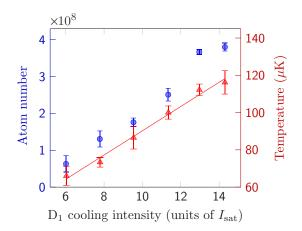
FIG. 10. (Color online) Number of atoms captured in the  $^6$ Li  $D_1$  molasses (circles) and their temperature (triangles) as functions of the  $D_1$  cooling beam intensity for  $\delta_{\rm cool} = 4~\Gamma$  and  $I_{\rm rep} = I_{\rm cool}/20$ . The number of atoms in the compressed MOT is  $8 \times 10^8$ . The atom number (temperature) increases linearly with a slope of  $4 \times 10^7$  atoms/ $I_{\rm sat}$  (6.5  $\mu$ K/ $I_{\rm sat}$ ).
