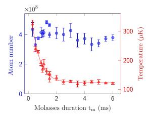
FIG. 8. (Color online) Number of atoms captured in the  $^6$ Li  $D_1$  molasses (circles) and their temperature (triangles) as functions of the molasses duration, with a 1/e cooling time constant  $\tau_{\rm cool} = 0.6$  ms. The number of atoms in the compressed MOT is  $8 \times 10^8$ .
