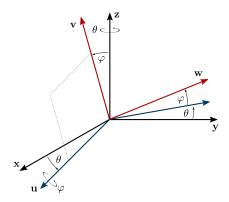
Figure 3.17: Introducing the coordinate system. We introduce the basis  $(\mathbf{u}, \mathbf{v}, \mathbf{w})$ , derived from the Cartesian coordinates with two rotations  $\theta$  and  $\varphi$  such that the motion of the particle remains in the  $(\mathbf{u}, \mathbf{v})$  plane.
