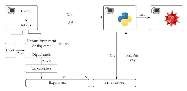
Figure 2.15: Computer control of the experiment. The type of information exchanged between the elements is written in italic font. The electronic boards for the optocoupler box are presented in annex A.6.
