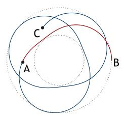
Figure 3.16: Trajectories in a linear potential. We first consider a trajectory starting at point  $A = (r_0, \theta_0, p_{r_0}, L_z)$ . The first perihelion of this trajectory is B. We now consider a second trajectory, starting at point  $C = (r'_0, \theta'_0, p'_{r_0}, L_z)$  with the same energy and orbital momentum. We show that this second trajectory will come arbitrarily close to point B, meaning that the two trajectories are one and the same.
