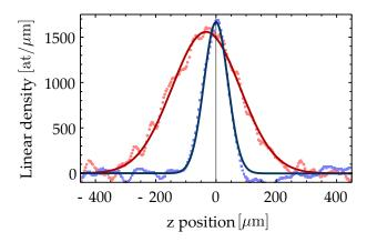
Figure 5.15:  $4.5 \times 10^5$  Lithium atoms (in red) and  $1.9 \times 10^5$  Potassium atoms (in blue) at  $\sim 38~\mu K$  in the optical dipole trap at the end of the RF evaporation, after 0.5 ms TOF.
