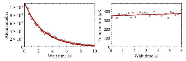
Figure 3.1: Time evolution of a Lithium cloud trapped in the quadrupole trap.**Left**: the atom number decays exponentially, with a lifetime  $\sim 2.8$  s limited by the background pressure. **Right**: simultaneously, the temperature T slowly increases, with a heating rate estimated by a linear regression to  $5.1 \pm 2.1 \,\mu\text{K/s}$ . Here, we plot  $m\sigma^2/k_B t_{TOF}^2 \propto T$ , where  $\sigma$  is the measured width of the distribution after time-of-flight  $t_{TOF}$ .
