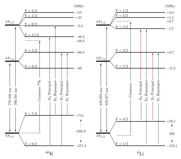
Figure 2.2: Energy levels of lithium and potassium. Note that <sup>40</sup>K has an inverted hyperfine, rendering its magnetic trappping easier. Values are taken from [Gehm 2003] and [Tiecke 2010].
