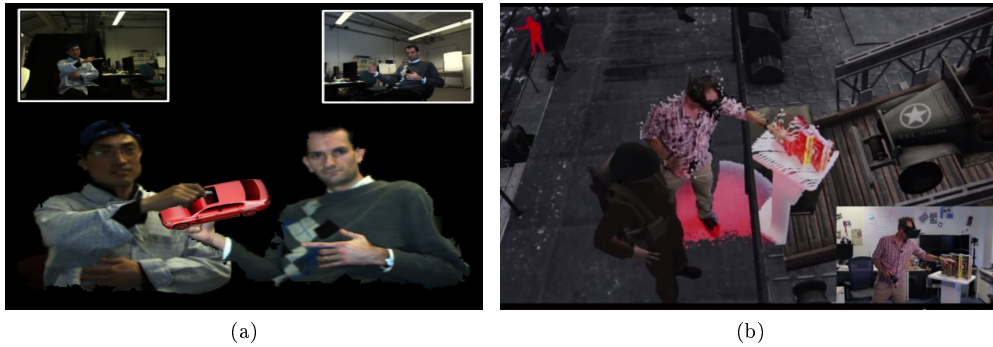
FIGURE 2.9 – Two examples of AV applications. These two examples present how real objects can be injected into a VE. (a) Vasudevan et al. [Vasudevan et al., 2010] represent a 3D reconstruction of the upper bodies of two distant users into a shared VE. (b) "Never Blind VR" [Nahon et al., 2015] represents in the VE some elements from the real world such as close obstacles or other people in the room.
