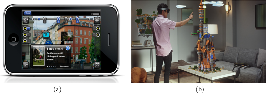
FIGURE 2.7 – Two examples of AR applications. These two examples mix a real world with virtual information (a) Contextual virtual information is superimposed over the real world with Junaio AR View. (b) The virtual world is composited with the real world. Here a virtual "castle" is displayed on the table.
