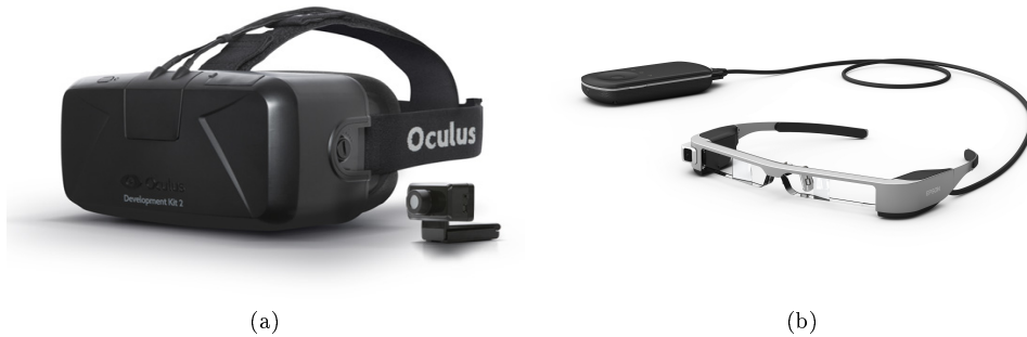
FIGURE 2.14 – Two examples of visual display devices used for MR user interfaces. (a) The Oculus Rift DK2 is an HMD used for VR applications that provides a 100^\circ horizontal field of view and a 360^\circ FOR with a positional and rotational tracking. Its resolution is 960 \times 1080 pixels per eye. (b) The Epson Moverio BT-300 is an example of see-through glasses used for AR applications. It provides a 23^\circ diagonal FOV and depending on the tracking technology used can provide a 360^\circ FOR.
