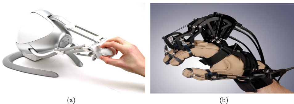
FIGURE 2.15 – Two examples of haptic output devices. (a) The Novint Falcon is a ground-reference haptic device that can apply force on the 3 axis of translation. (b) The Cybergrasp glove is a body-referenced haptic device that can apply forces on each finger in order to prevent the user's fingers from penetrating into a solid virtual object 2.15b.
