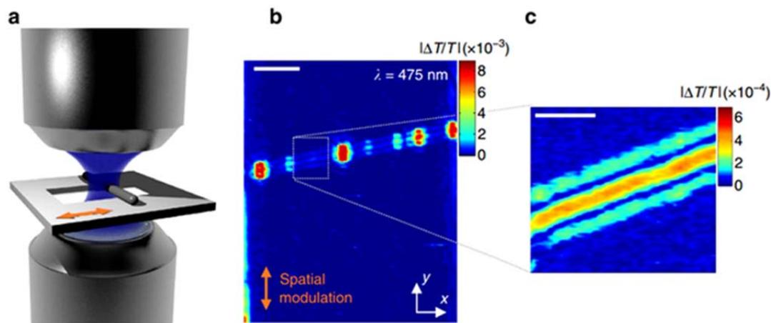
**Figure A.5:** Absorption-based imaging of SWNTs. (a) Sketch of the SMS technique showing the double microscope system and the sample. The position of the sample is periodically modulated at frequency  $f$  (orange arrow) and the transmitted beam power is synchronously detected at  $2f$ . (b) Transmission SMS image,  $|\Delta T/T(x,y)|$ , of a region of the trench showing the free-standing (22,6) individual semiconducting SWNT. (c) Zoom on a clean section of this nanotube (adapted from [95]).
