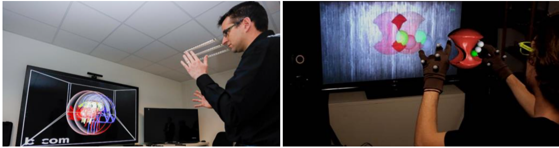
Figure 1.8: Illustrations of mid-air bimanual interaction schemes in semi-immersive systems. (Left) A virtual carousel with symmetric 3D object manipulation inspired from work presented by Gaucher et al. [Gaucher et al., 2013]. (Right) A virtual design application [Le Chénéchal et al., 2014b] based on an asymmetric control scheme.
