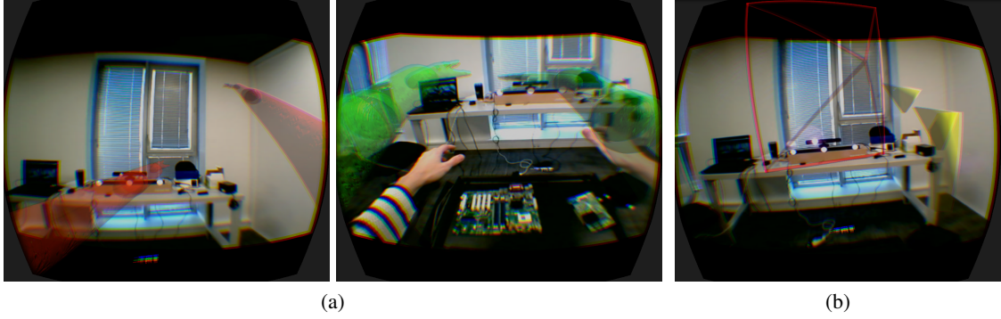
Figure 3.26: (a) The stretchable guiding arms, controlled by the remote expert's location, from the agent's viewpoint. On the left, the arms are extended and red because the guide is ahead of the agent. On the right, the agent has reached the guide's location and the guiding arms retrieve their initial length and green color. (c) A simple guiding technique based on directional arrows and viewing frustum of the remote expert.
