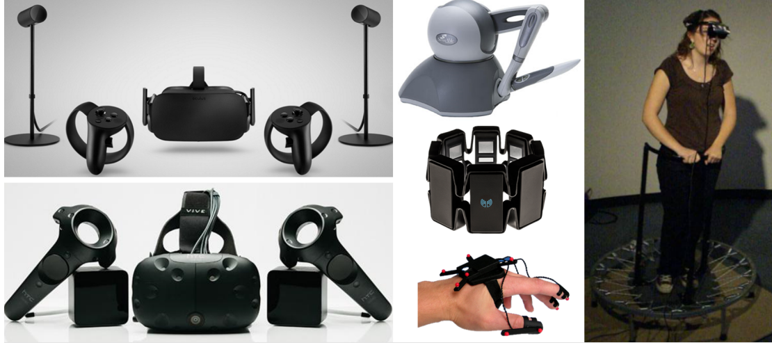
Figure 1.4: (Left) The Oculus Rift CV1 and the HTC/Valve Pre Vive, with their controllers and tracking system, available on the consumer market. (Middle) The Omni PHANTOM desktop haptic arm, the Myo device for hand tracking, the finger tracking system based on ART. (Right) the Joyman device [Marchal et al., 2011] for navigation.
