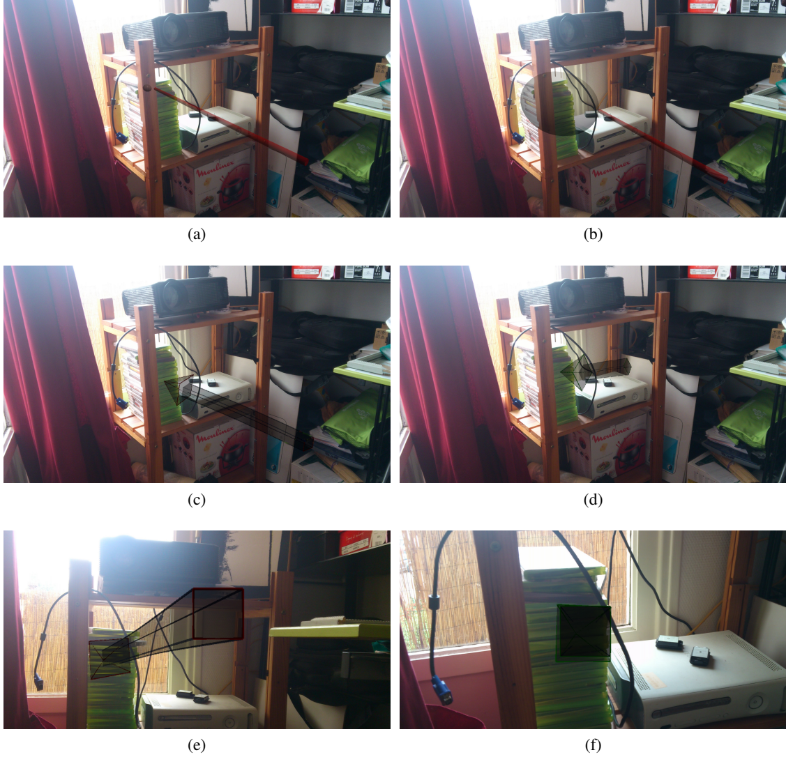
Figure 3.10: Illustration of the static mode for navigation guiding. (a), (b), (c) and (d) are exocentric PoVs from the agent's workspace used to explain the expert interactions, while (e) and (f) are actual screenshots of the agent's display. First, the expert defines a virtual sphere using the 3D ray in (a) and (b). Then, the system computes the location of the two final control points using the sphere as bounding volume and the ray for their respective orientation in (c) and (e). Last, on (d) and (f), the agent reaches the correct spot pointed by the navigation technique; it has been computed in a way that the camera FoV, worn by the agent, contains the initially defined spherical bounding volume.
