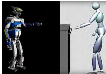
Figure 5.5: The result of the re-targeting of the drawer opening task onto the unconstrained skeleton of the HRP-2 robot. The movie is available here [ http://tinyurl.com/j8qnbtp ]
