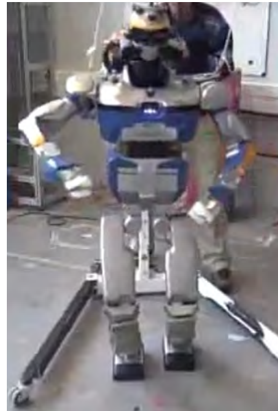
(b) Real HRP-2 robot performing walking-reaching sequences.
