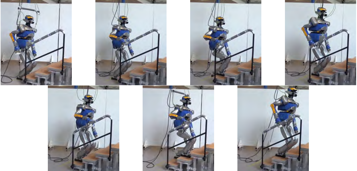
Figure 2.3: Set of contact stances realized by the humanoid robot HRP-2 using the method proposed in this chapter. The experiment has been realized 5 times in a row without failure. The accompanying video shows the realization of the experiments.
