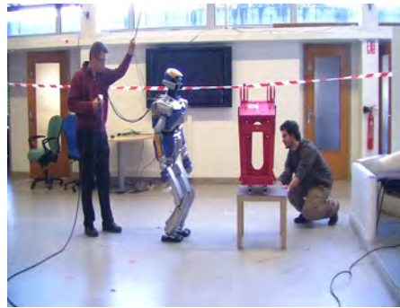
Figure 6.2: Robot tracking the engine pylon using a motion capture system
