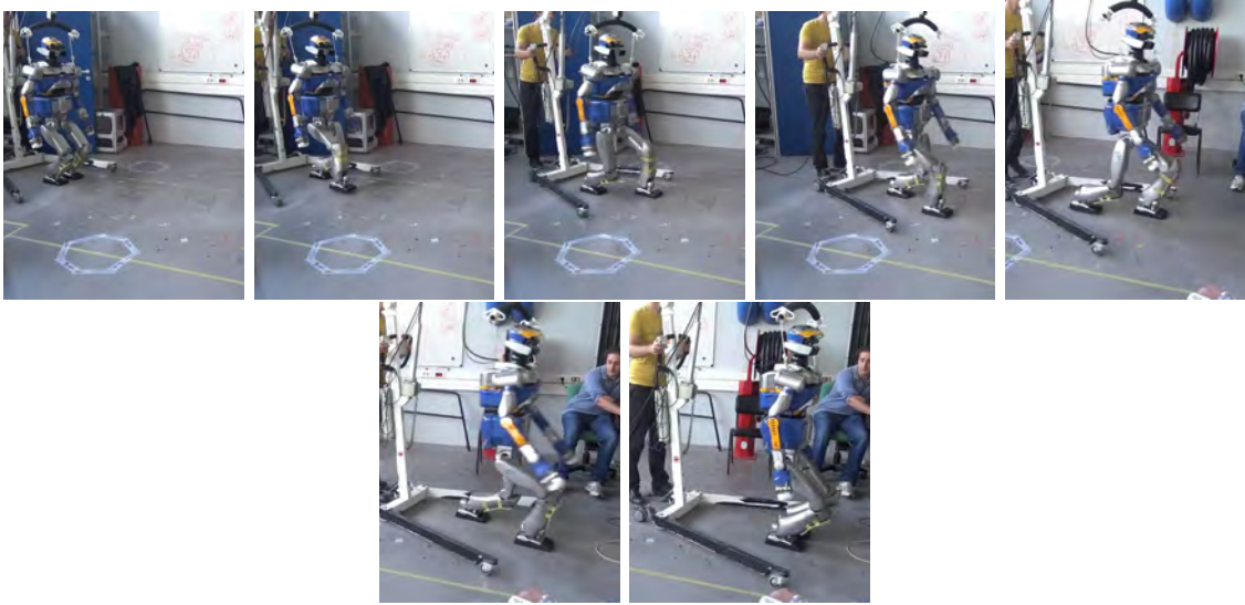
Figure 2.7: Experiment 1: Walking in straight line with enjambment of 100cm.
