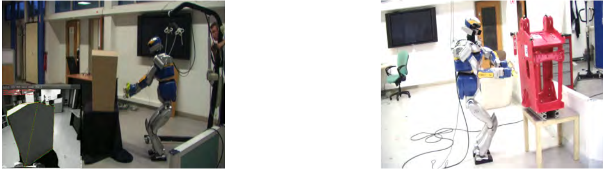
Figure 6.3: HRP-2 doing a whole body screwing motion holding a 3D printed industrial screwdriver. On the left side one can see the visual servoing done on a mockup of the engine pylon. On the right side the robot is controlled via motion capture data as the visual servoing did not work on the 3D printed engine pylon.
