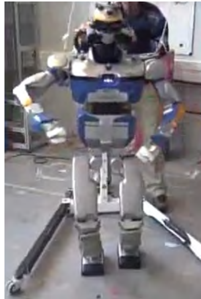
(b) Real HRP-2 robot performing walking-reaching sequences.
