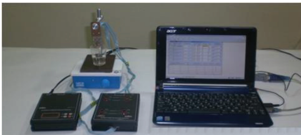
Figure 9. Photograph of the working area, presenting the conductometric device, the working cell with the transducer, and the computer.
