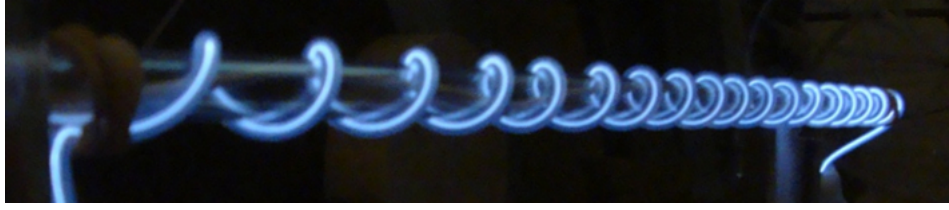
Figure 5.5: Photograph of the pulsed corona discharge propagating in argon gas inside an 2 mm inner diameter silicone tube over 105 cm between a source (a tungsten needle) and a counter electrode.
