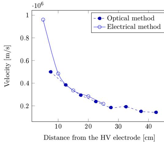
**Figure 5.9:** Discharge instantaneous velocity of propagation in argon with water vapor (calculated from a fit of the data of Figure 5.8) and compared to the velocity in argon with water vapor obtained from electrical measurement (data from Figure 5.4).
