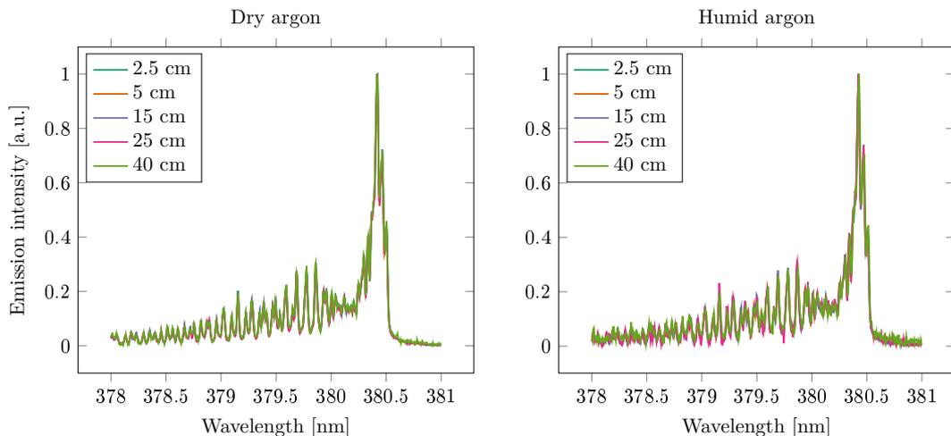
**Figure 5.11:** Optical emission spectra of the  $\text{N}_2$  second positive system between 378 and 381 nm (0-2 band) measured at various locations (2.5, 5, 15, 25, and 40 cm from the needle electrode, overlaid) along the quartz tube in dry argon and humid argon (760 ppm  $\text{H}_2\text{O}$ ).
