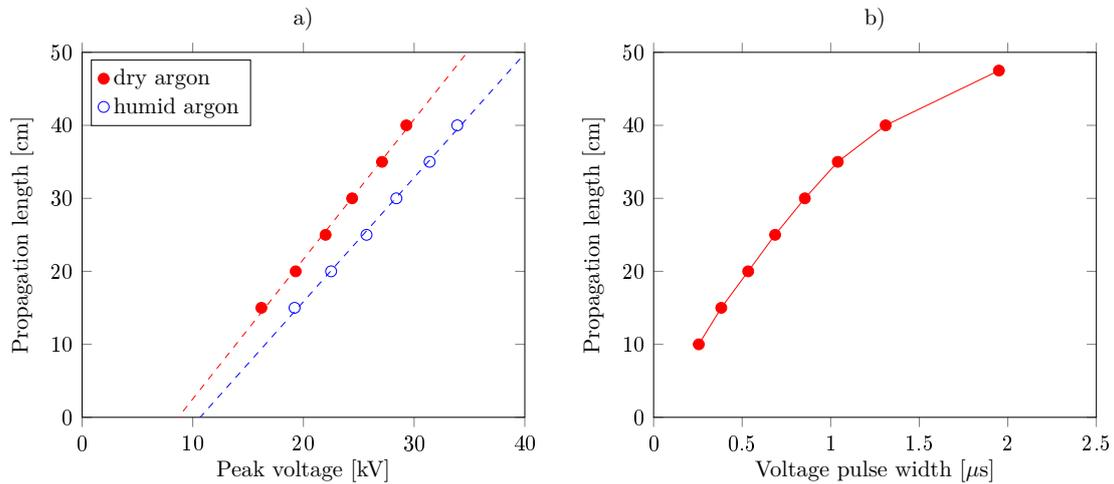
**Figure 5.3:** Pulsed corona discharge electrical characterization. (a) Discharge propagation length at constant pulse width (700 ns) for increasing peak voltage in humid argon (4.7 slm, blue symbols), and dry argon (3.9 slm, red symbols) with linear fits (dashed lines). (b) Discharge propagation length at constant peak voltage (23.3 kV) for an increasing pulse width in dry argon.
