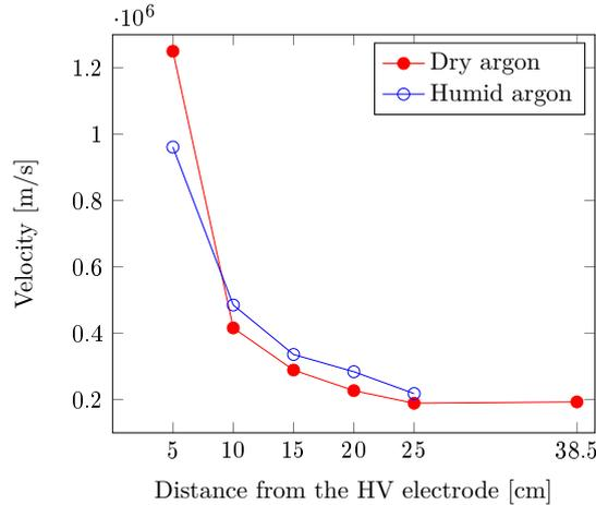
**Figure 5.4:** Dependence of the streamer velocity in dry and humid argon on the distance from the HV electrode measured by the movable probe. The discharge settings (flow rate and applied HV) were the same as for biological experiments
