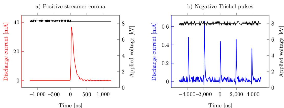
**Figure 4.4:** Voltage and current waveforms for a) Positive streamer corona, frequency of pulses 13 kHz, b) Negative Trichel pulses, frequency of pulses 473 kHz (current and voltage values were inverted, the supplied voltage and formed pulses were negative).
