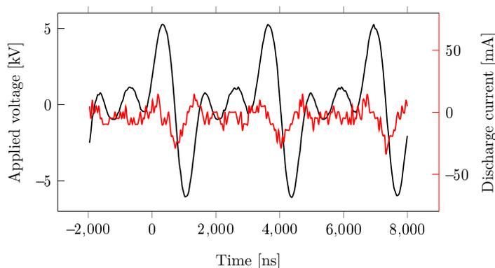
**Figure 6.2:** Waveform of the dielectric barrier discharge inside the argon jet. The high voltage development over time (—) and time development of the electric current measured on the grounded copper electrode (—), frequency of pulses is 30.2 kHz.
