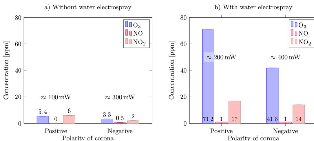
**Figure 4.5:** Concentration of O<sub>3</sub> measured by the homemade ozone analyzer, and NO and NO<sub>2</sub> measured by the commercial gas analyzer in artificial air (20% O<sub>2</sub>, 80% N<sub>2</sub>), 15 min accumulation in the zone with the DC corona discharges with or without water electro spray. The mean power of every experimental setup is indicated above the bars.
