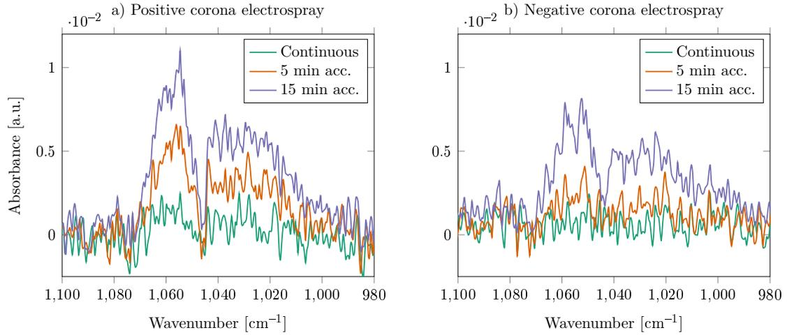
**Figure 4.7:** Examples of  $O_3$  FTIR spectra formation in time in a) positive corona with electro-spray, and b) negative corona with electro-spray. Continuous measurement in air flowing through the discharge chamber, 5 and 15 min gas accumulation inside the chamber and then spectra measured.
