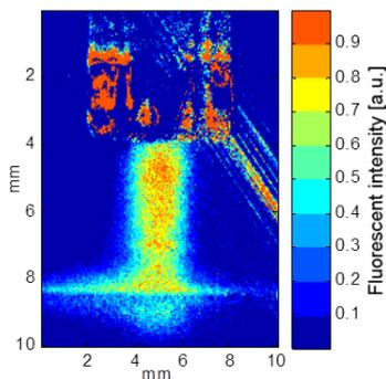
**Figure 6.4:** Indirect exposure of biological samples to the plasma jet. OH-PLIF of the jet fed by saturated argon, the fluorescence intensity (color scale) linearly corresponds to the concentration of OH radicals (Measured by Florent Sainct, CentraleSupélec).
