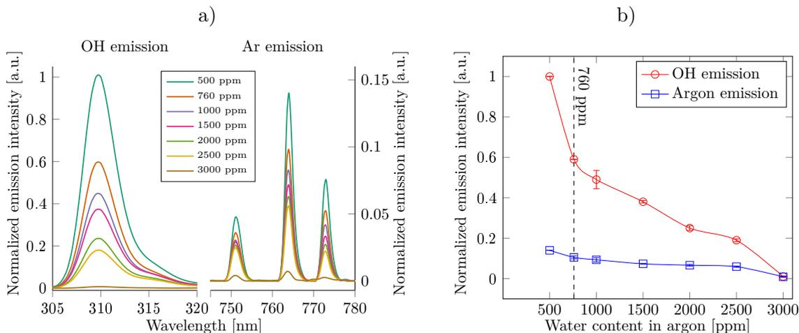
**Figure 6.3:** Optical emission spectroscopy of argon jet with varying water vapor content. a) Normalized emission spectra of OH (305 – 320 nm) and argon emission (745 – 780 nm) intensity dependence on water content in argon gas. b) Dependence of OH and argon emission maxima on water content in argon (normalized, average of two experiments). Electrical parameters for humid argon were kept constant during the whole experiment.
