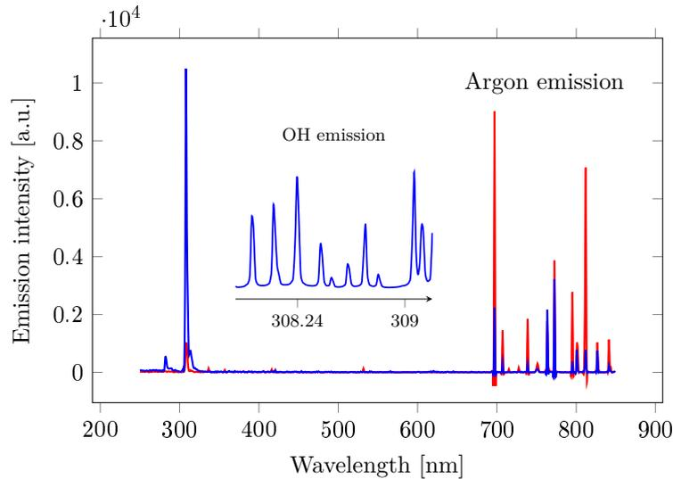
**Figure 5.6:** Optical emission spectra of the pulsed corona discharge in dry (red line) and humid argon (blue line) acquired at 5 cm from the HV electrode. Detector integration time 600 ns, grating 300 lines/mm. The insert represents a spectrum of the rotational bands of  $\text{OH}^*[\text{A}^2\Sigma^+ - \text{X}^2\Pi]$  measured in humid argon (760 ppm water vapor), grating 2400 lines/mm.
