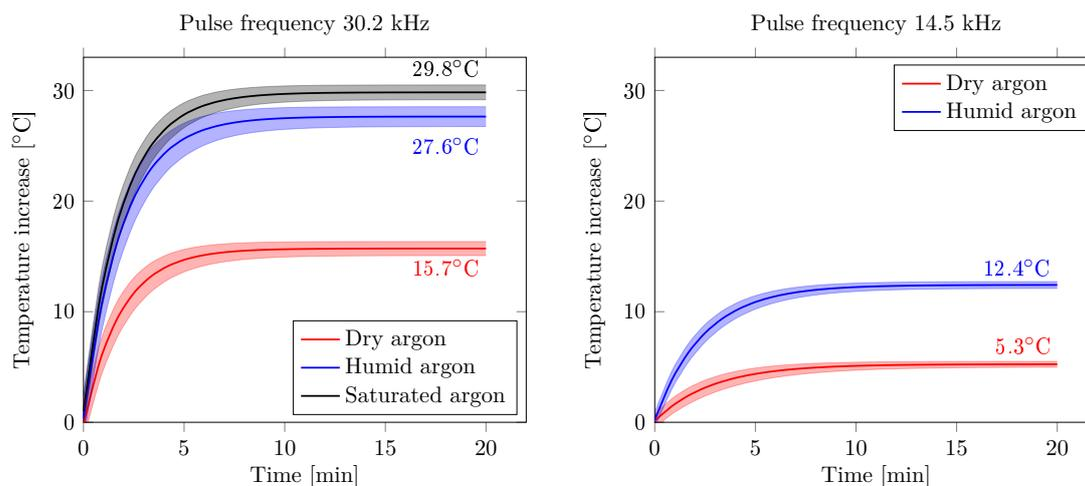
**Figure 6.5:** Temperature increase over the ambient temperature of the cover glass 1 cm from the jet nozzle in the dry, humid and saturated argon discharge. Values represent the final value of the surface temperature increase over ambient after 20 min of discharge running. The initial (ambient) temperature varies between 18 – 23°C. Frequency of HV pulses: a) 30.2 kHz, b) 14.5 kHz (fits with 95% confidence intervals).
