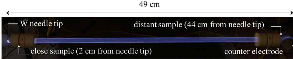
**Figure 5.1:** Photograph of the pulsed corona discharge propagating in argon gas inside an 8 mm inner diameter quartz tube over 49 cm between a charged tungsten needle and a grounded counter electrode. The bacterial sample locations at 2 and 44 cm are indicated.
