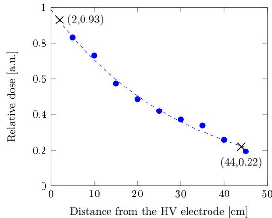
**Figure 5.10:** Relative UV-B dose (305-311 nm) per discharge event calculated for each position from the data of Figure 5.8, including the second emission maximum at 2.4  $\mu\text{s}$ . Relative dose one corresponds to the relative dose at the tip of the HV electrode.
