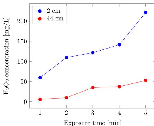
**Figure 5.17:**  $\text{H}_2\text{O}_2$  concentration at 2 and 44 cm from HV electrode produced in water droplets ( $5 \times 10 \mu\text{L}$ ) over increasing exposure times to the plasma discharge in humid argon (760 ppm  $\text{H}_2\text{O}$ ). Experiments were carried out in triplicates.
