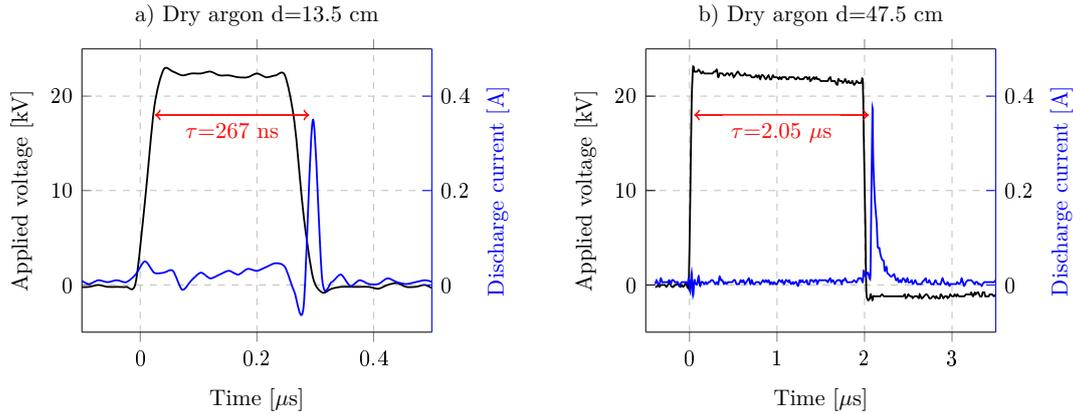
**Figure 5.2:** Voltage and current waveforms for two needle-to-counter-electrode gap distances for a discharge in dry argon gas (3.9 slm). a) Gap distance of 13.5 cm, and b) gap distance of 47.5 cm, with  $\tau$  being the delay from the voltage pulse rise to the arrival of the propagating discharge to the counter electrode.
