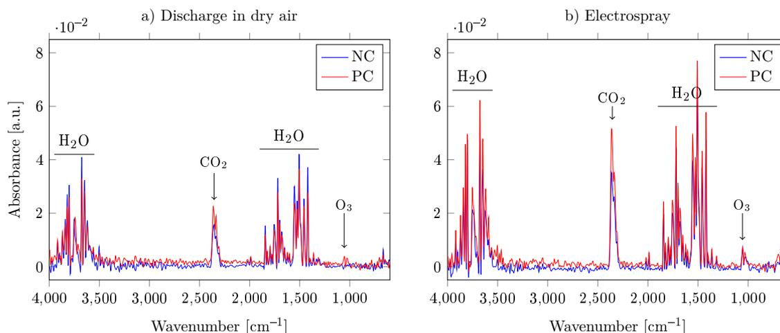
**Figure 4.6:** Examples of FTIR spectra from positive and negative corona discharge measured in a) dry air, and b) in ambient air with water electro spray. 15 min accumulation inside 1 L chamber the with the discharge running, the gas was then transferred to a vacuumated cuvette.
