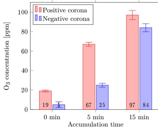
**Figure 4.8:** Ozone concentration measured by FTIR for PC and NC discharge with water electro-spray. The gas from the discharge chamber was flowing to FTIR spectrometer continuously (0 min) or was accumulated for 5 or 15 min and then the concentration was measured. The concentrations were calculated according to Equation 4.4.
