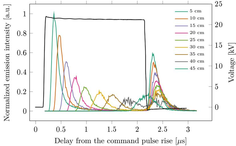
**Figure 5.8:** Excited  $\text{OH}^*[\text{A}^2\Sigma^+ - \text{X}^2\Pi]$  radicals emission (305-311 nm) relative intensity profile evolution with time for different light collecting positions along the tube (distance from the needle electrode: 5, 10, 15, 20, 25, 30, 35, 40, 45 cm) and synchronized applied voltage signal. Humid argon (760 ppm  $\text{H}_2\text{O}$ , 4.7 slm)
