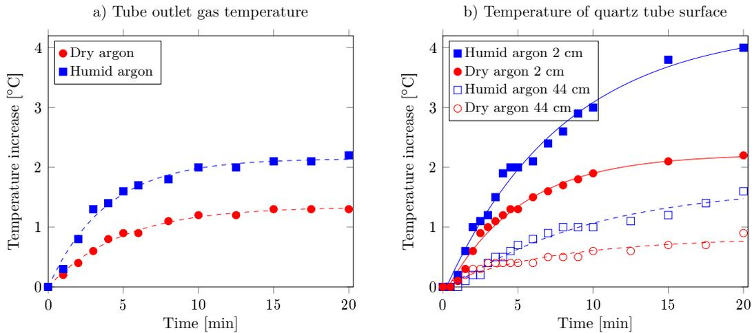
**Figure 5.12:** Absolute temperature increase over treatment times of: a) the feed gas measured at the counter electrode in dry (red) and humid argon (blue), and b) quartz tube surface at 2 (full symbols) and 44 cm (hollow symbols) from the HV electrode, with one phase exponential fits (lines).
