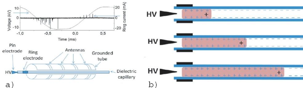
**Figure 2.2:** Plasma bullet propagation in a capillary; taken from [13]: a) The corresponding waveforms of voltage and current (measured on the ring electrode) during the negative and the positive cycle; b) The propagation of consecutive positive bullets in a capillary which is pre-charged negatively
