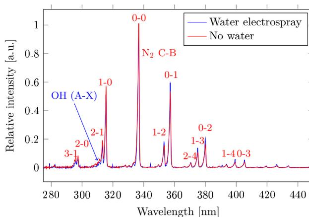
**Figure 4.20:** Emission spectra of DC corona discharges in the UV region for the positive streamer corona with water (blue curve) and without water (red curve).  $U_{\text{blue}} +12\text{ kV}$ ,  $U_{\text{red}} +16\text{ kV}$ , gap 1.5 cm, nozzle 0.6/0.8 mm inner/outer diameter, conductivity  $500\ \mu\text{S}/\text{cm}$ , water flow rate 0.4 ml/min. (Modified from the PhD Thesis of B. Pongrác [178]).
