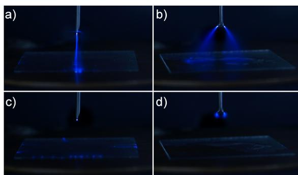
**Figure 4.2:** Photos of DC corona discharges in air with a hypodermic injection needle as a HV electrode (clipped for electro spray b, d) and a glass cover slide on a copper grounded electrode: a) positive corona, b) positive corona with water electro spray, c) negative corona, d) negative corona with water electro spray (4 s exposure time).
