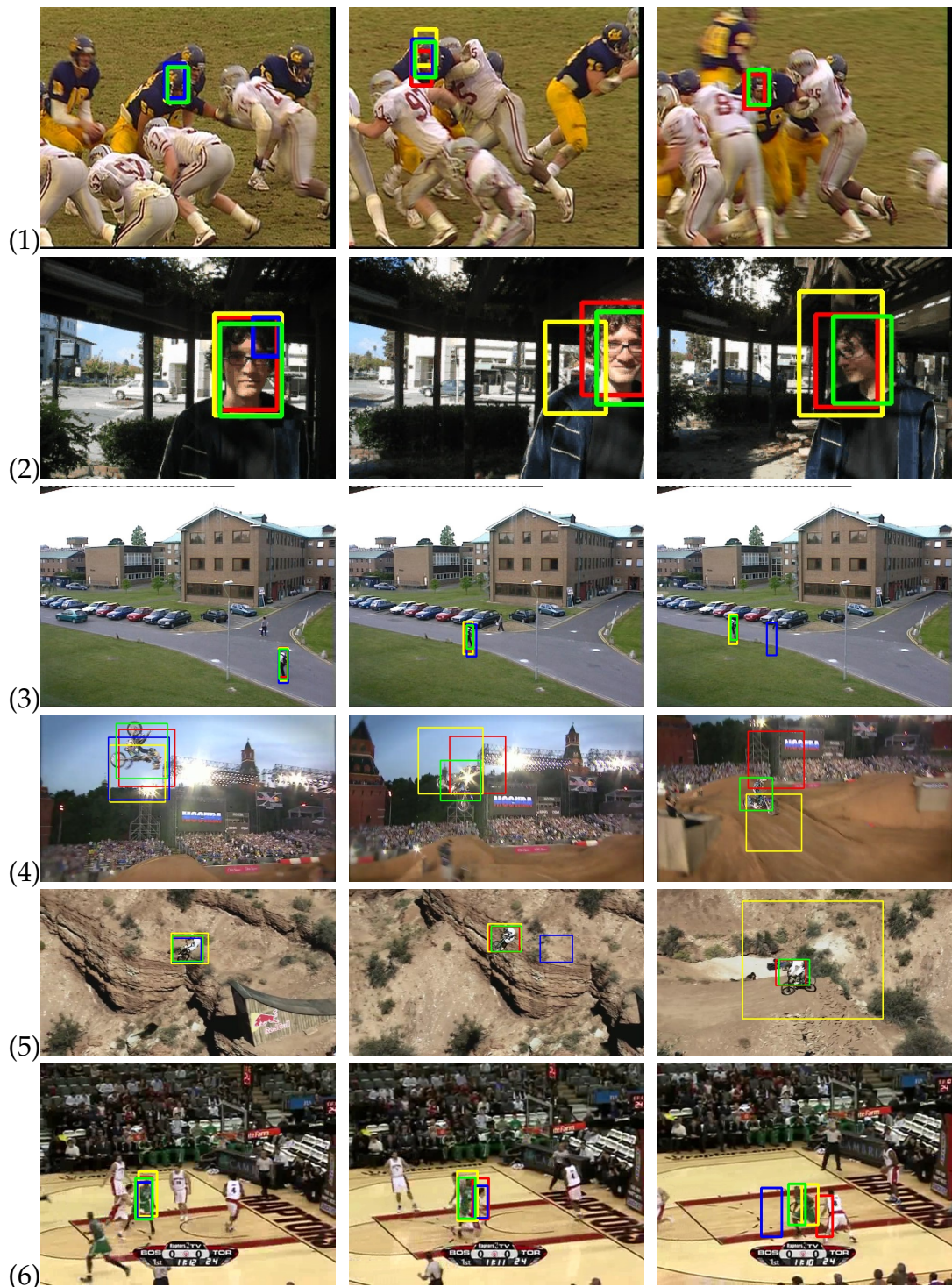
Figure 4.5 – Qualitative results on (1) Football1, (2) Trellis, (3) Walking, (4) MotorRolling, (5) MountainBike, and (6) Basketball sequences from the OTB dataset [Wu et al., 2013]. Green: Our result, Red: Struck, Blue: TLD, Yellow: SPLTT. See text for details.
