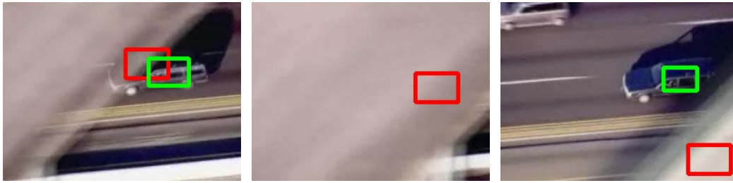
Figure 4.1 – Three sample frames from the Carchase sequence in the TLD dataset [Kalal et al., 2012]. Each image also shows the result of our method (in green) and Struck [Hare et al., 2011] (in red). As the car starts to move to a severely occluded state, updating the appearance model with the prediction result leads to model drift, as shown by the Struck result. Our proposed method estimates such states, and does not update the model in such cases.
