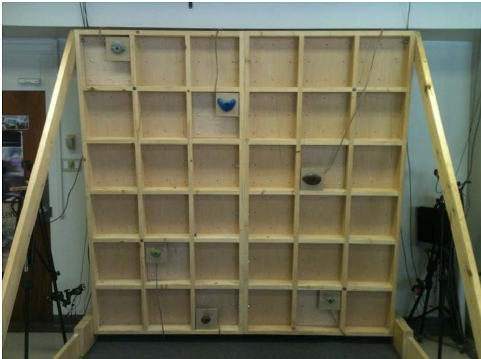
**Figure 2.1:** *The instrumented bouldering wall used for the data capture. The holds are mounted on 6D force sensors. On each side of the wall one can see the tripods on which four of the 24 OptiTrack cameras are mounted.*
