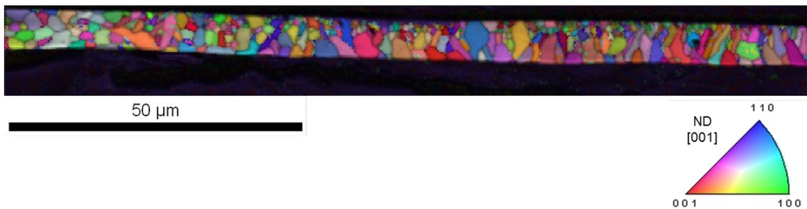
Figure 3.14: IPF+IQ map of the cross-section of a flake.
