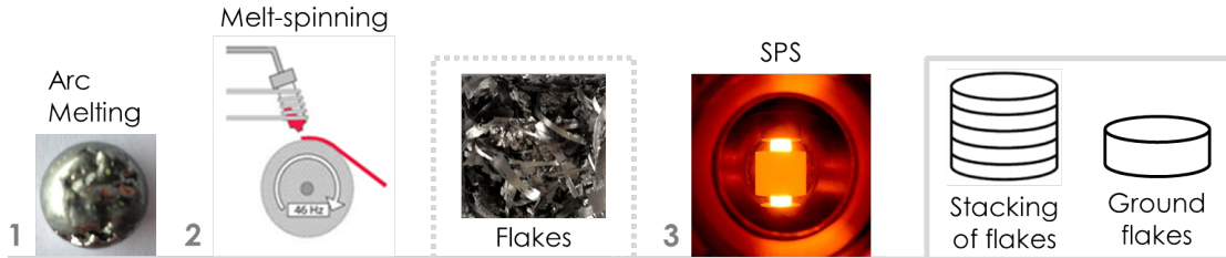
Figure 3.1: Experimental procedure for the production of isotropic and textured materials with melt-spinning process.
