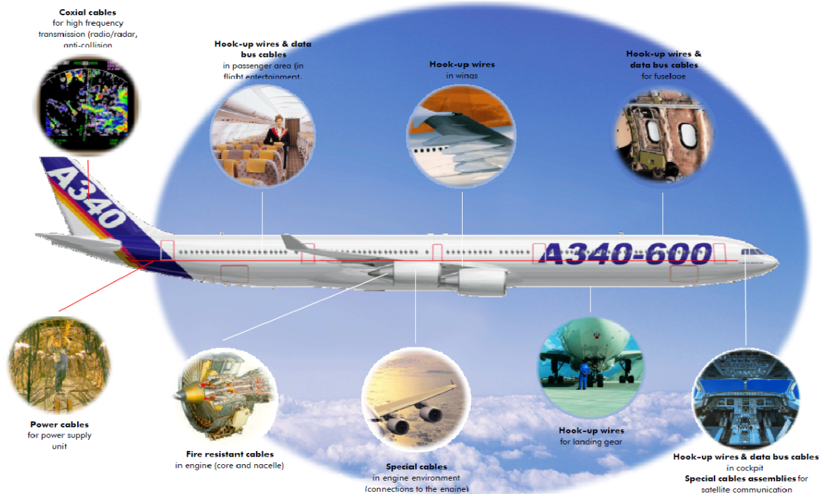
Figure 1.4 A map showing different cable types with their function in an airbus A340 aircraft. Source: [2]
