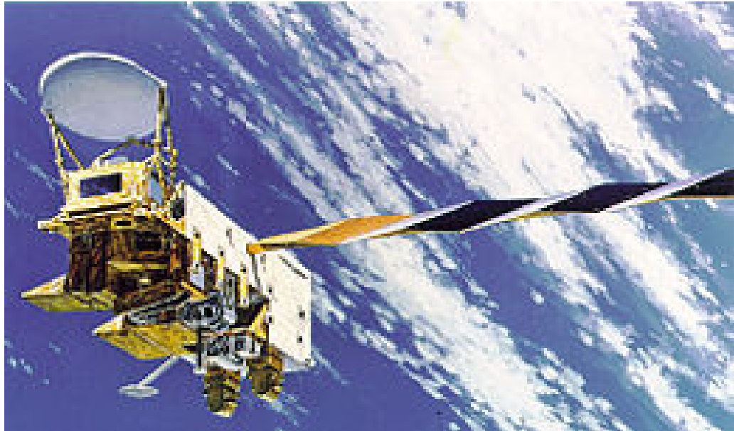
Fig. 3 - 11 AMSR-E aboard AQUA satellite. Source: [ http://aqua.nasa.gov/ ]
