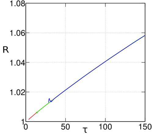
FIGURE 3 – Generic initial condition for one helical vortex  $L = 1, Re = 5000$  : three computations with different initialisations corresponding to times  $t_* = -3.125$  (red),  $t_* = -12.5$  (green) and  $t_* = -28.15$  (blue). (a) Squared core size  $a^2$  vs  $\tau$ ; the dotted black line represents the 2-D diffusion law  $a^2 = 4\tau/Re$ . (b) Radial position  $R$  of vorticity maximum versus  $\tau$ .
