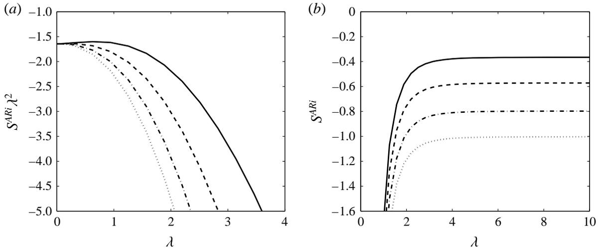
FIGURE 8. Strain rate parameter  $S^{ARi}$  for an array of vortex rings as a function of  $\lambda = L_z/R$  for various  $\epsilon = a/R$ . Solid line:  $\epsilon = 0.33$ ; dashed line:  $\epsilon = 0.1$ ; dash-dot line:  $\epsilon = 0.033$ ; dotted line:  $\epsilon = 0.01$ .
