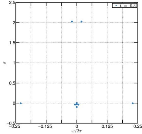
Figure 9.11 – Spectrum in the  $(\sigma, \omega/2\pi)$  plane for  $N = 3$  helical vortices with a central hub vortex at  $L = 0.3$ ,  $a = 0.09$  and  $Re = 10000$ . Only the first 9 dominant modes are shown.
