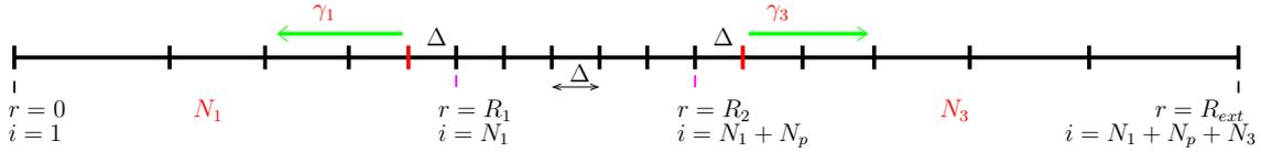
Figure 3.1 – Structure of the radial mesh used for the spatial discretisation. In the central section (indices  $i = N_1, \dots, N_1 + N_p$ ), the grid points are regularly spaced. Two regions of irregularly spaced points are represented with different contraction/expansion parameters  $\gamma_1$  for  $i = 1, \dots, N_1 - 1$  and  $\gamma_2$  for  $i = N_1 + N_p, \dots, N_r$ .
