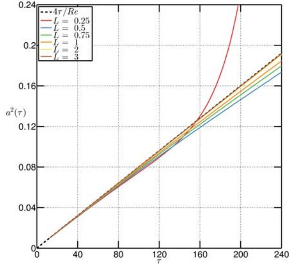
Figure 6.6 – Time evolution of the squared core size  $a^2$  for a single helical vortex at  $Re = 5000$  and different values of  $L$ . The black dashed line shows the two-dimensional diffusion law  $a^2(\tau) = 4\tau/Re$ .
