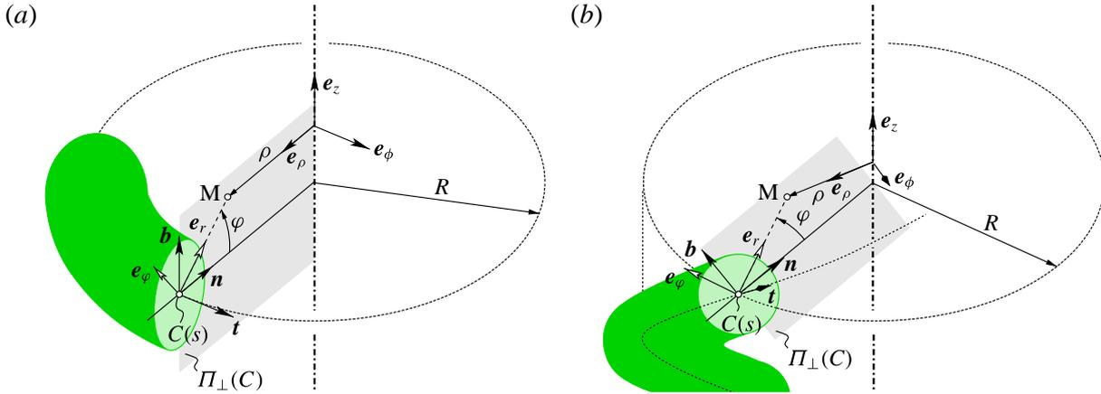
FIGURE 2. (Colour online) Illustration of the coordinate system for a ring (a) and a helix (b). The point  $M$  can be localized using the global cylindrical frame  $(e_\rho, e_\phi, e_z)$ , or the local frames: the Serret–Frenet frame  $(n, b, t)$  and the frame  $(e_r, e_\phi, t)$ . Note that vectors  $e_r$  and  $e_\phi$  are in the plane  $(n, b)$ . Point  $C(s)$  is defined as the point on the curve  $\mathcal{S}$  which is the closest to point  $M$ .
