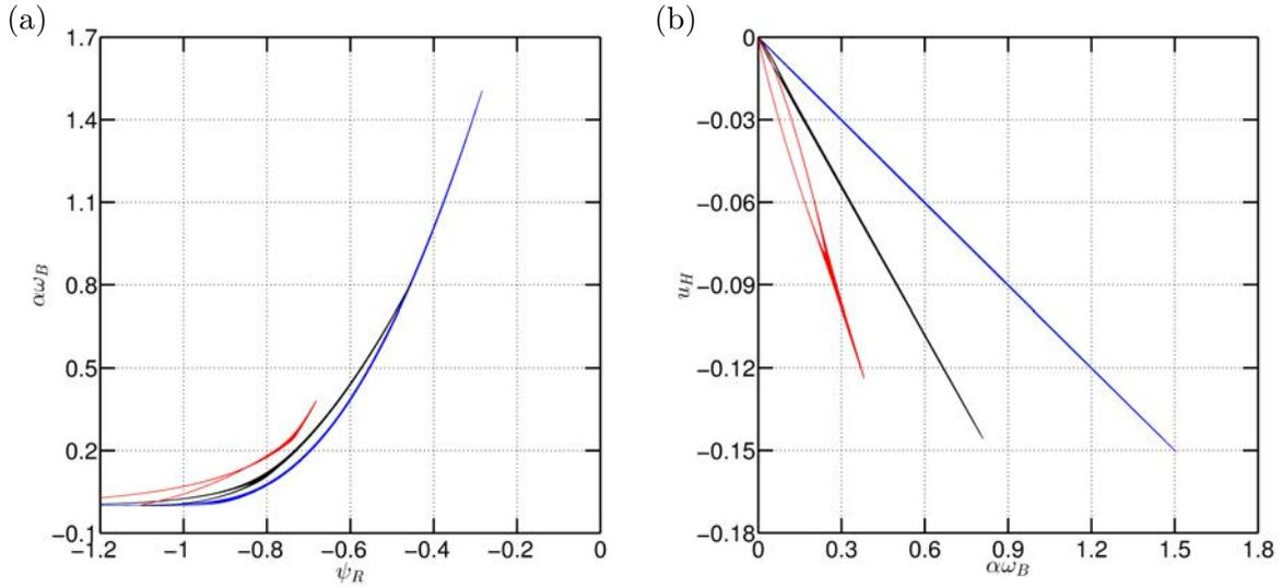
Figure 6.22 – One helical vortex of reduced pitch  $L = 0.25$  and  $Re = 5000$ . Scatter plots of the quantities  $(\alpha\omega_B, \Psi_R)$  and  $(u_H, \alpha\omega_B)$  for instant  $\tau = 62.5$  (blue), 112.5 (black), 202.5 (red).
