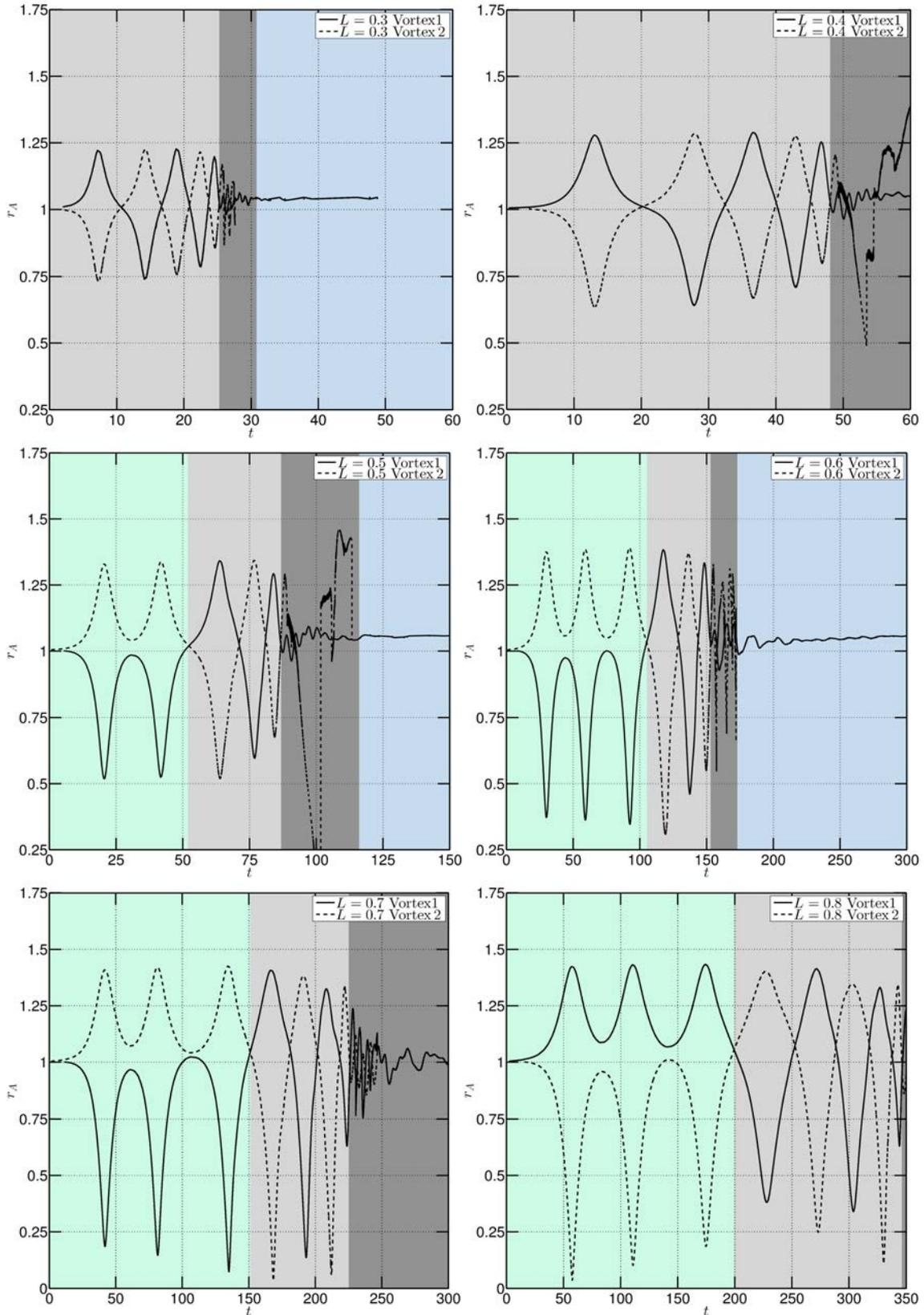
Figure 10.4 – Time evolution of the vortex centres  $r_A$  at  $Re = 10000$  for  $L = 0.3, \dots, L = 0.8$  with initial core size  $a = 0.06$ . The light grey area corresponds to the time interval where the leapfrogs occur, the light green region (when it exists) to the overtaking phase, the dark grey area to the merging instant ( $r_A$  is erroneously determined in this zone) and the blue region to the merged state.
