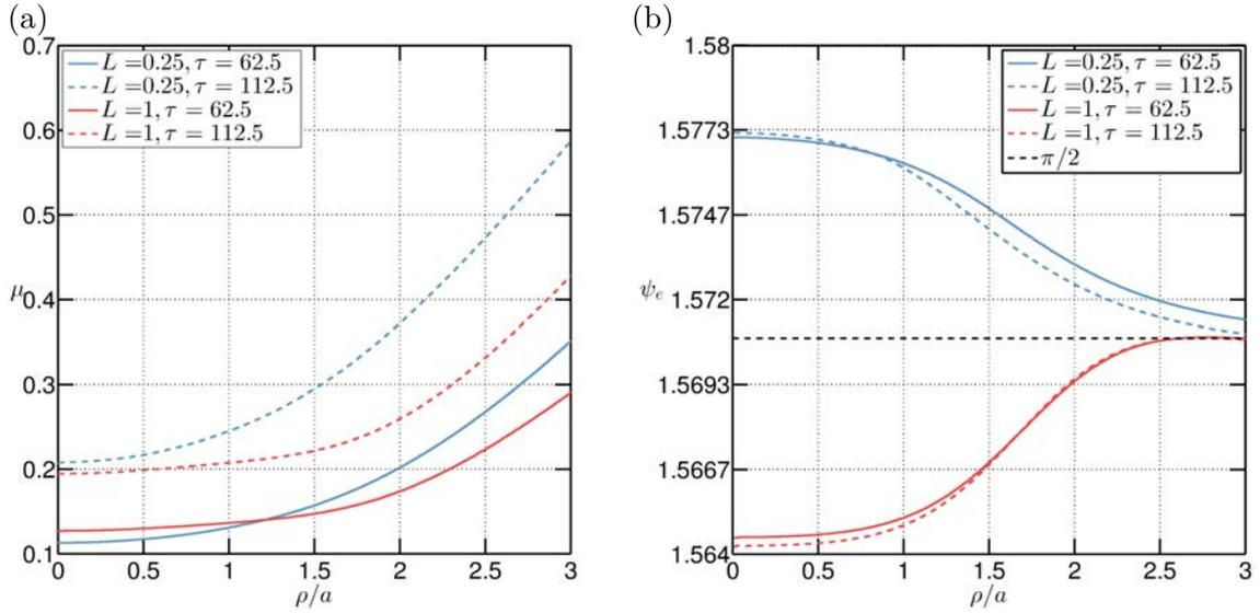
Figure 5.8 – One helical vortex of reduced pitch  $L = 0.25$  and  $L = 1$  at  $Re = 5000$ : (a) ellipticity  $\mu$  at different instants  $\tau = 62.5, 112.5$ . (b) Angle  $\psi_e$  of the major axis of the ellipse at the same instants. On both plots, the radial coordinate is made dimensionless with the core size  $a$ .
