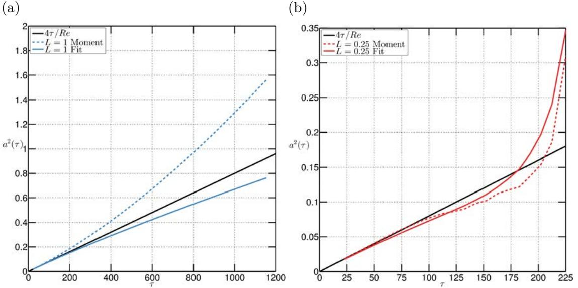
Figure 5.7 – Time evolution of the squared core size  $a^2$  for one helical vortex at  $Re = 5000$ . (a)  $L = 1$ . (b)  $L = 0.25$ . Solid: fit of the axisymmetric mode of the helical vorticity  $\omega_{BA}^{(0)}$ . Dashed:  $a_d^2$  obtained from the vorticity moments. In both graphs, the solid black line represents the two-dimensional diffusion law.
