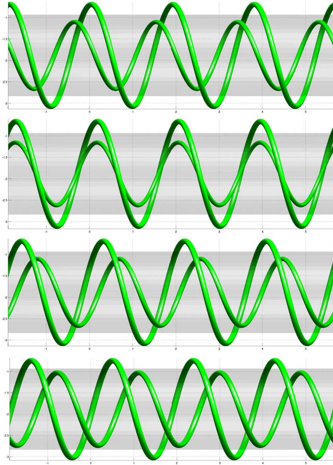
Figure 10.3 –  $Re = 10^4$ . Time evolution of  $N = 2$  helical vortices of reduced pitch  $L = 0.3$  with initial core size  $a = 0.06$  perturbed with the helical pairing mode. The vortices undergo a leapfrogs process. Isovalue of the helical vorticity  $\omega_B = \frac{1}{2}\omega_B^{max}$  at instants  $\tau = 6.8, 7.3, 7.8, 8.3$ . Time evolution goes from top to bottom. The grey region is the cylinder of radius  $R = 1$  around which the unperturbed helical vortices would coil.
