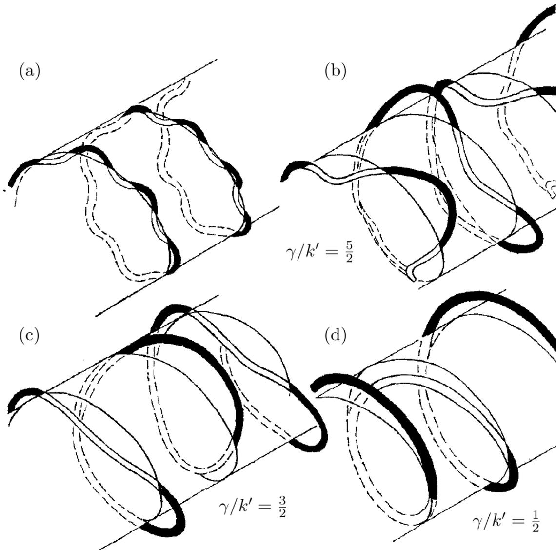
Figure 11.1 – General perturbation modes as sketched by [Widnall \(1972\)](#) for different values of the parameter  $\gamma/k'$ . Widnall makes a distinction between (a) short-wavelength modes, (b) and (c) intermediate wavelength or mutual induction modes and (d) long-wavelength modes. Taken from [Bolnot \(2012\)](#).
