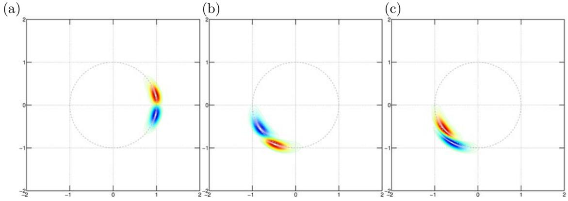
Figure 11.6 – Single helical vortex at  $L = 0.3$  and core size  $a = 0.09$ . Real part of the dominant eigenmode for (a)  $k = 0$  (helically symmetric perturbations), (b)  $k = 0.09$  and (c)  $k = 0.54$ .
