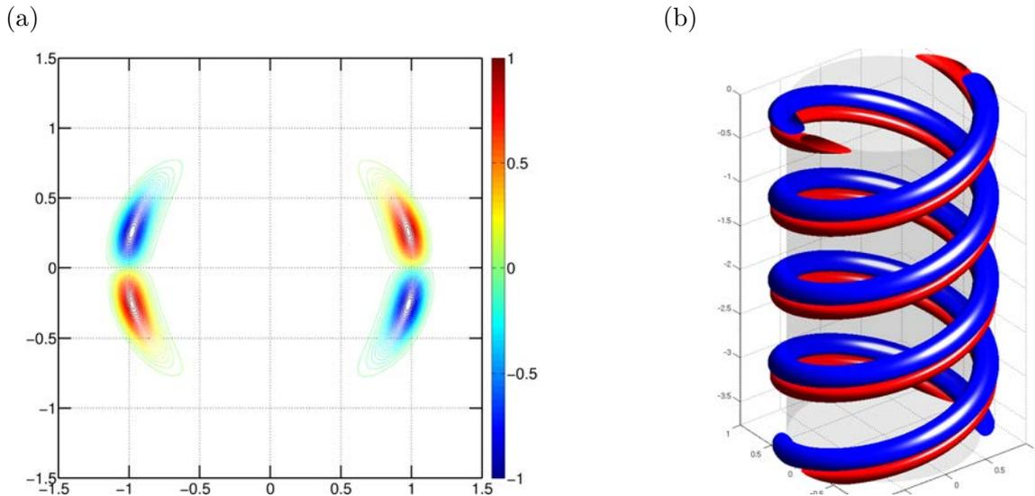
Figure 9.3 – Two helical vortices for  $L = 0.3, a = 0.09$  at  $Re = 10000$ . Structure of the neutral mode represented with a filled red circle in figure 9.2-a. (a) Contours of the real part of  $\hat{\omega}_B$  in  $\Pi_0$ . (b) Three-dimensional isosurface of vorticity corresponding to  $\pm \max \Re \{ \hat{\omega}_B \} / 4$  (red for positive isovalue and blue for the negative one).
