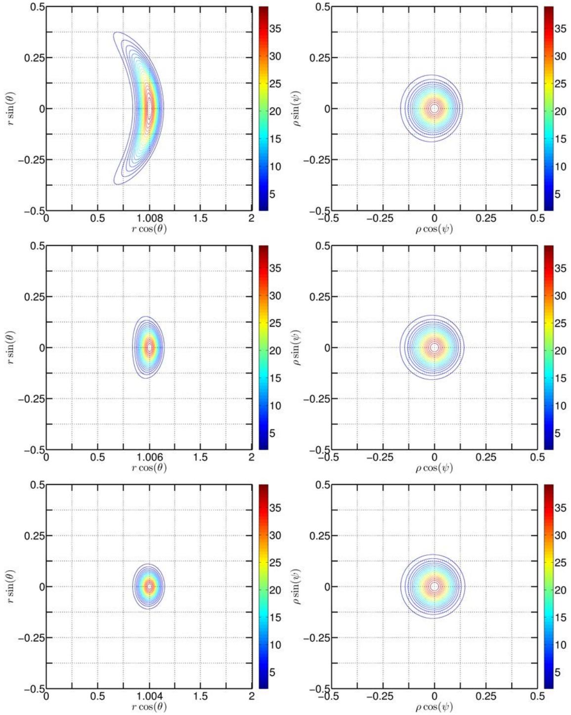
Figure 5.1 – Single vortex of core radius  $a = 0.09$ . Top: reduced pitch  $L = 0.20$ , middle:  $L = 0.60$  and bottom:  $L = 1$ . Left column: contours of vorticity  $\omega_B$  in the  $\Pi_0$  plane. Right column: contours of vorticity  $\omega_B$  in the  $\Pi_\perp$  plane.
