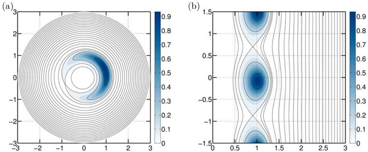
Figure 6.10 – One helical vortex of reduced pitch  $L = 0.25$  for  $Re = 5000$  at  $\tau = 92.5$ . (a) Isocontours of the stream function in the rotating frame  $\Psi_R$  (black lines) superimposed on top of the quantity  $\alpha\omega_B$ . (b) Representation in the meridian  $r - z$  plane (two coils are represented).
