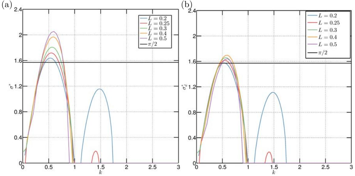
Figure 11.2 – Single helical vortex of core size  $a = 0.06$  at  $Re = 5000$ . Normalized growth rates as a function of  $k$  for various values of the reduced pitch  $L$ : (a)  $\sigma^*$  and (b)  $\sigma_d^*$ .
