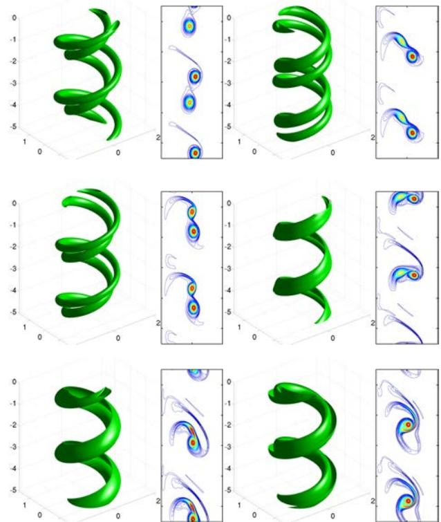
FIGURE 10 – Isovalue of the vorticity component  $\omega_B = 4$  of two helical vortices of pitch  $L = 0.3$  and core size  $a_b = 0.06$  represented at different instants. Time evolution goes from left to right and top to bottom.
