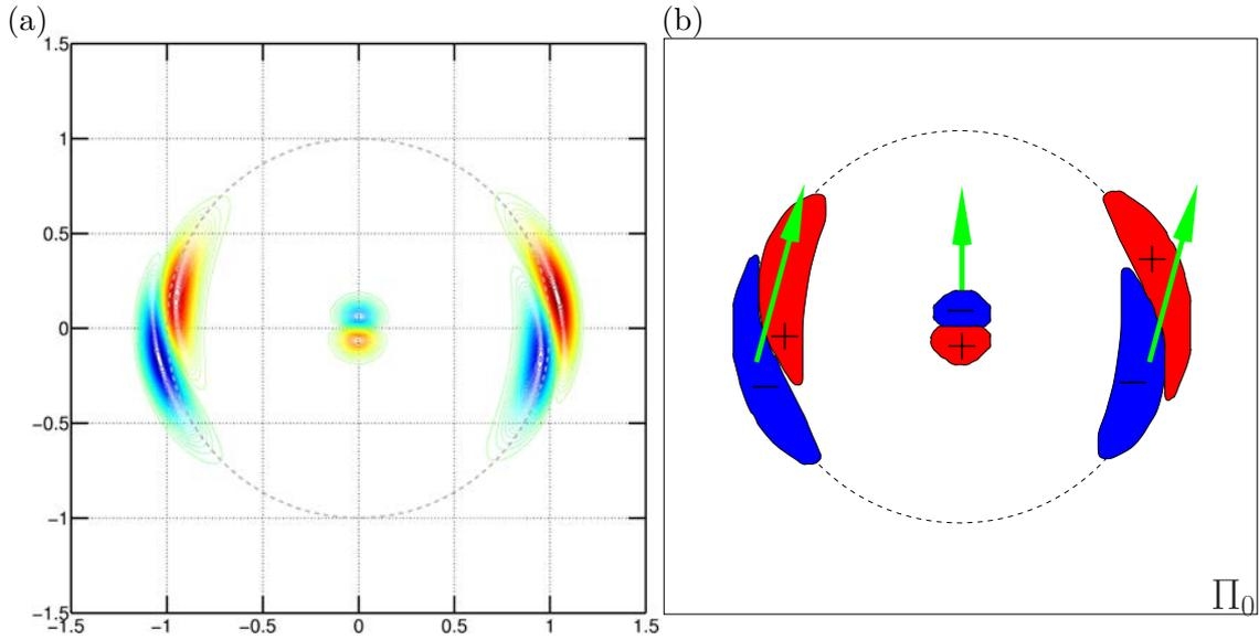
Figure 9.9 – The most unstable mode for the base flow corresponding to two helical vortices with  $L = 0.3$ , core size  $a = 0.09$  and a central hub vortex of core size  $a$ . Reynolds number for perturbations is  $Re = 10000$ . (a) Contours of  $\Re\{\hat{\omega}_B\}$  in  $\Pi_0$ . (b) Schematic representation: the displacement induced by the unstable mode when superimposed on the base flow are represented with the green arrows.
