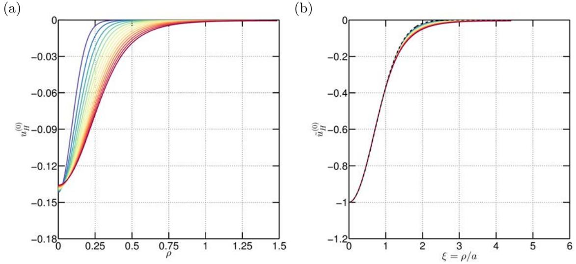
Figure 6.8 – One helical vortex of reduced pitch  $L = 0.5$  at  $Re = 5000$ . (a) Axisymmetric part of the helical jet  $u_H^{(0)}(\rho)$  at instants  $\tau = 22.5 : 10 : 172.5$  (time increases from left to right). (b) Scaled profiles of the axisymmetric part of the helical jet as a function of the similarity variable  $\xi$  (6.26) for the same instants.
