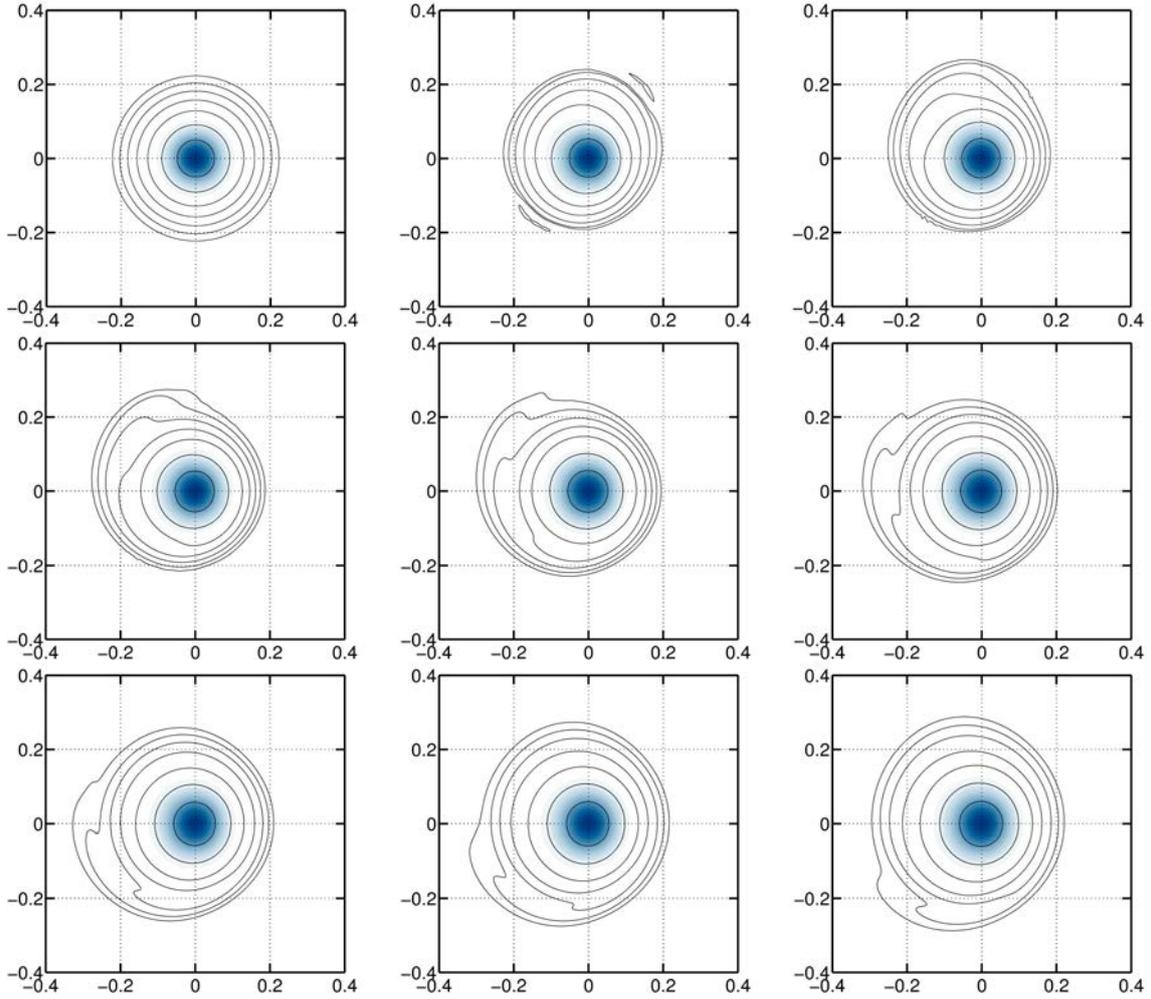
Figure 6.3 – One vortex of reduced pitch  $L = 0.25$  and initial core size  $a = 0.06$  at  $Re = 5000$ . Vorticity contours in the  $\Pi_{\perp}$  plane during the relaxation process. From left to right, top to bottom  $t\Gamma / (2\pi a_0^2) = 0, 10, \dots, 80$ . Contours levels are  $\omega_{B_A} / \omega_{B_A}^{(0)}(0) = 0.5, 0.1, 0.01, 0.001, 10^{-4}, 10^{-5}, 10^{-6}$ .
