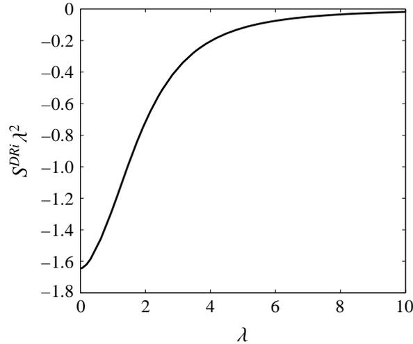
FIGURE 7. Strain rate parameter  $S^{DRi}$  generated by distant rings in an array of rings as a function of the aspect ratio  $\lambda = L_z/R$ .
