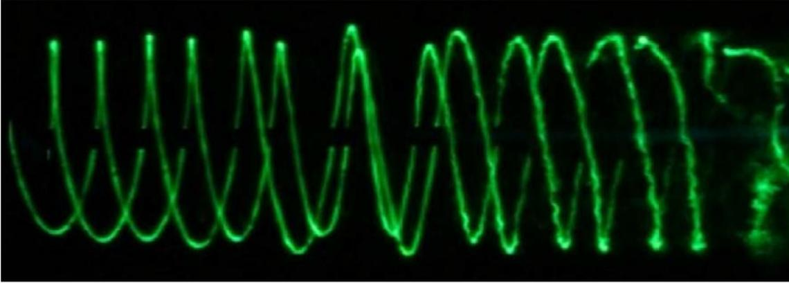
Figure 10.2 – Spatial evolution of  $N = 2$  helical vortices generated by a two-bladed rotor in a water channel. The vortex system is perturbed with one blade being radially offset. Such perturbation can be understood in a context where the helical symmetry is preserved. (Bolnot, 2012).
