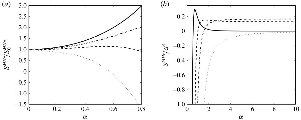
FIGURE 10. Strain rate parameter  $S^{MHe}$  versus  $\alpha = L/R$  for  $N$  helices with  $N = 1, 2, 3, 5$  (solid, dash, dash-dot, dotted lines) for  $\varepsilon = 1$ . (a)  $S^{MHe}$  is normalized by its expression at the origin  $S_0^{MHe} = -N^2/(24\alpha^2)$ ; (b)  $S^{MHe}$  is normalized by  $\alpha^4$ .
