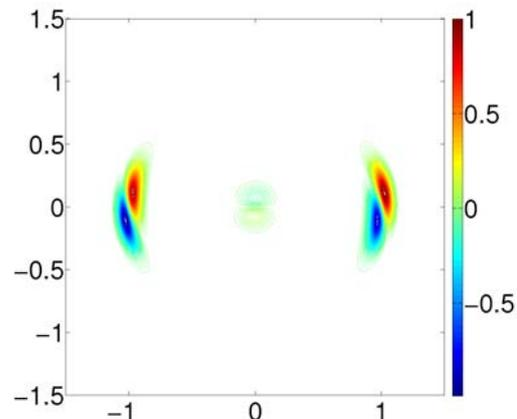
FIGURE 8 – Most unstable mode for the case of two vortices with  $L = 0.3$  and a central hub vortex of core size  $2a_b$ . The resulting instability mode can be described as a displacement mode for both helical vortices and the hub vortex as well.
