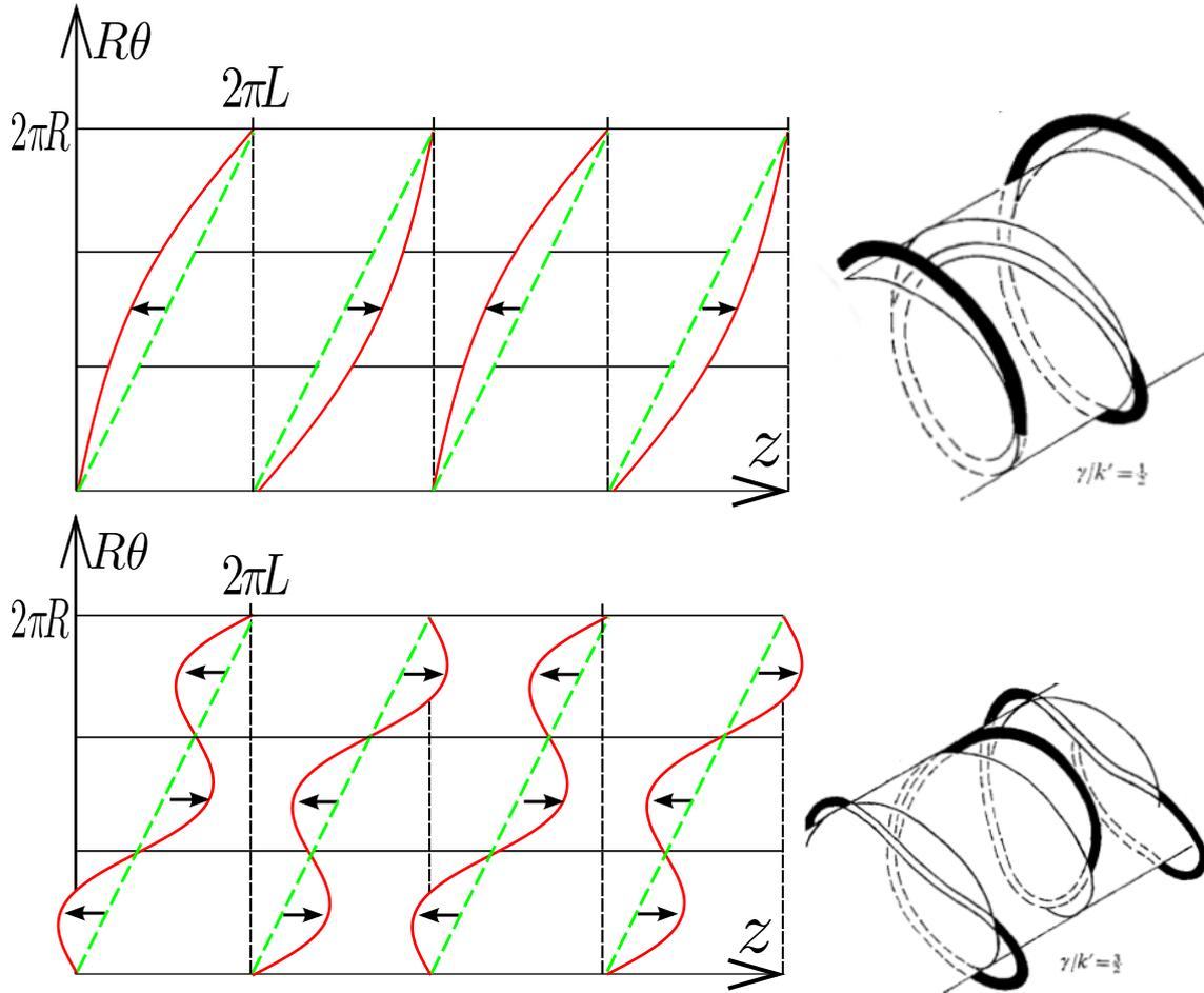
Figure 11.4 – Structure of the displacement modes. Left: sketch of the mode with the helix unwrapped in the  $R\theta - z$  plane. Right: original figure of the mode from [Widnall \(1972\)](#). Top: mode  $k = 1/2$ . Bottom:  $k = 3/2$ .
