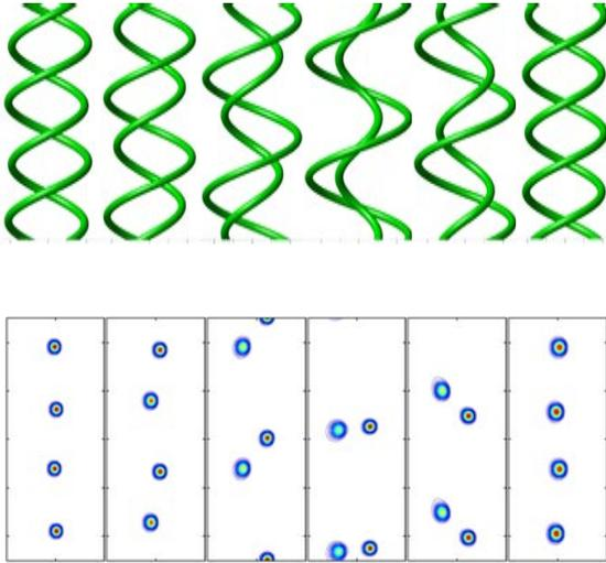
FIGURE 9 – The vortices undergo a leapfrogging process. Time evolution goes from left to right. Top figures : Isovalue of the vorticity component  $\omega_B = 10$  represented at different instants for two helical vortices of pitch  $L = 0.3$  and core size  $a_b = 0.06$ . Bottom figures : vorticity component  $\omega_B$  in the  $(r, z)$ -plane.
