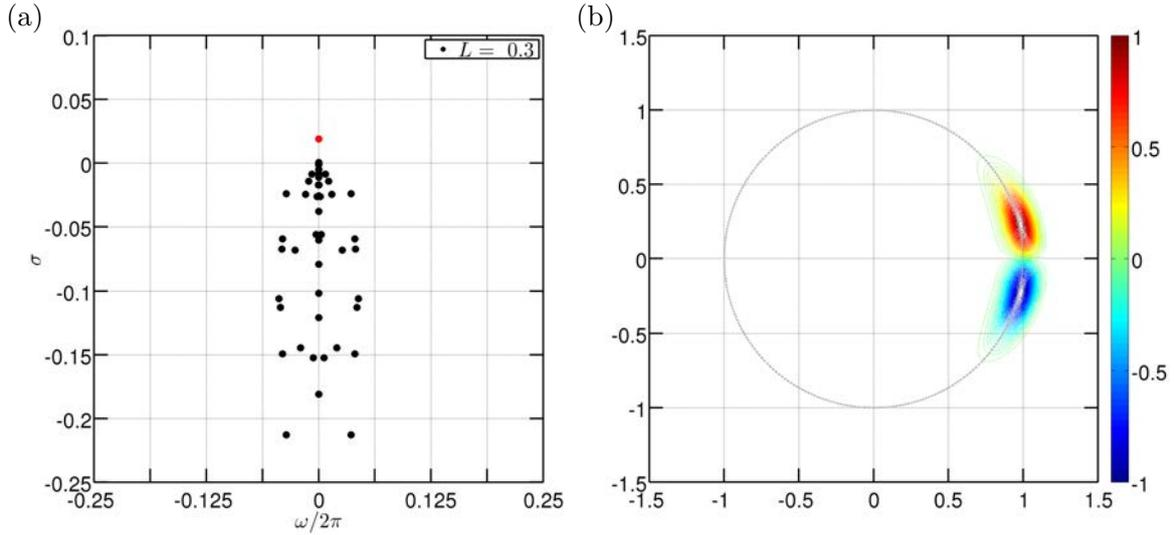
Figure 9.1 – (a) Spectrum in the  $(\sigma, \omega/2\pi)$  plane for a single helical vortex with reduced pitch  $L = 0.3$  and core size  $a = 0.09$  at  $Re = 10000$ . The 50 dominant eigenvalues are displayed. (b) Mode structure of the mode represented with a red dot in graph (a): contours of the real part of  $\hat{\omega}_B$  in  $\Pi_0$ . The associated imaginary part is zero.
