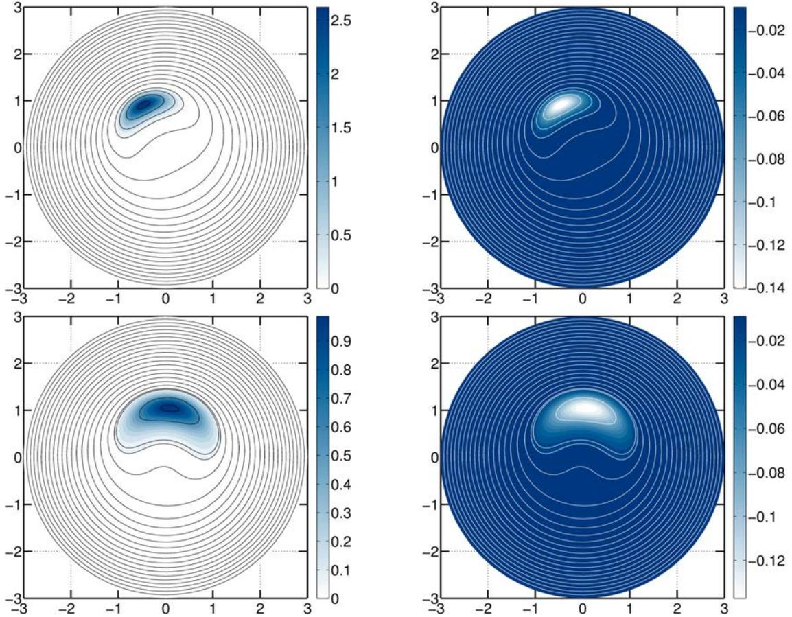
Figure 6.4 – One helical vortex of reduced pitch  $L = 0.5$  at  $Re = 5000$ . Left column: isocontours of the stream function in the rotating frame  $\psi_R$  (black lines) superimposed on top of the quantity  $\alpha\omega_B$  with  $\omega_B$  being the helical vorticity. Right column: same isocontours of  $\Psi_R$  (white lines) superimposed on top of the helical velocity (jet)  $u_H$ . The chosen instants are  $\tau = 62.5$  (top) and  $\tau = 162.5$  (bottom).
