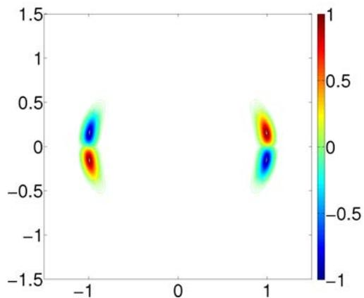
FIGURE 7 – Neutral mode which exists due to the invariance of the base flow with respect to the azimuth. This mode only rotates the base flow in the clockwise direction.
