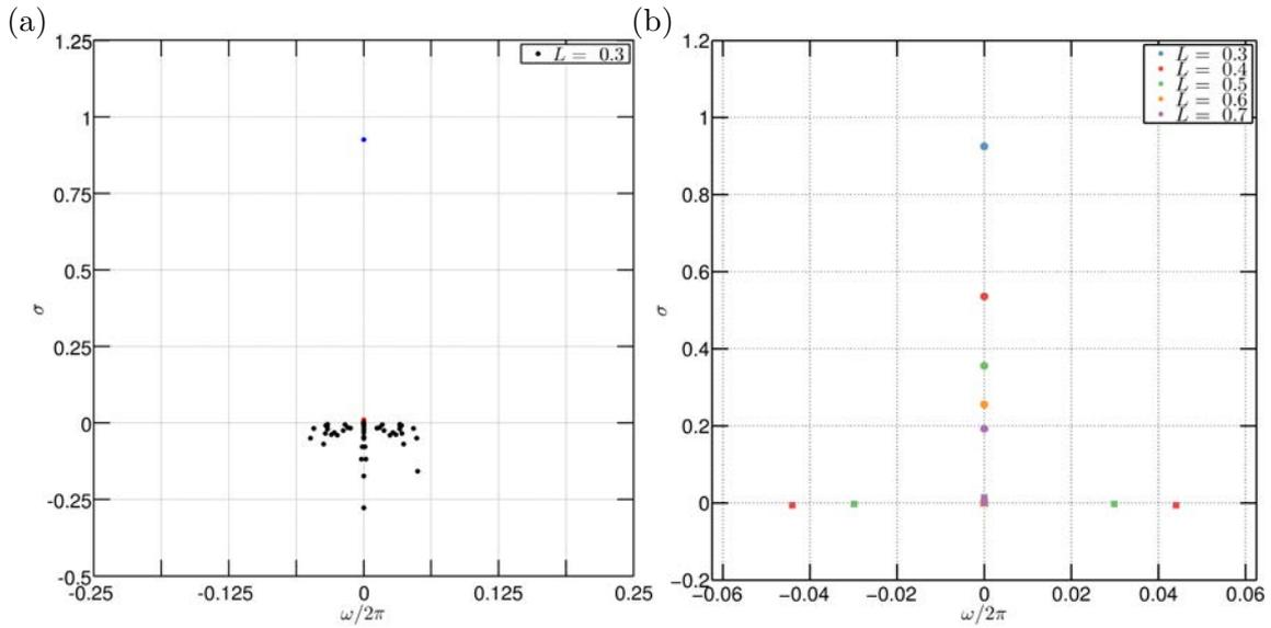
Figure 9.2 – (a) Spectrum in the  $(\sigma, \omega/2\pi)$  plane for two helical vortices with  $L = 0.3$  and  $a = 0.09$  at  $Re = 10000$ . The first 50 eigenvalues are displayed. The dominant eigenmode is represented in red and the neutral one in blue. (b) Spectrum showing the first four dominant eigenvalues for various  $L$  at  $Re = 10000$ . The dominant mode is represented in filled circles.
