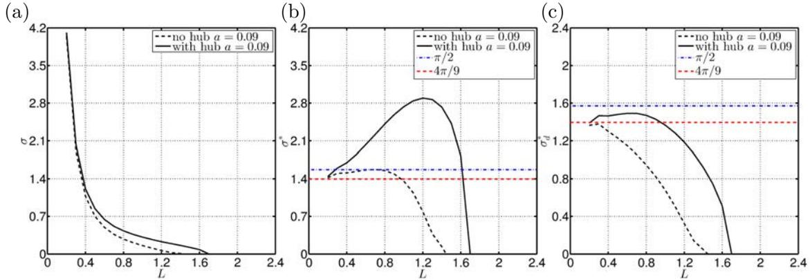
Figure 9.12 – Growth rate of the dominant instability mode for  $N = 3$  helical vortices with the vortex hub (solid line) and without (dashed line) for  $a_{hub} = a = 0.09$  at  $Re = 10000$  as a function of pitch  $L$ . (a) Growth rate  $\sigma$ . (b) Normalized growth rate  $\sigma^*$ . (c) Normalized growth rate  $\sigma_d^*$ .
