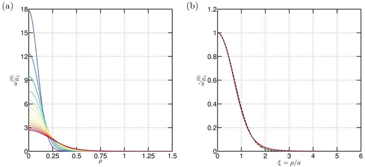
Figure 6.7 – One helical vortex of reduced pitch  $L = 0.5$  at  $Re = 5000$ . (a) Axisymmetric part of  $\omega_{B_A}^{(0)}(\rho)$  at instants  $\tau = 22.5, 32.5, \dots, 172.5$  (time increases from top to bottom). (b) Scaled profiles of the axisymmetric part of the helical vorticity as a function of the similarity variable  $\xi$  (6.26) for the same instants.
