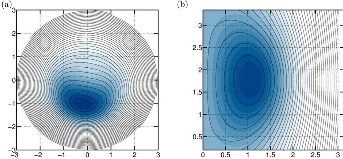
Figure 6.11 – One helical vortex of reduced pitch  $L = 1$  for  $Re = 5000$  at  $\tau = 1750$ . (a) Isocontours of the stream function in the rotating frame  $\Psi_R$  (black lines) superimposed on top of the quantity  $\alpha\omega_B$ . (b) Representation in the meridian  $r - z$  plane.
