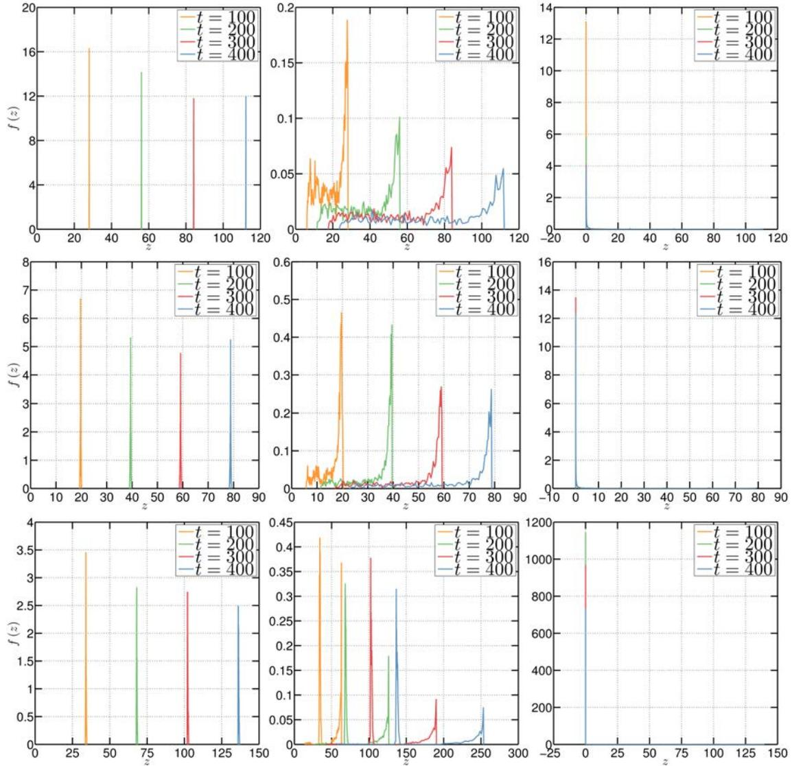
Figure 6.19 – Passive particles ( $St = 0$ ): time evolution of the probability density functions of the axial position  $z$  at  $t = 100$  (orange),  $t = 200$  (green),  $t = 300$  (red) and  $t = 400$  (blue). First row: case 1; second row: case 2; bottom row: case 3. The  $N_p$  particles are initially set at  $z = 0$  in the vortex core (left column), or in the inner region (central column) or in the outer region (right column).
