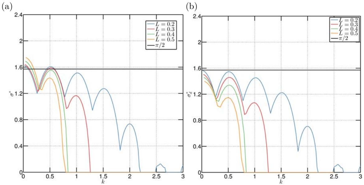
Figure 11.7 –  $N = 2$  helical vortices of core size  $a = 0.06$  at  $Re = 5000$ . Normalised growth rates as a function of  $k$  for various values of reduced pitch  $L$ : (a)  $\sigma^*$  and (b)  $\sigma_d^*$ .
