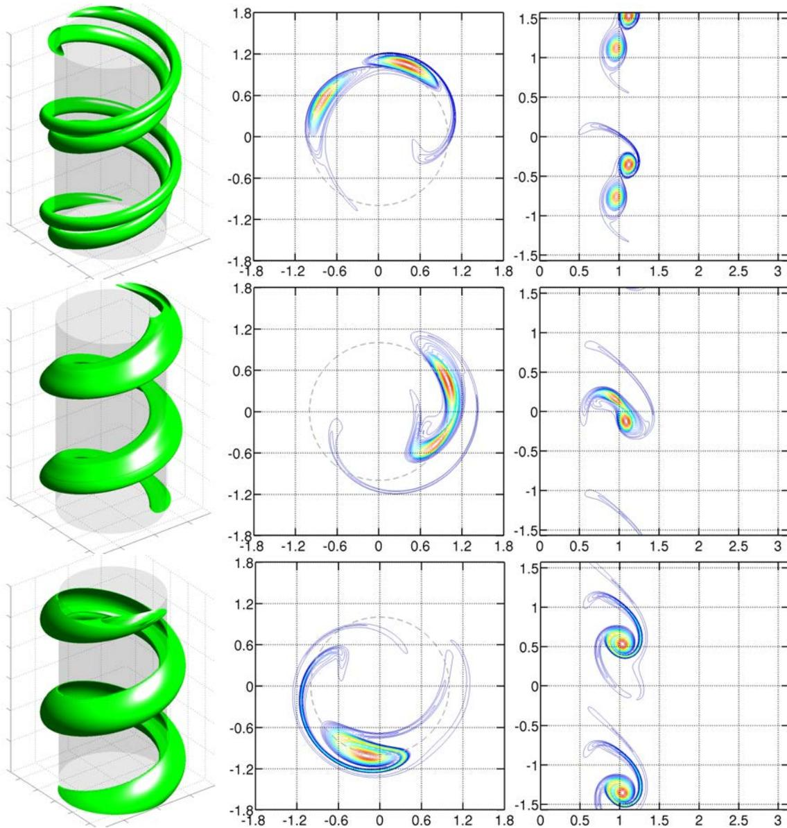
Figure 10.8 –  $N = 2$  helical vortices of pitch  $L = 0.3$  and core size  $a = 0.06$  perturbed initially with the helical pairing mode at  $Re = 10000$ . Left column: isovalue of the vorticity component  $\omega_B = \omega_B^{max}/4$ . Central column: contours of the helical vorticity  $\omega_B$  in plane  $\Pi_0$ . Right column: contours of the helical vorticity  $\omega_B$  in the median  $r - z$  plane. The chosen instants are  $\tau = 24, 25, 26$  (top to bottom).
