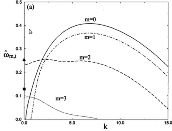
Figure 8.7 – Temporal growth rate as a function of the axial wavenumber  $k$  for  $\beta = 4$  and various values of  $m = 0, \dots, 3$ , at  $Re = 667$ . From (Gallaire and Chomaz, 2003)
