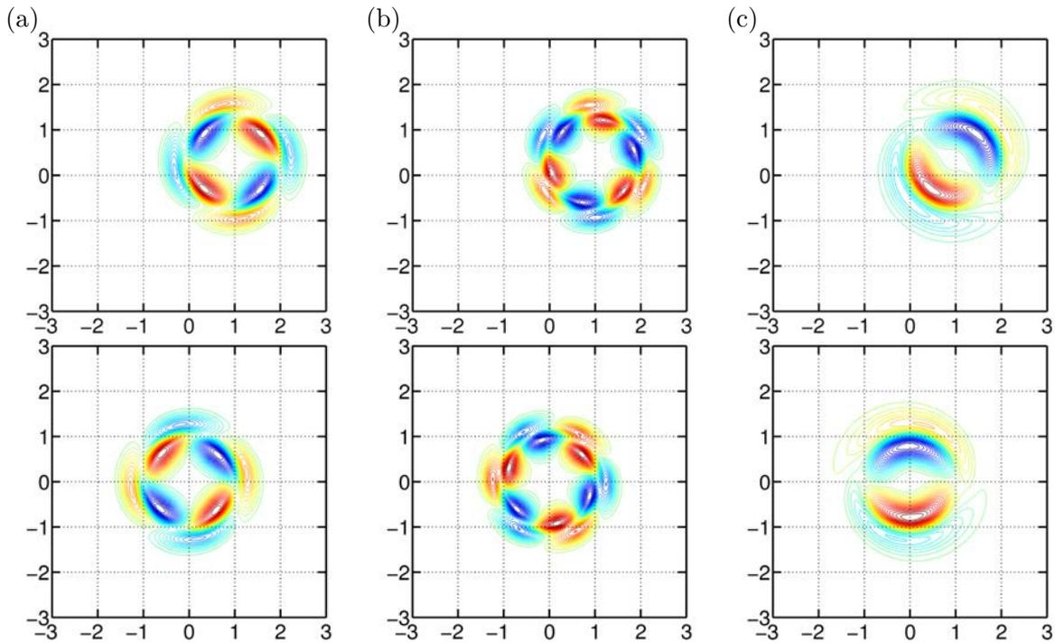
Figure 8.8 – Carton and McWilliams vortex: structure of the modes, obtained with the Arnoldi algorithm, at  $Re = 667$ . First row: (a) Unstable mode ( $m = 2, k = 0$ ). (b) Unstable mode ( $m = 3, k = 0$ ). (c) Unstable mode mode ( $m = 1, k = 0$ ). Second row: modes obtained when the base flow is off-centred from the axis.
