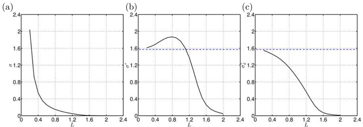
Figure 9.5 – Growth rate of the dominant instability mode for  $N = 2$  helical vortices for  $a = 0.09$  at  $Re = 10000$  as a function of pitch  $L$ . (a) Growth rate  $\sigma$ . (b) Normalized growth rate  $\sigma^*$  as defined in (9.4). (c) Normalized growth rate  $\sigma_d^*$  as defined in equation (9.6). In figures (b) and (c) the horizontal dashed line is located at the value  $\pi/2$ .
