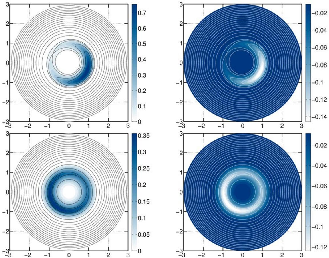
Figure 6.23 – One helical vortex of reduced pitch  $L = 0.25$  and  $Re = 5000$ . Snapshots at  $\tau = 112.5$  (top) and  $\tau = 202.5$  (bottom). Left column: contours of the stream function in the rotating frame  $\Psi_R$  (black lines) superimposed on top of the quantity  $\alpha\omega_B$ . Right column: same streamlines (white lines) superimposed on top of the quantity  $u_H$ .
