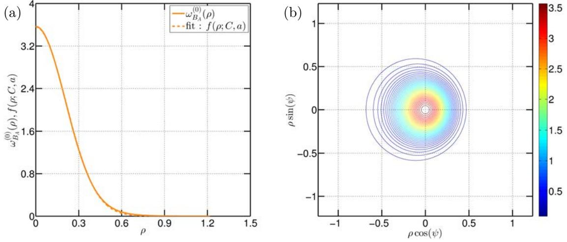
Figure 5.4 – A single vortex of reduced pitch  $L = 1$ . (a) Plot of the axisymmetric part of the helical vorticity  $\omega_{BA}^{(0)}(\rho)$  fitted with a Gaussian function  $f(\rho; C, a)$ . (b) Iso-contours of  $\omega_{BA}(\rho, \psi)$  on the  $\Pi_{\perp}$  plane.
