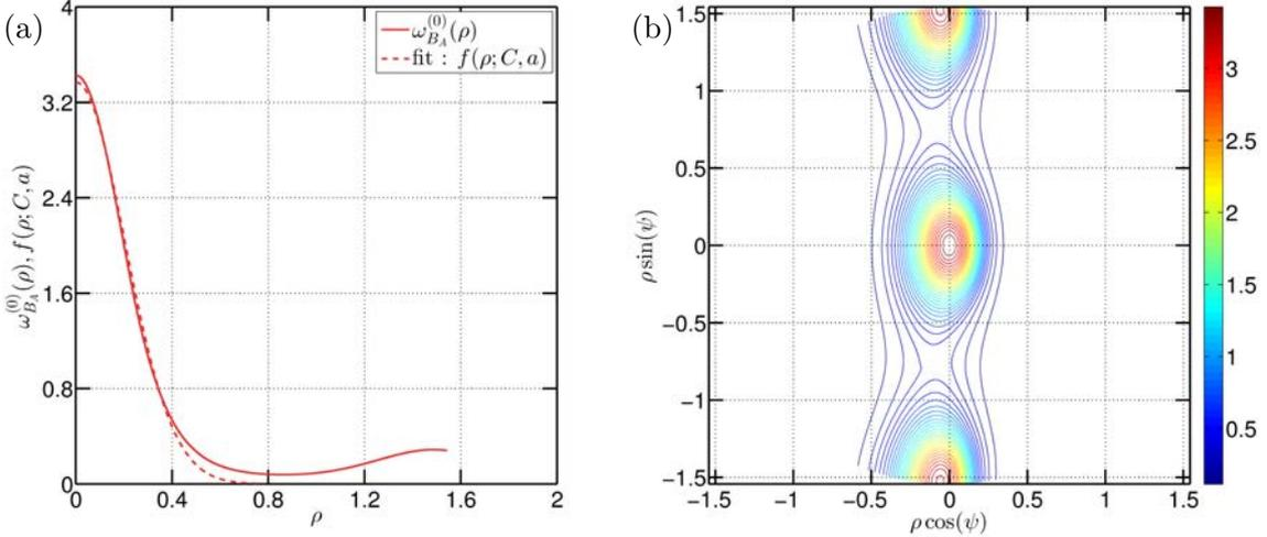
Figure 5.5 – One vortex of reduced pitch  $L = 0.25$ . (a) Plot of the axisymmetric part of the helical vorticity  $\omega_{BA}^{(0)}(\rho)$  and the fit function. (b) Iso-contours of  $\omega_{BA}(\rho, \psi)$  on the  $\Pi_{\perp}$  plane.
