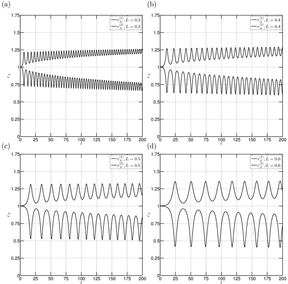
Figure 10.7 – Overtaking motion of  $N = 2$  inviscid vortex filaments obtained with the cut-off theory: radial position as a function of time. The initial positions are obtained from the DNS. The core size is fixed at  $a = 0.06$  in all figures. (a)  $L = 0.3$ , (b)  $L = 0.4$ , (c)  $L = 0.5$ , (d)  $L = 0.6$ .
