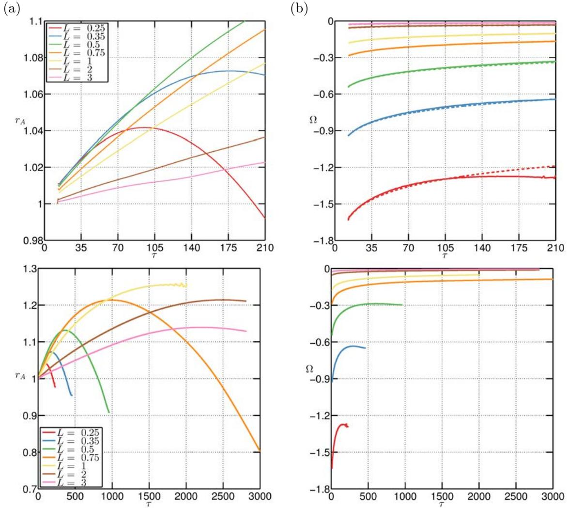
Figure 6.9 – One helical vortex at  $Re = 5000$ . (a) Time evolution of the helix radii  $r_A$ , for different values of  $L$ . (b) Time evolution of the angular velocity  $\Omega$  for the same range of parameters. The dotted lines are the predicted values by the cutoff theory coupled to a 2D diffusion law for the vortex core size.
