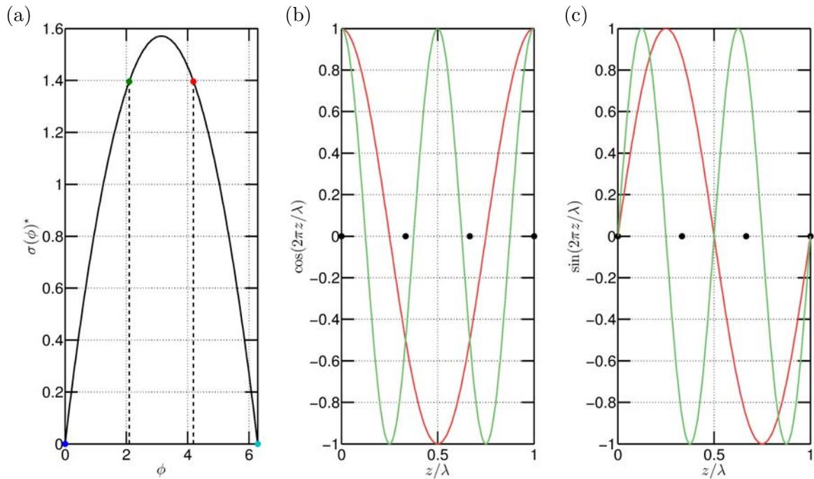
Figure 9.14 – Analogy with an array of point vortices for  $N = 3$  separated by  $h = 2\pi L/3$ : (a) Dispersion relation, the full dots correspond to the modes pertinent for  $N = 3$ . (b) Real part of the induced displacement by the unstable mode  $\phi = 2\pi/3$  (red curve) and  $4\pi/3$  (green curve). (c) Imaginary part.
