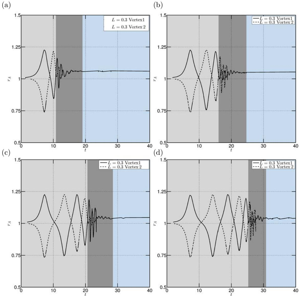
Figure 10.5 – Influence of the Reynolds number on the leapfrog mechanism of two helical vortices of pitch  $L = 0.3$  with core size  $a = 0.06$ . (a)  $Re = 2500$ . (b)  $Re = 5000$ . (c)  $Re = 7500$  and (d)  $Re = 10000$ . In all figures, the evolution of  $r_A$  is shown as a function of time. The grey region indicates the time interval when the leapfrogs occur, the dark grey represents the merging phase and the clear blue region indicates the merged state.
