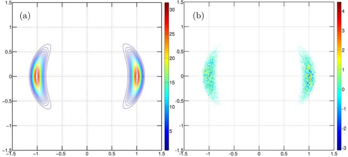
Figure 8.1 – Stability analysis of  $N = 2$  helical vortices of reduced pitch  $L = 0.3$  with core size  $a_b = 0.09$ . (a) Frozen base flow : contours of the helical vorticity component  $\omega_B$  in the  $\Pi_0$  plane. Note that the  $x$  and  $y$  are chosen such that vortex centres are aligned at  $y = 0$ . (b) Initial helical vorticity perturbations  $\omega'_B$  in  $\Pi_0$ .
