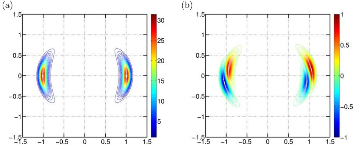
Figure 10.1 – (a) Base flow: Two helical vortices  $L = 0.3$  with core size  $a = 0.1$ . Component  $\omega_B^{Base}$  (b) Real part of the eigemode  $\hat{\omega}_B$  of the helical pairing mode. These two fields will be combined and set as initial condition for the non linear computation.
