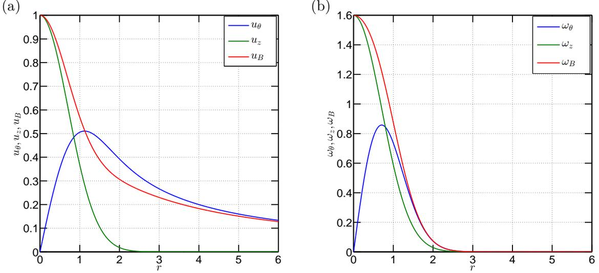
Figure 8.4 – Batchelor vortex for swirl parameter  $q = 0.8$  in the helical framework with  $L = 1.76$ . (a) The azimuthal  $u_\theta$  and axial  $u_z$  components are combined to yield the helical velocity component  $u_B$  (equation (8.37)). (b) The Azimuthal  $\omega_\theta$  and axial  $\omega_z$  vorticity components are combined to yield the helical vorticity  $\omega_B$  (equation by (8.38)).
