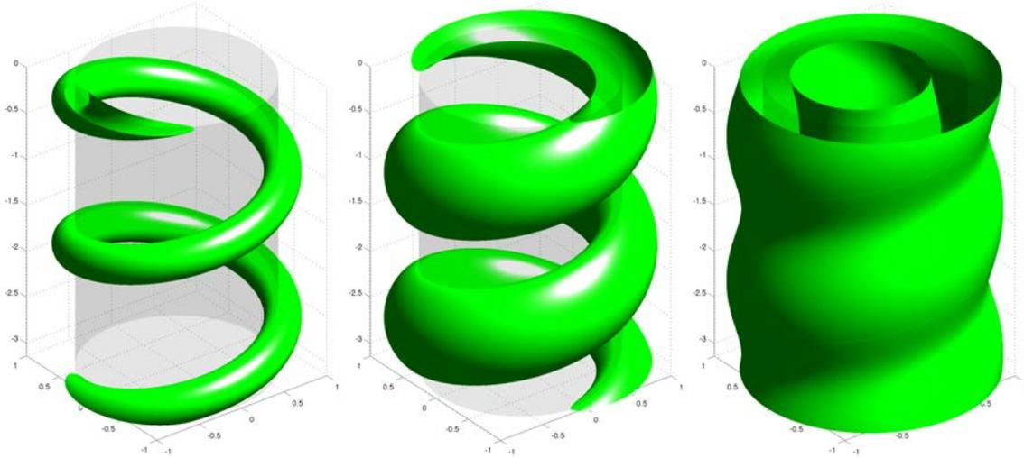
Figure 6.21 – One helical vortex of reduced pitch  $L = 0.25$  and  $Re = 5000$ . Isosurfaces of  $\alpha\omega_B$  at instants  $\tau = 22.5, 92.5, 142.5$ . The chosen isosurface value is  $\alpha\omega_B(\tau) = 0.15 \max(\alpha\omega_B)$ .
