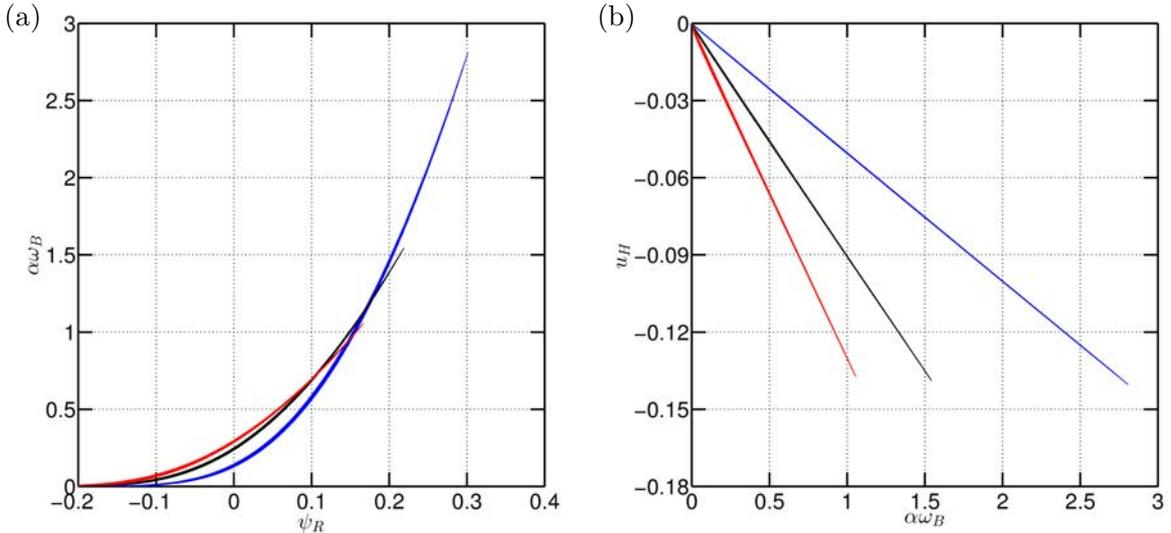
Figure 6.5 – One helical vortex of reduced pitch  $L = 0.5$  at  $Re = 5000$ . Scatter plots of the quantities  $(\alpha\omega_B, \Psi_R)$  and  $(u_H, \alpha\omega_B)$  at instants  $\tau = 62.5$  (blue),  $112.5$  (black),  $162.5$  (red). During the diffusing stage, all the (vorticity, streamfunction) points on (a) and (velocity, vorticity) points on (b) are aligned in a single curve for a given time  $\tau$ , illustrating the functional relationship between these quantities.
