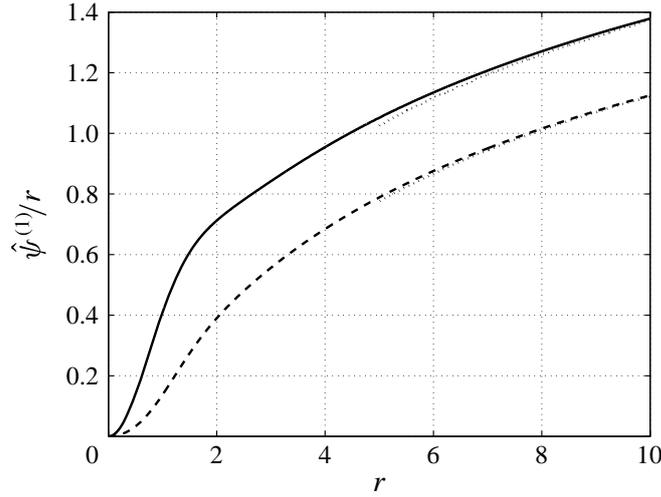
FIGURE 4. Characteristics of the dipolar correction for the Batchelor vortex.  $\hat{\psi}^{(1)}/r$  versus  $r$  (solid line:  $W_0 = 0$ ; dashed line:  $W_0 = 1$ .  $W_{00} = 0$  for both cases) The dotted lines correspond to the asymptotic behaviour (3.11).
