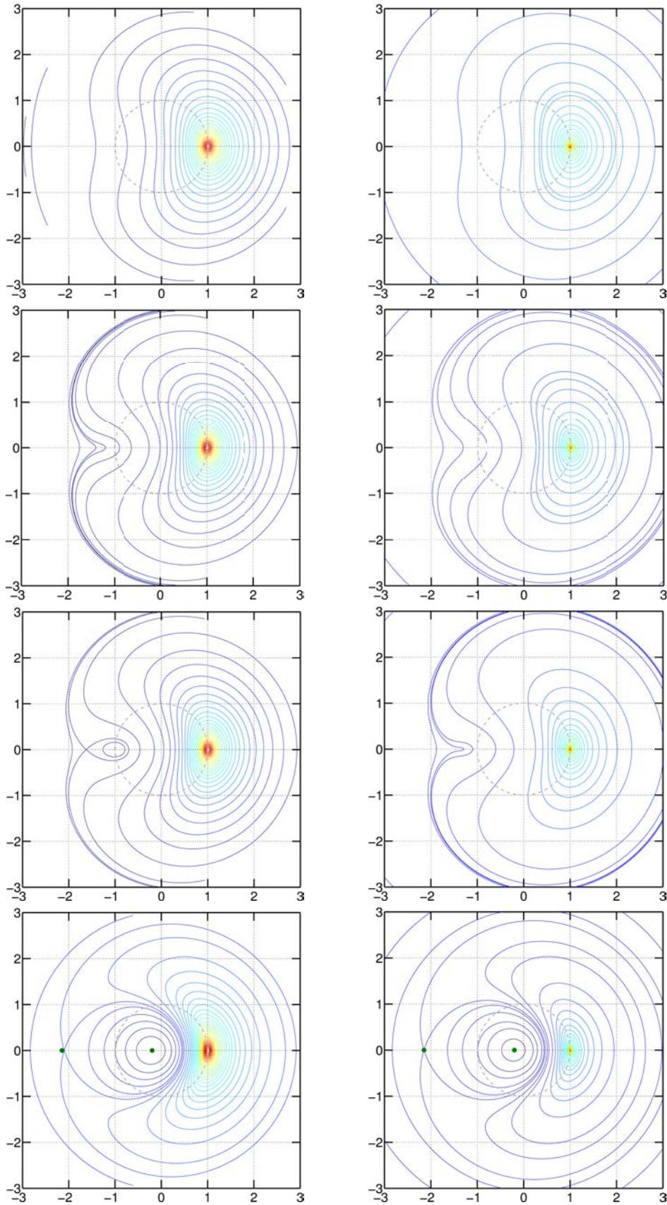
Figure 6.13 – Streamline topology in the laboratory frame for a helical vortex of reduced pitch  $L = 1$  (top),  $L = 0.815$  (second row),  $L = 0.791$  (third row) and  $L = 0.5$  (bottom). Left: Contours of  $\Psi$  from the DNS for a vortex with finite core size  $a = 0.06$ . Right: contours of  $\Psi_H$  from analytical formula (6.30). On both bottom graphs, the green dots correspond to the critical points of  $\Psi_H$ .
