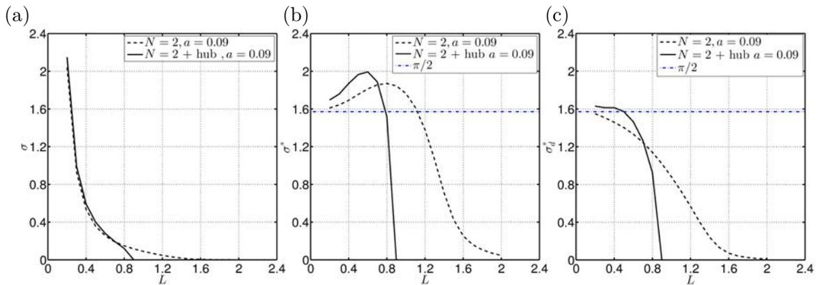
Figure 9.10 – Growth rate of the dominant instability mode for  $N = 2$  helical vortices with the vortex hub (solid line) and without (dashed line) for  $a_{hub} = a = 0.09$  at  $Re = 10000$  as a function of pitch  $L$ . (a) Growth rate  $\sigma$ . (b) Normalized growth rate  $\sigma^*$ . (c) Normalized growth rate  $\sigma_d^*$ . In (b) and (c) the horizontal line represents  $\pi/2$ .
