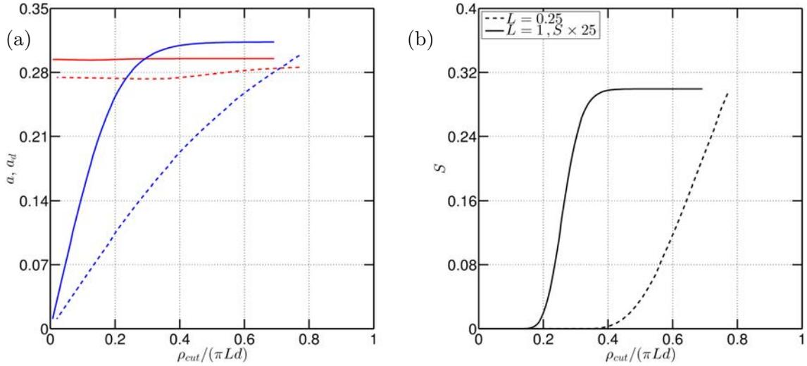
Figure 5.6 – One helical vortex for  $L = 1$  (solid) and  $L = 0.25$  (dashed). (a) Core sizes  $a$  (red) and  $a_d$  (blue) as a function of  $\rho_{cut}/(\pi L d)$  (see definition of  $d$  in equation (5.33)). (b) Error  $S$  (equation (5.35)) as a function of  $\rho_{cut}/(\pi L d)$ . Note that for  $L = 1$ , the error  $S$  is multiplied by a factor of 25.
