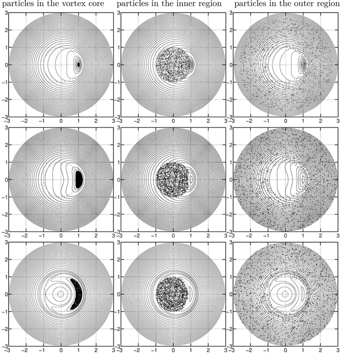
Figure 6.16 – Particle initialisations in the  $\Pi_0$  plane on top of the streamlines in the rotating frame. Particles are set in the vortex core (left column), in the inner region (central column) and in the outer region (right column). Top row: case 1, middle row: case 2 and bottom row: case 3.
