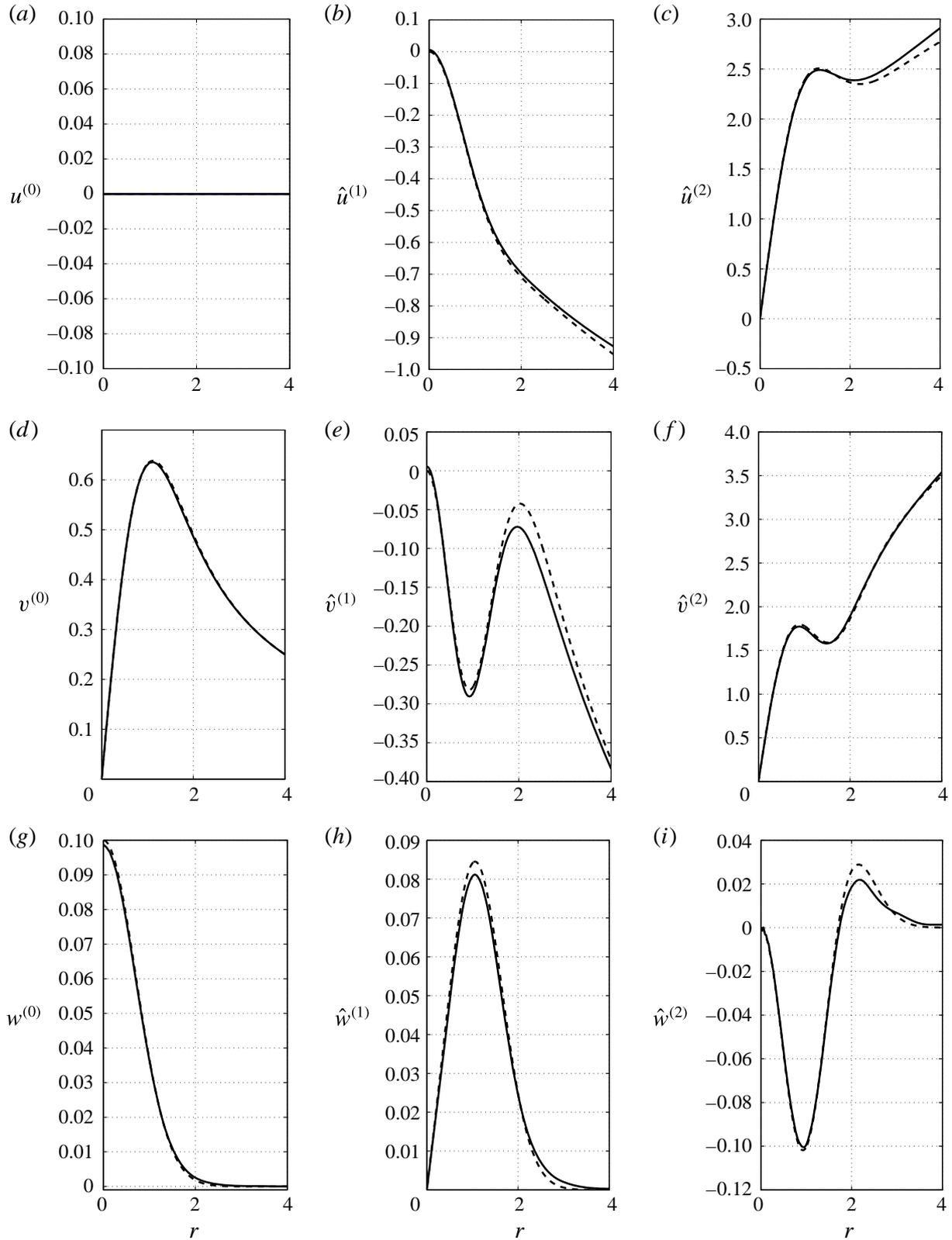
FIGURE 11. Array of swirling vortex rings with jet strength  $W_0 = 0.1$ , at  $L_z/R = 3$ ,  $\varepsilon = 0.11$ ,  $Re = 2000$ : comparison between asymptotic results (dashed lines) and DNS results (solid lines). (a,d,g) Monopolar component; (b,e,h): dipolar component; (c,f,i) quadrupolar component. (a–c) Radial velocity, (d–f) azimuthal velocity, (g–i) axial velocity.
