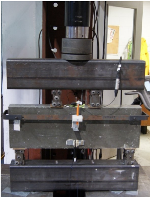
Figure 4.1 : Pre-cracking test apparatus
