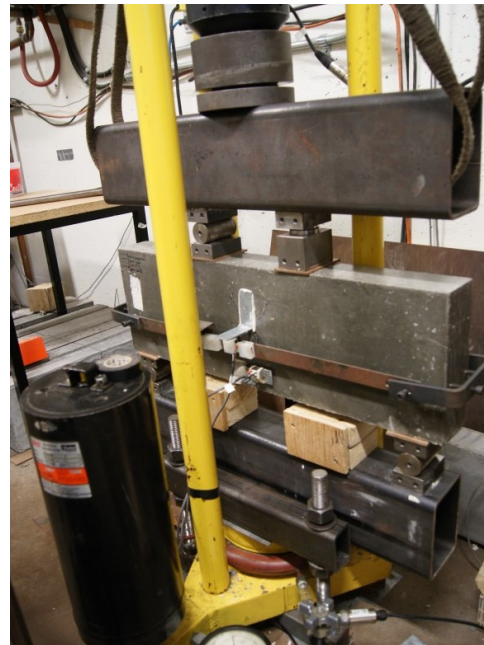
Figure 4.2 : Sustained loading test apparatus
