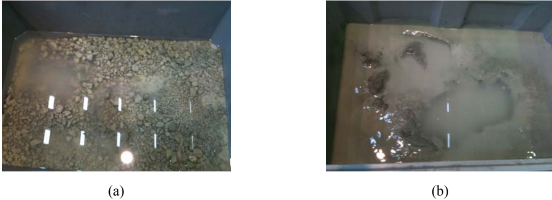
Figure 29 Difference of softness after 2 weeks of (a) illitic rock and (b) montmorillonitic rock immersed in water
