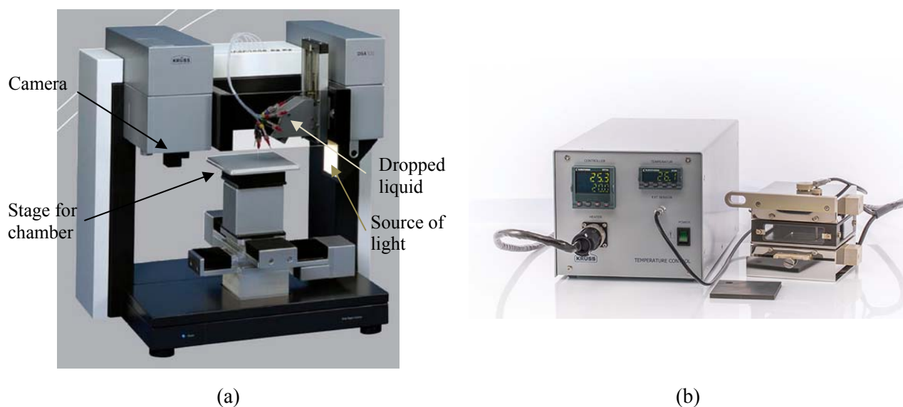
Figure 33 (a) Drop Shape Analyser DSA100 coupled with the (b) Kruss tempering chamber for high temperatures (TC21)
