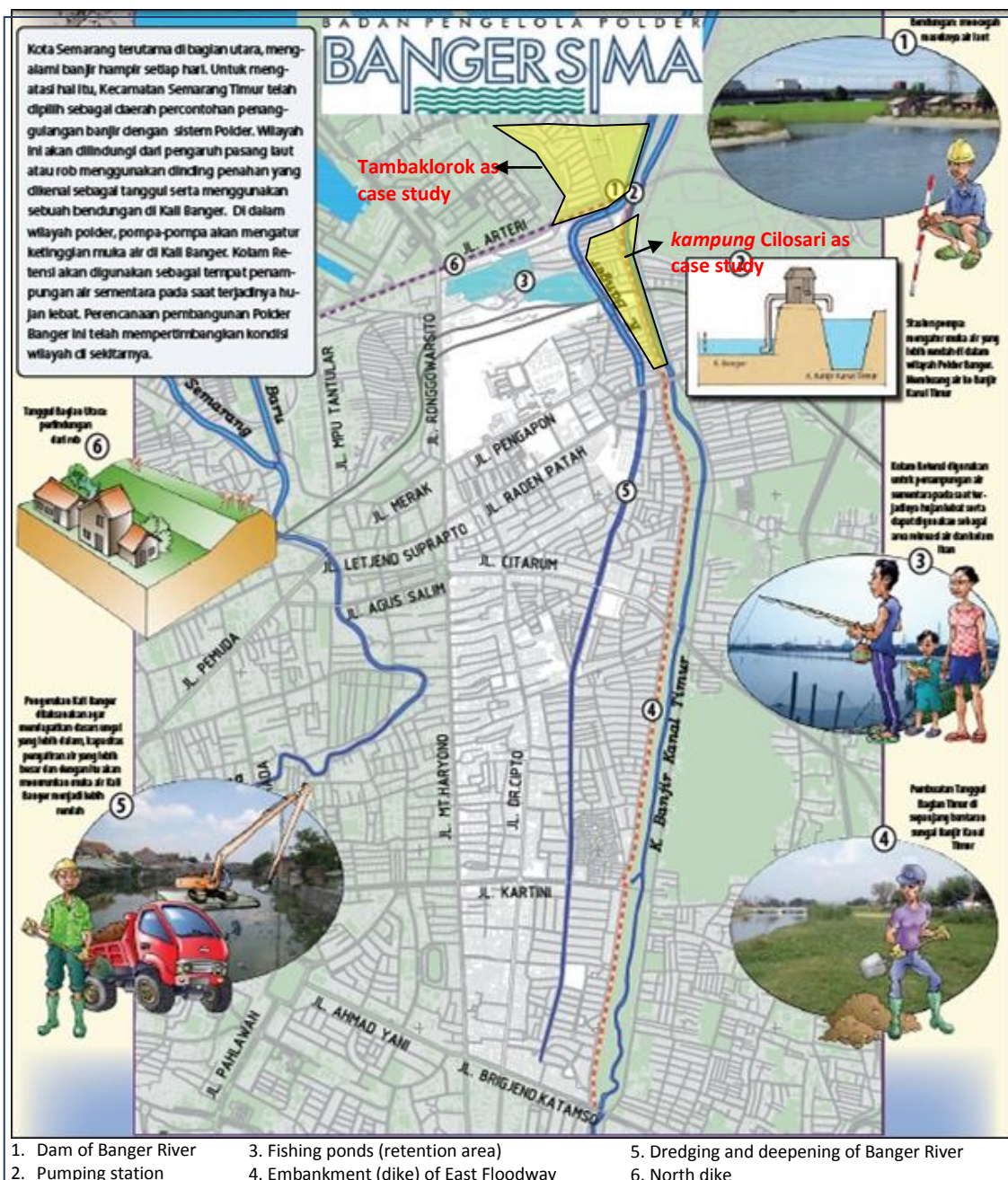
Figure 68. Design of Banger Polder Pilot Project
