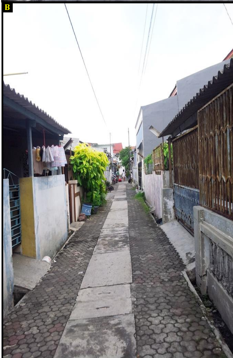
Figure B: Most of the houses have solid fences around, although the fences' conditions are diverse because of the economic resources and the desires of each household. However, most of the households have similar aims. They build fences to reduce the inundation impact in their houses. Furthermore, most of the house entrances are higher than the local road.
