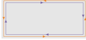
Figure 1.9: Edge states of a Kane-Mele insulator. In a Kane-Mele insulator (also called QSHE state), there are two counter-propagating helical edge states which form a Kramers pair on each interface. As a consequence, backscattering from an edge state to its counter-propagating partner is not allowed.
